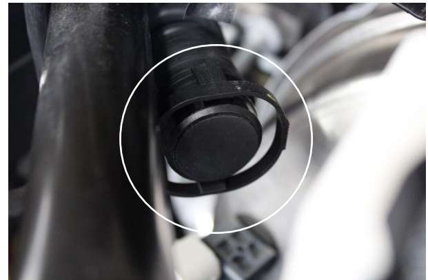
Fig. 7-k: Install Rubber Plug & Secure Vacuum Line To Sound Tube
