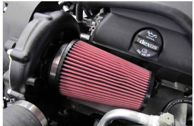
Fig. 8-e: Attach Air Filter To Supercharger Unit
