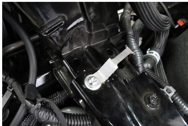
Fig. 5-b: Install Tube B Support Bracket & Button-Head Screw
