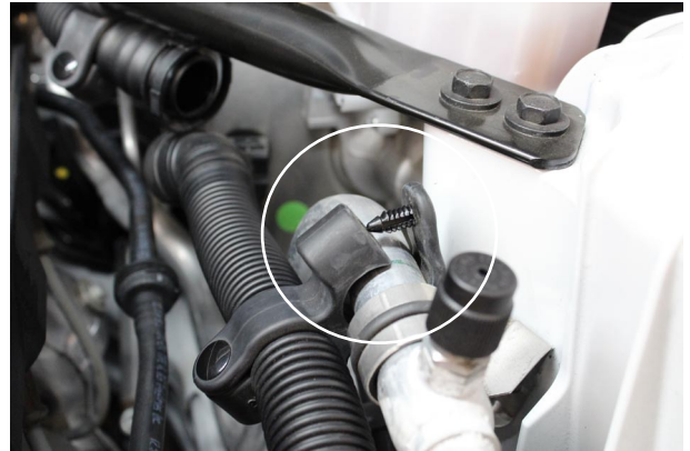
Fig. 1-ae: Unclip & Remove Sound Tube From Vehicle
