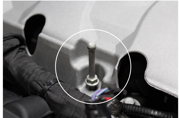
Fig. 7-d: Remove Engine Cover Fasteners
