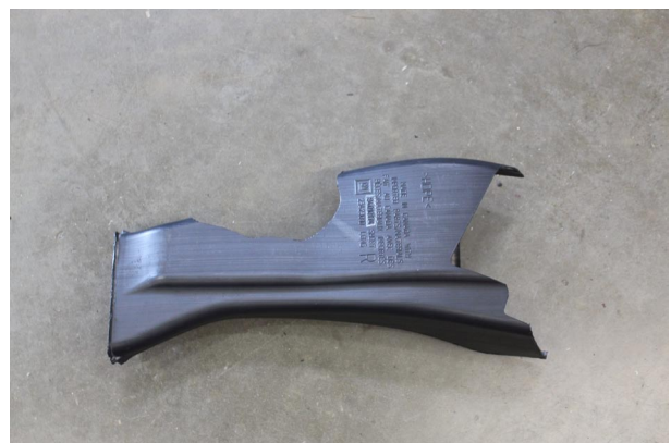
Fig. 6-c: Modified Brake Cooling Duct (Outer Section)
