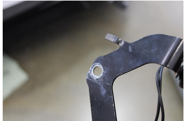
Fig. 9-b: Straighten Out Locating Tab
