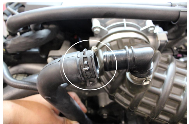
Fig. 1-aa: Remove Sound Tube From Air Inlet
