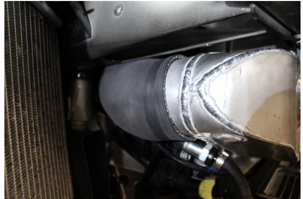
Fig. 3-s: Install Custom Silicone Discharge Sleeve To Charge Air Cooler
