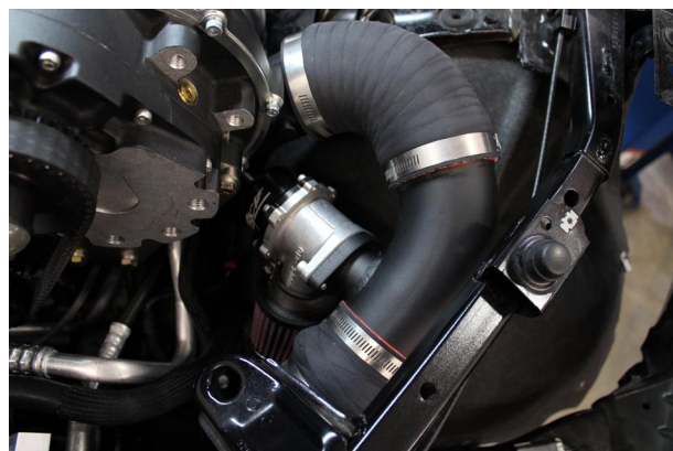
Fig. 5-f: Attach 90° Silicone Elbow & Discharge Tube "A"
