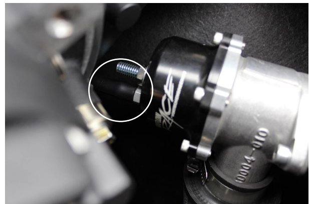
Fig. 7-l: Attach Vacuum Hose To Fitting
