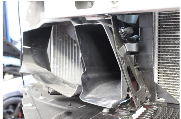
Fig. 1-m: Zoomed In - Remove Brake Duct Fastener
