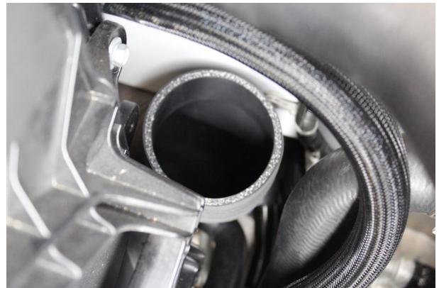
Fig. 3-t: Verify Fitment Of Custom Silicone Discharge Sleeve
