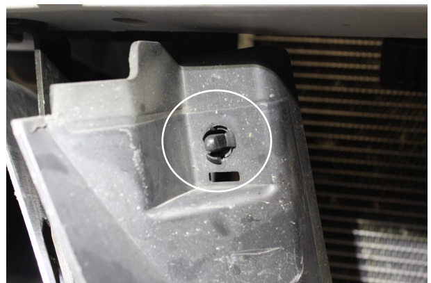
Fig. 1-l: Remove Ambient Air Temperature Sensor
