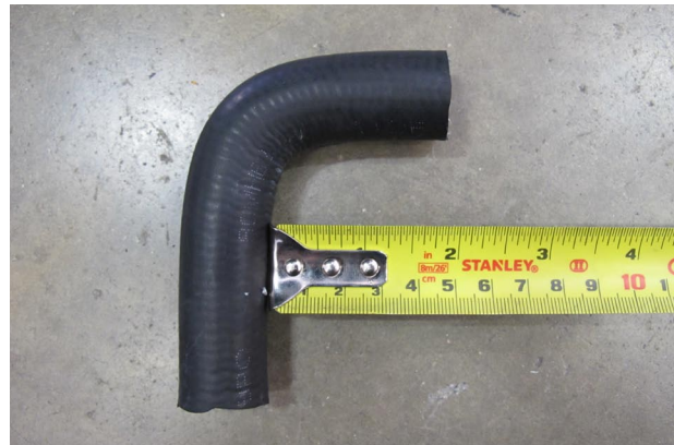
Fig. 3-h: Cut 2" From Inside Bend
