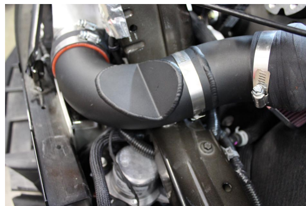
Fig. 5-c: Install Discharge Tube "B" As Shown
