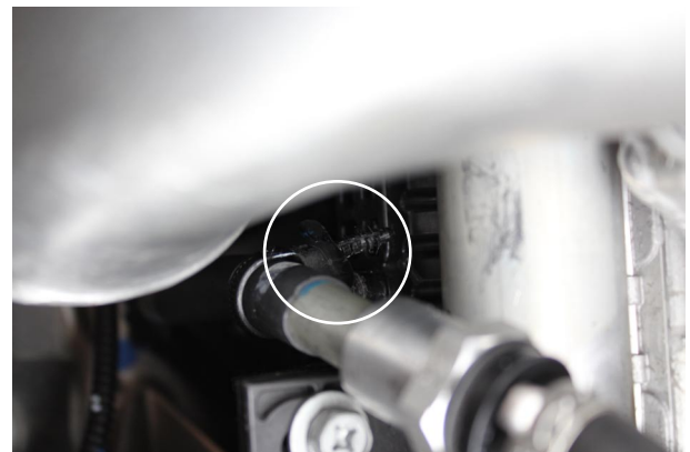
Fig. 2-f: Detach Trans. Cooler Line From Radiator
