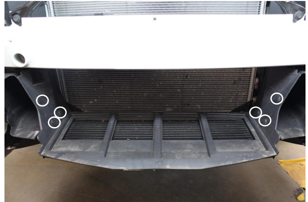
Fig. 1-j: Remove Shroud Fasteners
