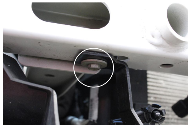
Fig. 6-f: Secure Transmission Cooler Mount
