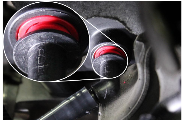
Fig. 7-h: Zoomed In - Remove 45° Fitting From Rear Of Intake Manifold
