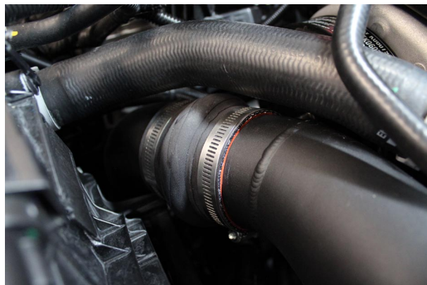
Fig. 5-h: Attach Discharge Tube "D" To Discharge Tube "C"
