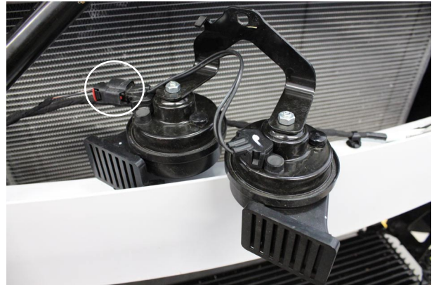
Fig. 1-s: Unplug Horn Assembly & Set Aside
