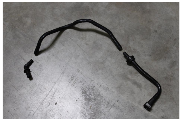
Fig. 7-i: Remove Fittings From Hard Plastic Vacuum Line
