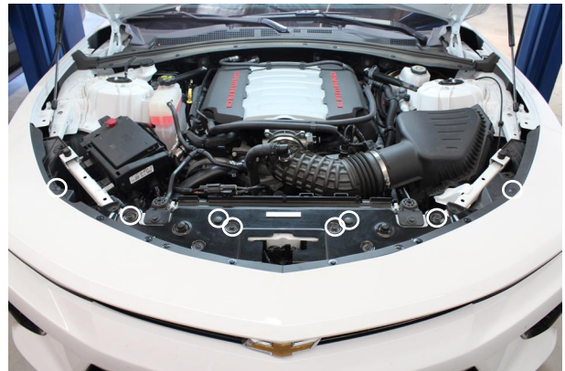
Fig. 1-e: Remove Front Bumper Fasteners
