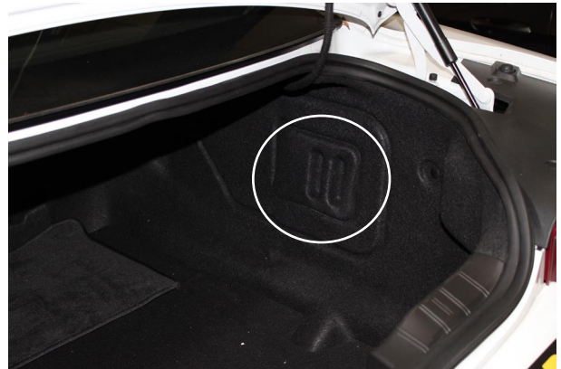
Fig. 1-a: Remove Battery Cover
