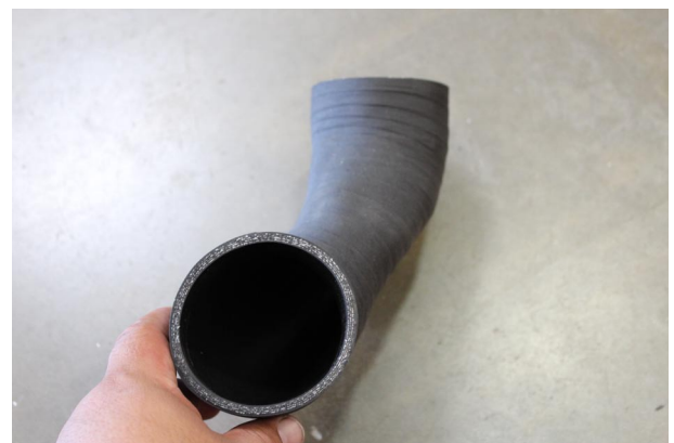
Fig. 3-r: Custom Silicone Discharge Sleeve
