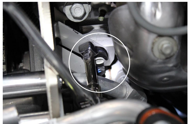
Fig. 4-l: Re-tighten A/C Mount Screw
