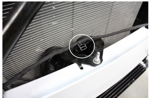
Fig. 1-r: Remove Horn Fastener
