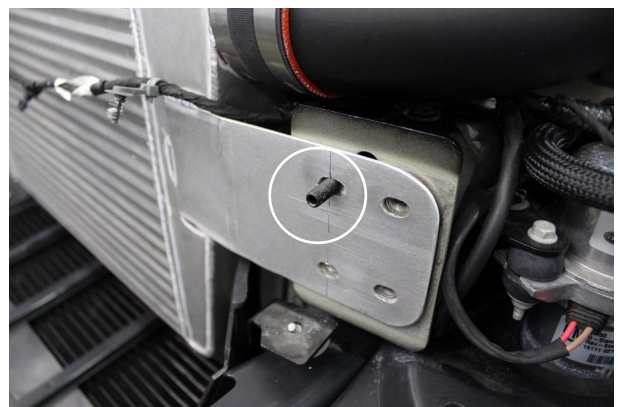
Fig. 3-o: Install Threaded Stud & Charge Air Cooler
