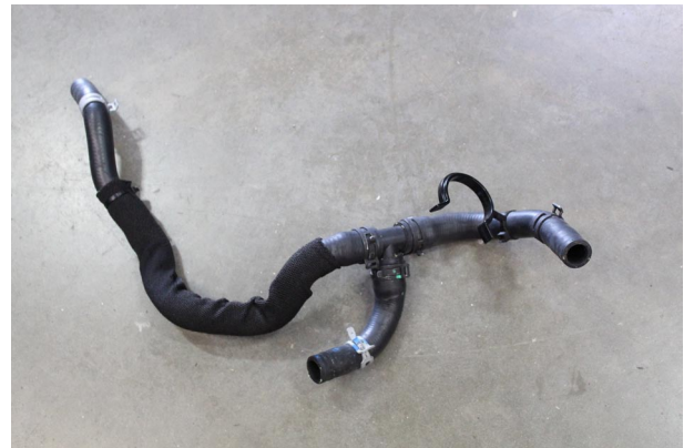
Fig. 3-e: Remove Coolant Hose Assembly
