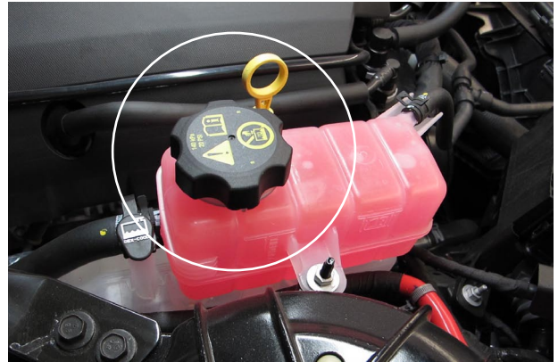
Fig. 3-ab: Fill Both Coolant Reservoirs
