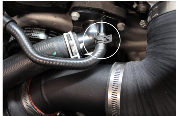
Fig. 3-z: Cut 1/2" From Small Diameter Coolant Hose
