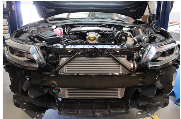
Fig. 9-e: Re-Install Headlights & Core Support Brackets
