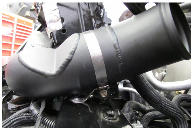
Fig. 5-d: Attach Hose Clamp To Tube B
