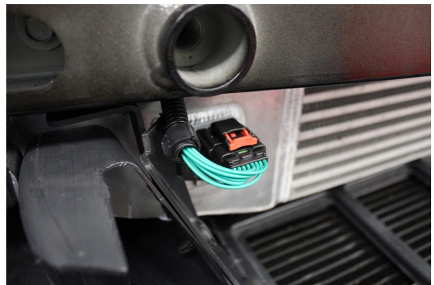
Fig. 6-i: Route MAF Harness Extension Towards Top Of Vehicle
