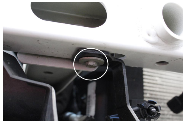
Fig. 1-n: Remove Trans Cooler Mount Screws
