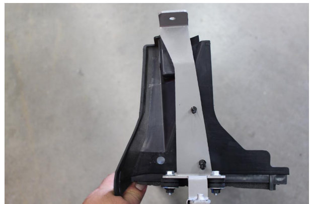
Fig. 2-c: Temporarily Mount New Trans. Cooler Bracket
