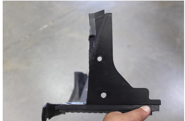
Fig. 2-d: Modify Trans. Cooler Shroud
