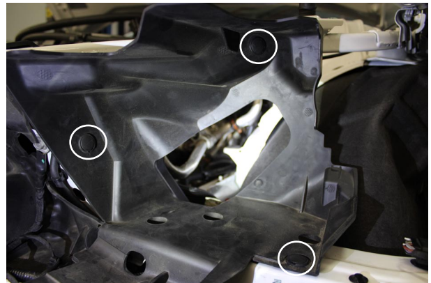
Fig. 1-t: Remove Plastic Fasteners
