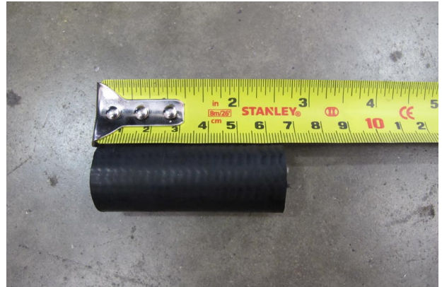
Fig. 3-j: Cut 2" Straight Section
