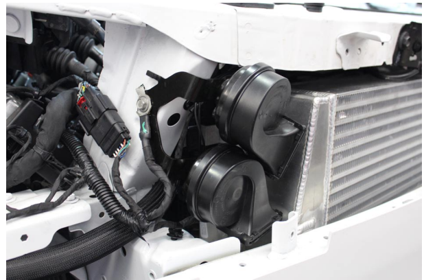
Fig. 9-d: Install Horn Assembly & Ground Strap
