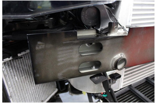
Fig. 3-p: Place Front Bumper Support Into Position
