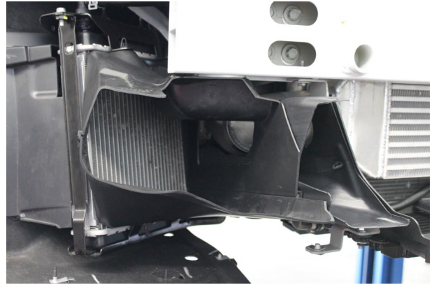
Fig. 6-d: Test Fit Cooling Ducts
