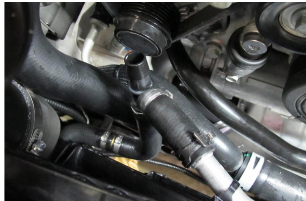
Fig. 3-n: Install Coolant Line Assembly
