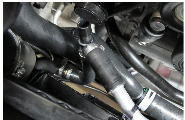
Fig. 3-l: Clock Coolant Line Assembly
