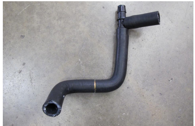
Fig. 3-k: Temporarily Assemble Coolant Lines
