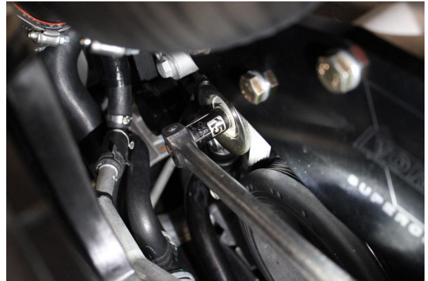
Fig. 4-m: Install Serpentine Drive Belt
