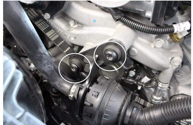
Fig. 1-ac: Remove Sound Tube Screws
