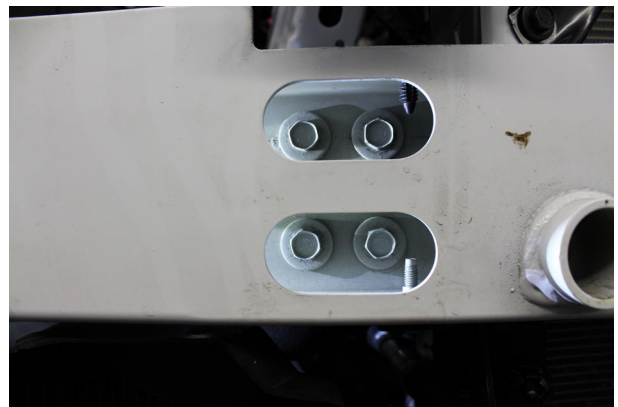
Fig. 1-u: Remove Front Bumper Beam Fasteners
