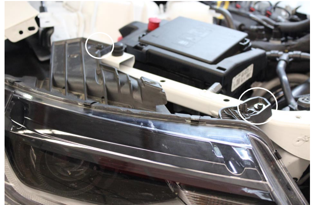
Fig. 1-g: Remove Headlight Fasteners
