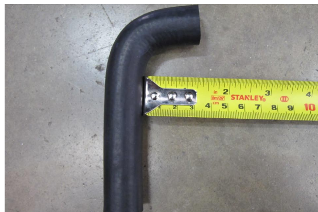
Fig. 3-i: Cut 1-1/2" From Inside Bend
