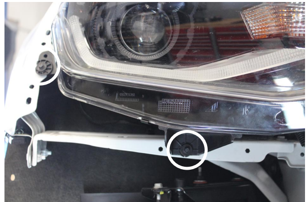
Fig. 1-h: Remove Headlight Fasteners
