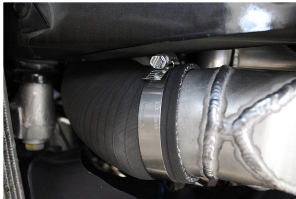
Fig. 5-g: Secure Custom Silicone Discharge Sleeve
