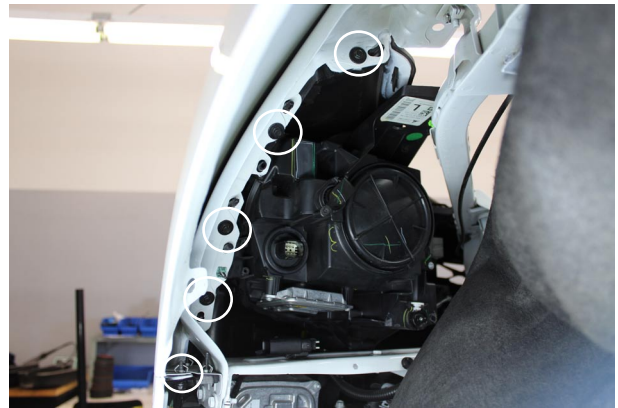
Fig. 1-d: Remove Front Bumper Fasteners
