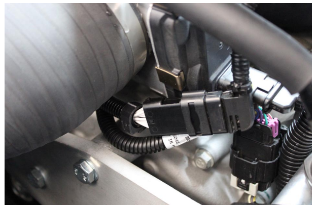
Fig. 6-l: Plug In MAF Extension Harness To MAF Sensor Connector
