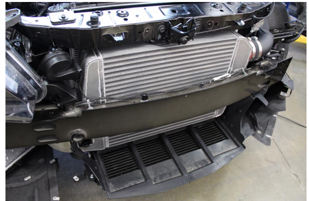
Fig. 3-q: Secure Front Bumper Support
