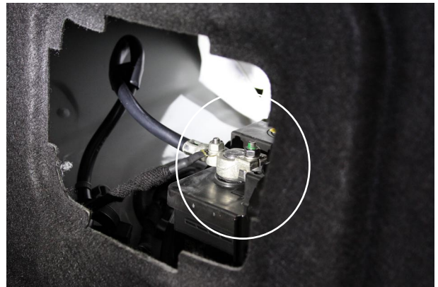
Fig. 1-b: Unplug Negative Battery Terminal
