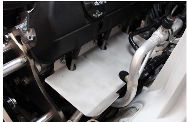
Fig. 8-b: Loosely Attach Heat Shield
