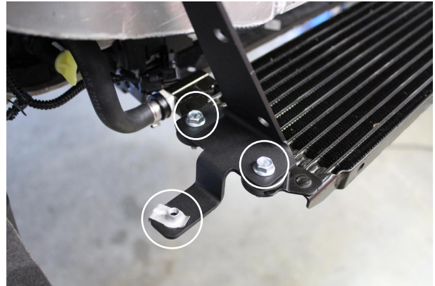
Fig. 2-g: Install P.Side Trans. Cooler Bracket
