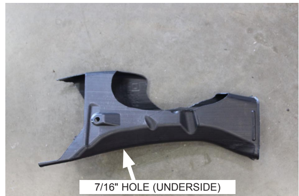
Fig. 6-b: Modified Brake Cooling Duct (Inner Section)
