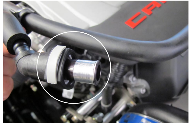
Fig. 8-d: Insert Hose Fitting To OEM Quick Release Fitting
