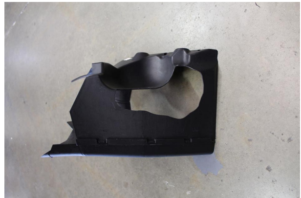
Fig. 6-a: Modified Supplemental Radiator Cooling Duct
