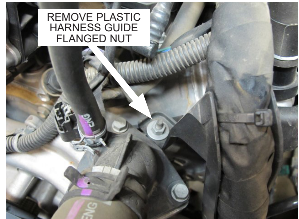
Fig. 1-G: Remove flanged nut
