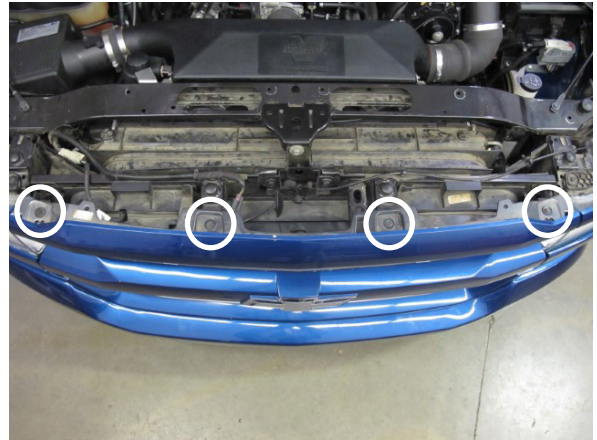
Fig. 2A-D: Remove upper grill screws then remove the grill
