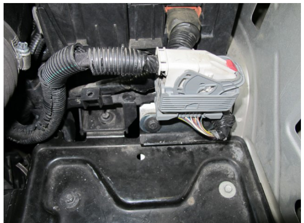
Fig. 4-L: Secure harness connector to relocation bracket
