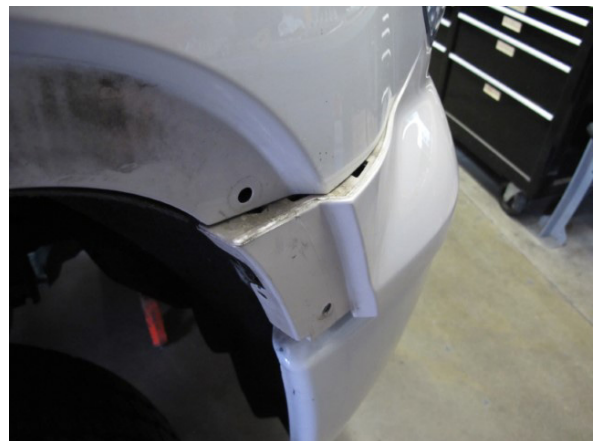
Fig. 2B-C: Detach bumper trim piece from front fenders
