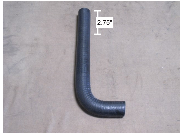
Fig. 9-D: Cut a 2.75" section of hose
