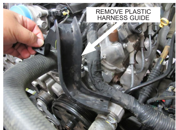
Fig. 1-I: Remove plastic harness guide
