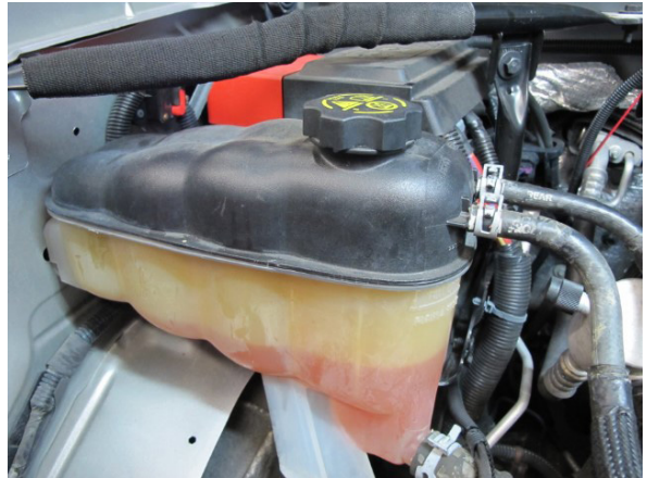
Fig.3-D: Refill engine coolant reservoir
