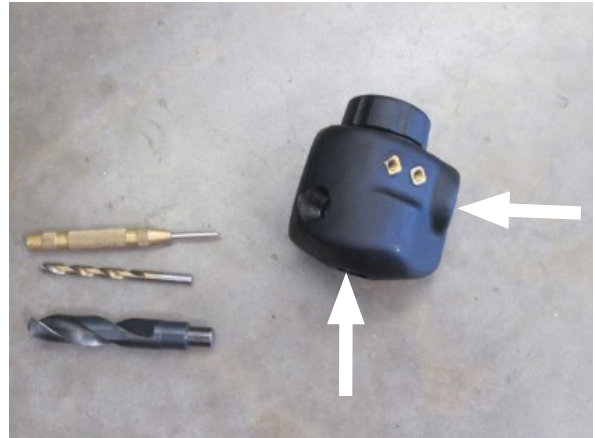
Fig. 8-A: Drill holes in surge tank
