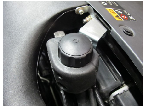
Fig. 8-GG: Install the surge tank cap
