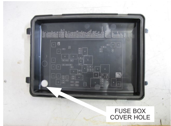
Fig. 8-N: Drill hole in fuse box cover
