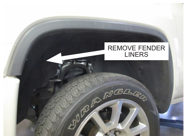
Fig. 1-O: Remove front fender liners
