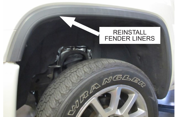
Fig. 13-D: Reinstall front fender liners
