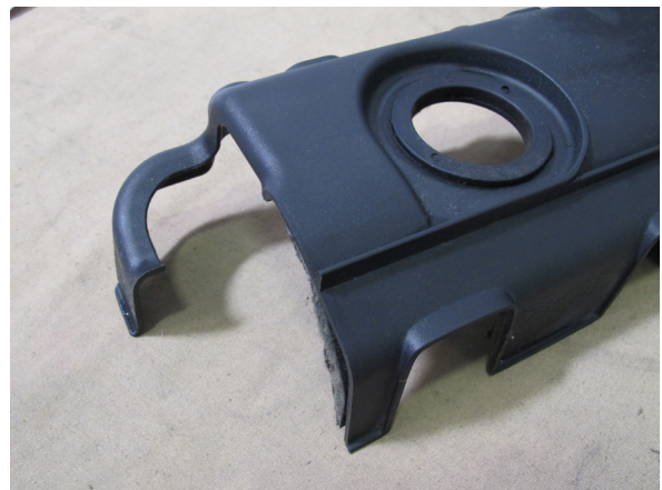
Fig. 12-C: Trim ignition coil cover
