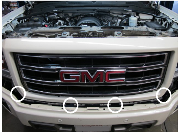
Fig. 2B-E: Remove screws securing the lower grill section
