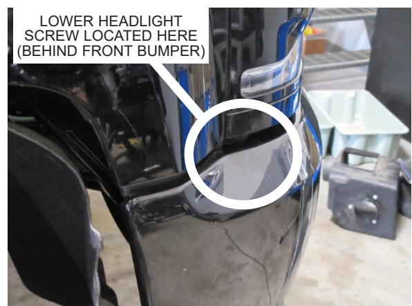
Fig. 13-C: Passenger side lower headlight screw location
