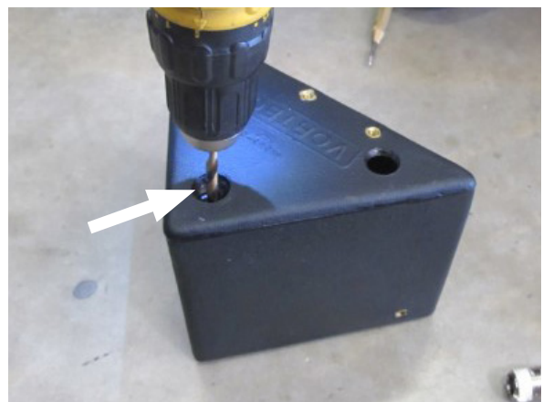
Fig. 8-C: Drill hole in reservoir
