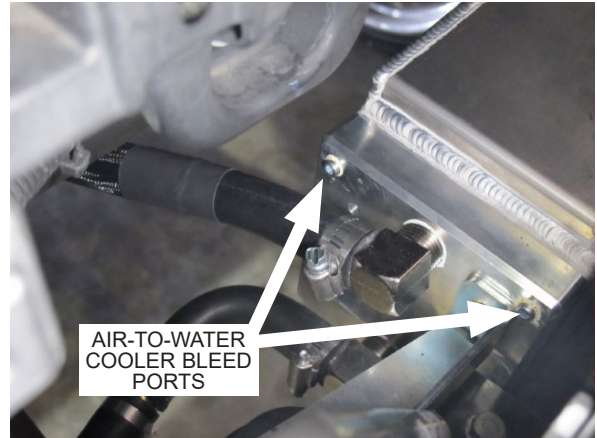
Fig. 8-EE: Air-to-water cooler bleed ports
