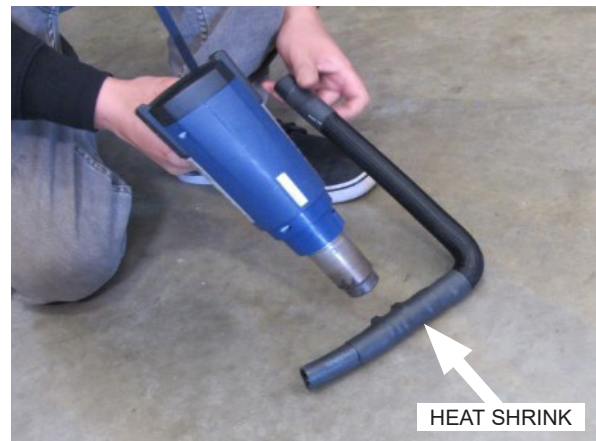
Fig. 8-W: Apply heat shrink to hose 4
