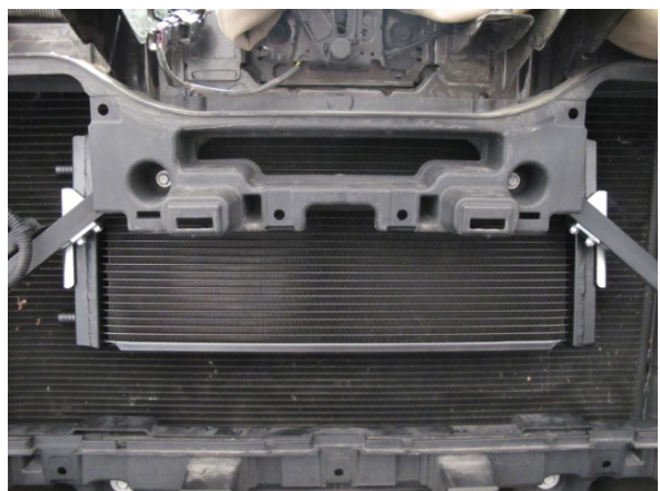
Fig. 7-F: Install heat exchanger and secure using self-tapping screws
