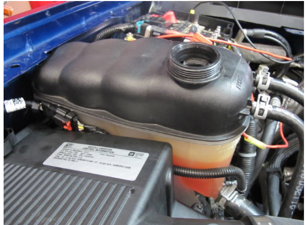
Fig. 3-A: Remove cap and drain coolant
