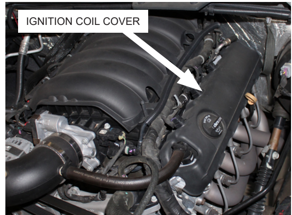
Fig. 1-M: Remove ignition coil cover
