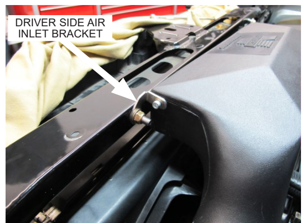
Fig. 10-L: Loosely install air inlet hardware
