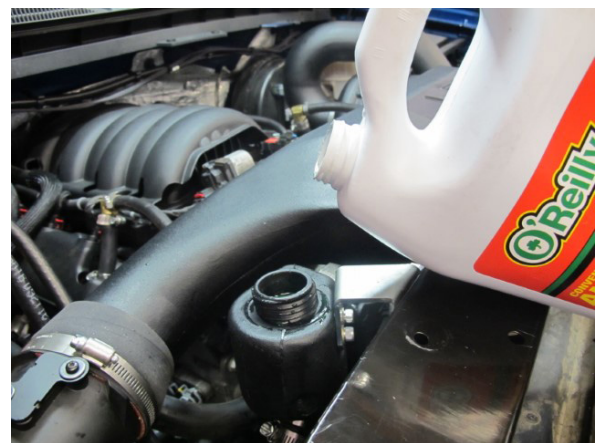
Fig. 8-DD: Fill coolant at surge tank
