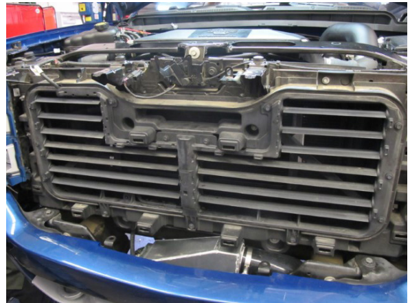
Fig. 13-E: Reinstall radiator shutters
