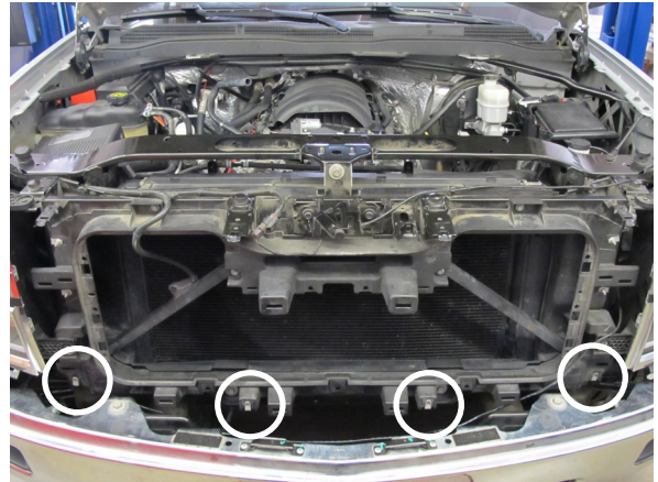
Fig. 2A-A: Remove lower grill screws
