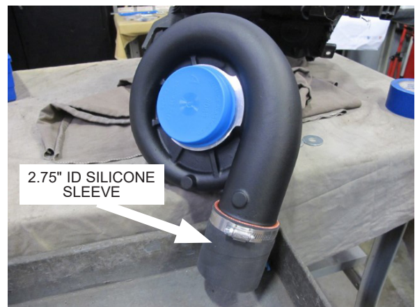
Fig. 5-C: Install straight 2.75" ID silicone sleeve
