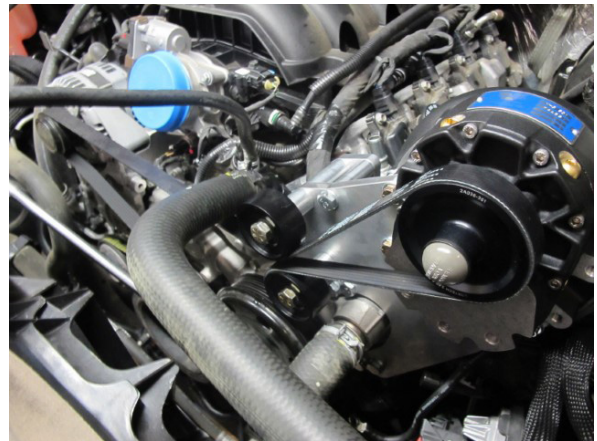
Fig. 5-E: Install 6-rib serpentine belt
