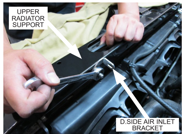
Fig. 10-C: Install driver side air inlet bracket
