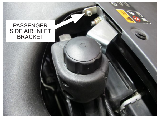
Fig. 10-M: Install passenger side air inlet hardware
