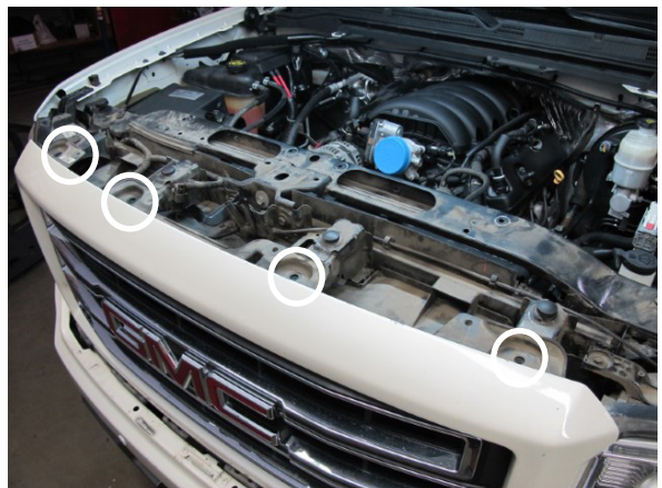
Fig. 2B-F: Remove screws securing the upper grill section then remove grill
