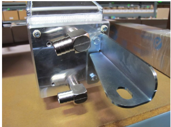
Fig. 6-G: Install driver side air-to-water cooler mounting bracket
