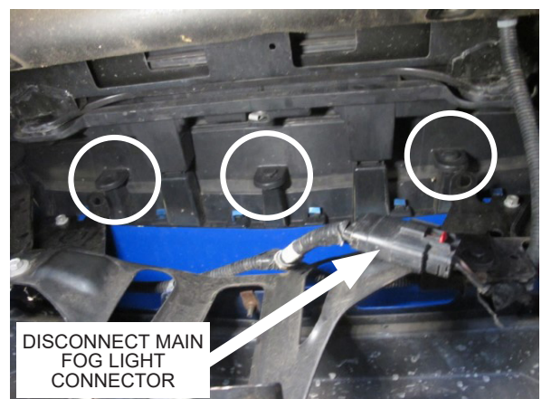
Fig. 2A-C: Remove three plastic clips and disconnect main fog light connector
