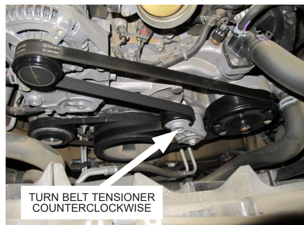
Fig. 1-F: Remove OEM serpentine belt
