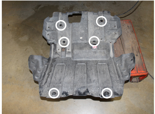
Fig. 1-P: Remove lower splash shield
