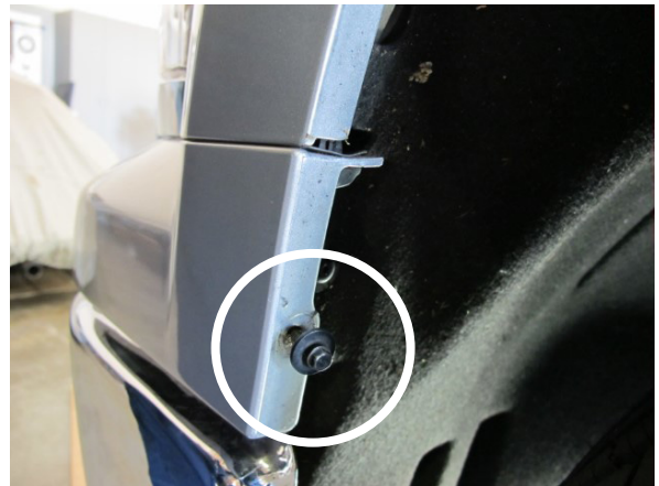
Fig. 2A-B: Remove corner grill screws
