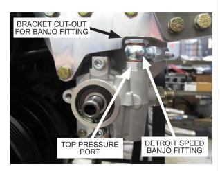
Fig. B: Top pressure port power steering pump with Detroit Speed banjo fitting
