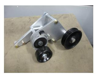
Fig. 3-B: Ribbed idler pulley (Vehicles without A/C only)
