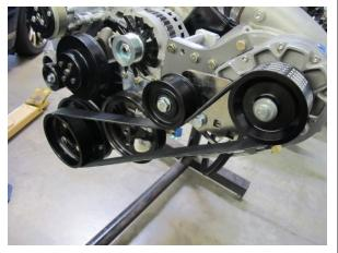
Fig. 6-D: Install supercharger drive belt
