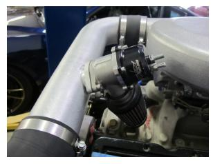
Fig. 7-J: Install bypass
