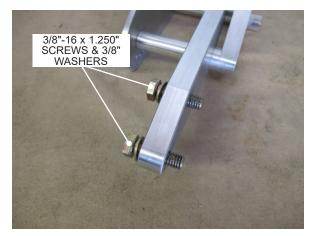
Fig. 4-E: Remove hardware
