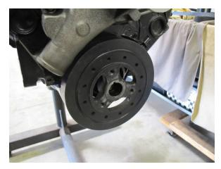
Fig. 1-D: Remove crank pulley and/or accessories from harmonic balancer
