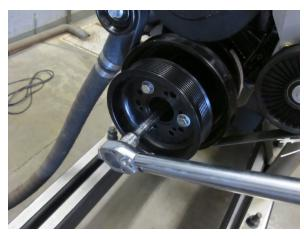
Fig. 5-F: Torque the crank bolt
