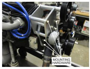
Fig. 3-D: Install A/C idler assembly
