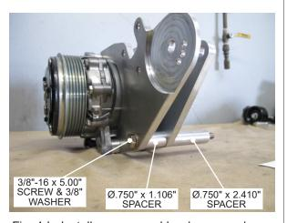
Fig. 4-L: Install spacers and hardware as shown
