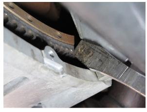
Fig. 5-A: Keep the engine from rotating
