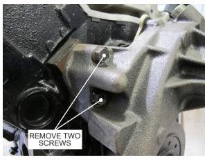
Fig. 3-A: Remove passenger side water pump screws
