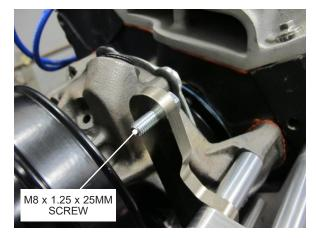
Fig. 2-F: Set alternator screw aside
