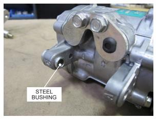
Fig. 4-J: A/C compressor steel bushings (Passenger side shown)
