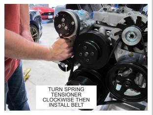
Fig. 5-J: Tension accessory drive belt
