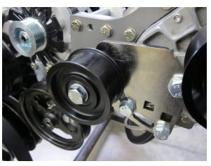
Fig. 6-C: Install flanged idler pulley
