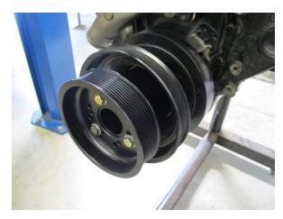
Fig. 5-E: Install belt drive assembly with accessory pulley to harmonic balancer
