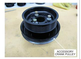
Fig. 5-D: Crank pulley assembly with accessory pulley
