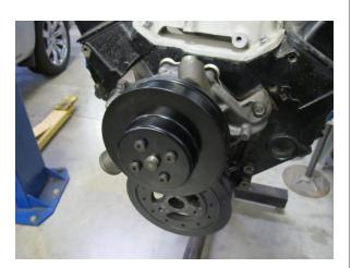
Fig. 1-C: Install water pump pulley
