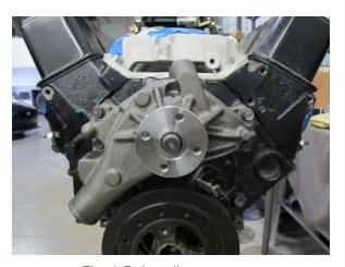
Fig. 1-B: Install water pump
