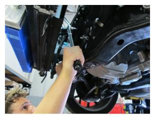
Fig. 5-B: Remove crank bolt
