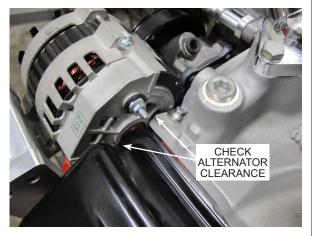
Fig. 2-E: Alternator clearance
