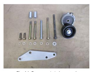
Fig. 4-I: Components to be reused
