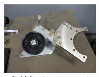
Fig. 2-C: Supercharger mounting bracket assembly
