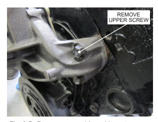
Fig. 2-B: Remove upper driver side water pump screw
