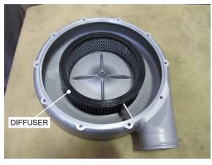
Fig. 7-A: Carburetor hat with diffuser
