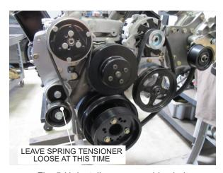
Fig. 5-H: Install accessory drive belt
