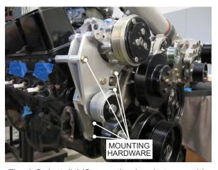
Fig. 4-Q: Install A/C mounting bracket assembly
