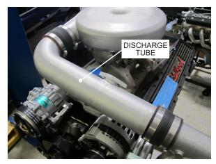
Fig. 7-H: Install discharge tube
