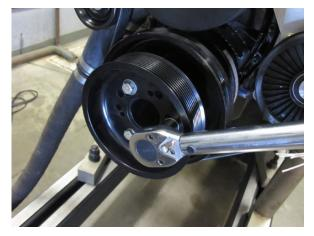
Fig. 5-G: Torque the 3/8"-16 x 5.00" screws
