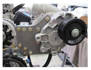
Fig. 6-A: Install supercharger
