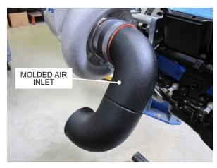
Fig. 8-C: Install molded air inlet to supercharger inlet
