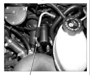
MODIFIED BRAKE BOOSTER HARD LINE MUST CLEAR INLET DUCT
