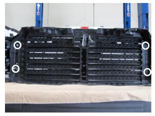
Fig. 1-W: Remove grill nuts
