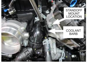
Fig. 2-K: Bend hardline for standoff clearance
