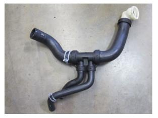
Fig. 1-G: Remove coolant hose assembly
