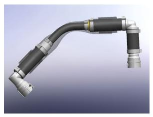
Fig. 2-N: Assemble the new PCV assembly
