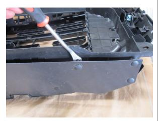
Fig. 1-V: Remove grill lower flap
