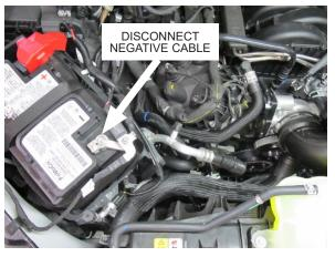
Fig. 9-I: Reconnect negative battery cable
