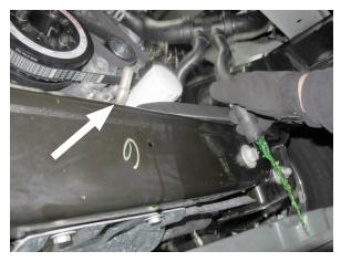
Fig. 1-F: Remove cap and drain coolant
