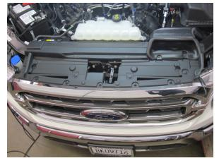
Fig. 9-H: Reinstall radiator support cover
