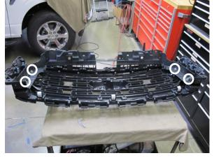
Fig. 2-E: Reattach shutter housing to grill
