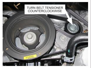
Fig. 1-E: Remove OEM serpentine belt
