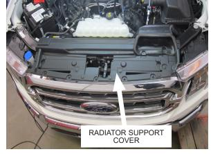
Fig. 1-N: Remove radiator support cover
