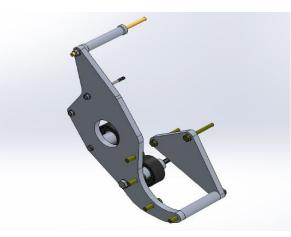
Fig. 3-A: Supercharger mounting bracket assembly
