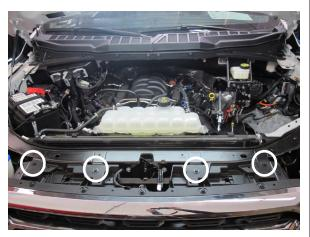
Fig. 1-P: Remove upper grill screws
