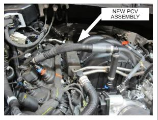
Fig. 2-O: Install new PCV assembly
