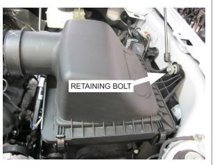
Fig. 6-A: Install air cleaner assembly
