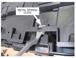
Fig. 1-Y: Remove shutter housing from grill
