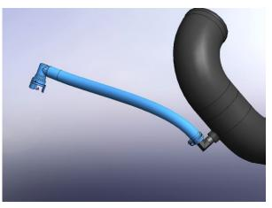
Fig. 6-E: Assemble PCV hose
