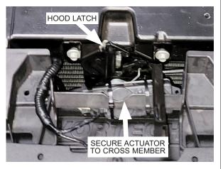
Fig.9-C: Mount air deflector motor
