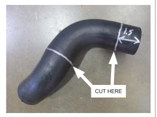
Fig. 2-G: Mark and cut coolant hose
