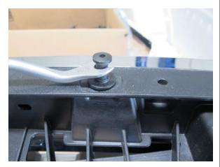
Fig. 1-X: Remove grill plastic fasteners
