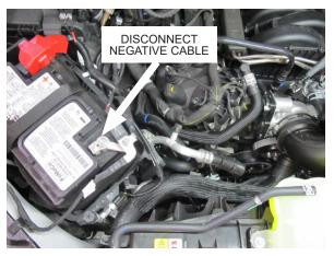
Fig. 1-A: Disconnect negative battery cable
