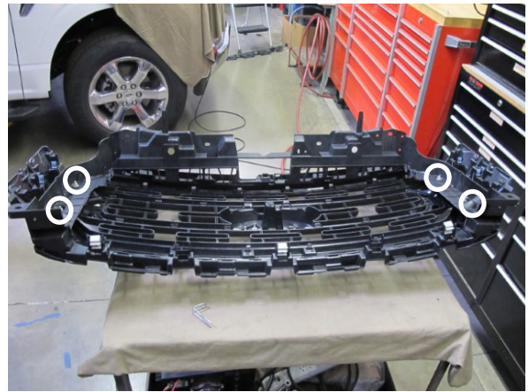
Fig. 2-E: Reattach shutter housing to grill
