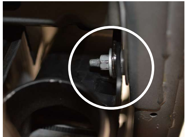
Fig. 4-y: Secure Charge Air Cooler
