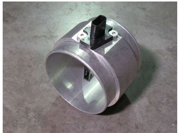
Fig. 4-ao: Install MAF Sensor To MAF Housing
