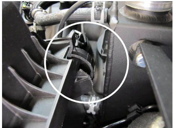
Fig. 7-g: Trim Air Box As Necessary
