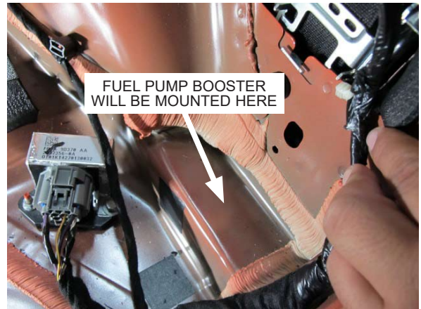
Fig. 6-j: Fuel Pump Booster Mounting Location
