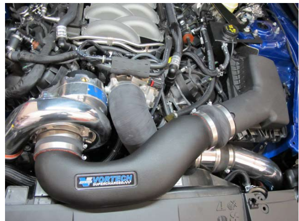
Fig. 7-l: Loosely Install Air Inlet Tube
