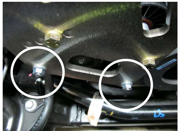
Fig. 2-l: Install 2x M8 Nuts & 2x 5/16" Washers
