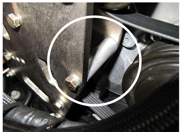
Fig. 2-r: Reinstall Previously Removed 1x 2.730" Spacer
