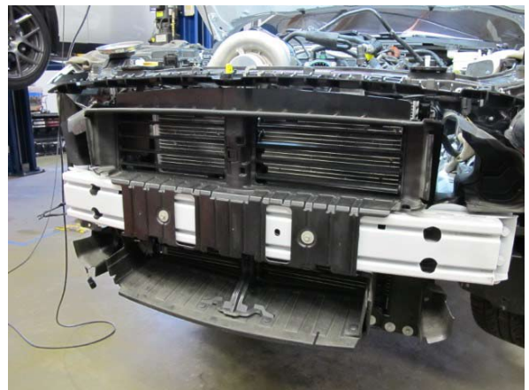
Fig. 1-o: Remove 8mm-Headed Fasteners
