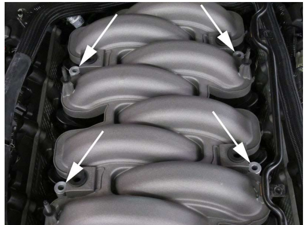
Fig. 5-n: Install Provided Fuel Rail Spacers
