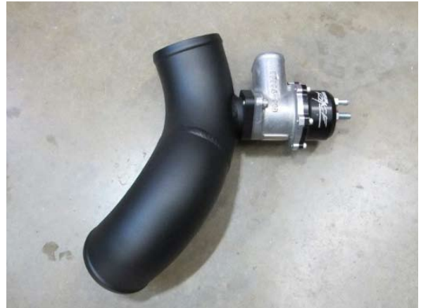
Fig. 4-ah: Install Bypass Valve (Automatic Transmission Vehicles)
