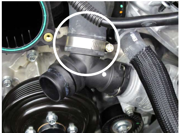
Fig. 3-h: Install #24 Hose Clamp
