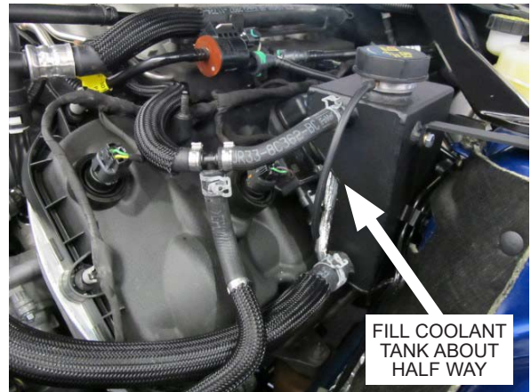
Fig. 3-y: Refill Cooling System
