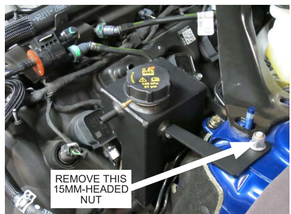
Fig. 3-r: Loosely Attach Coolant Tank
