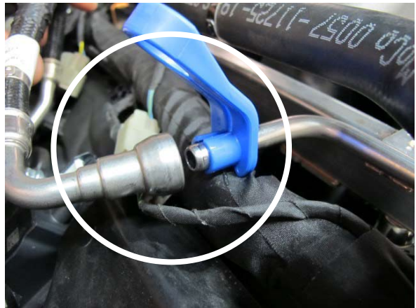
Fig. 5-g: Disconnect Direct Injection Fuel Line
