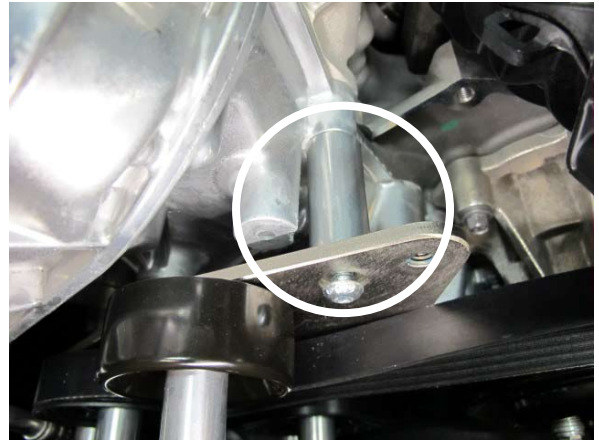
Fig. 2-j: Install 1x 2.058" Spacer
