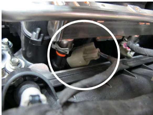
Fig. 5-d: Disconnect Fuel Injectors
