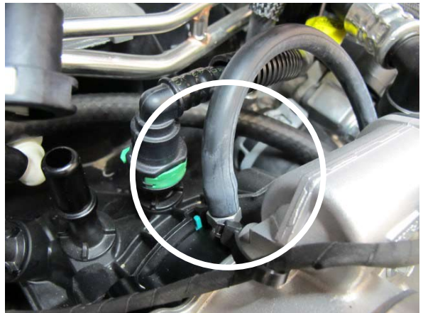
Fig. 4-ar: Attach Vacuum Hose To 1/4" Fitting
