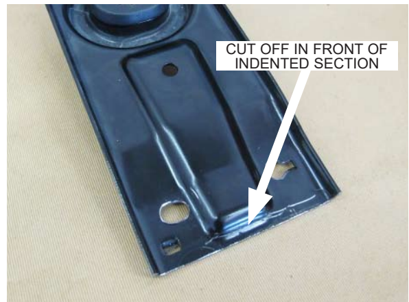
Fig. 3-e: Cut The Upper Radiator Bracket As Shown
