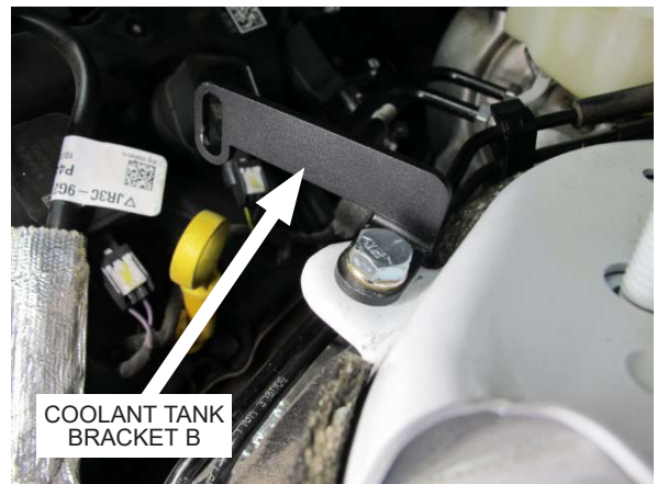
Fig. 3-q: Secure Coolant Tank Bracket B
