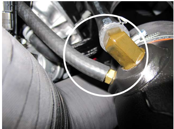
Fig. 7-m: Install 3/8" Hose, Then Secure Air Inlet Tube
