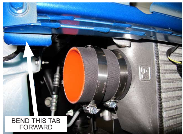
Fig. 4-aj: Install Silicone Sleeve & Hose Clamps
