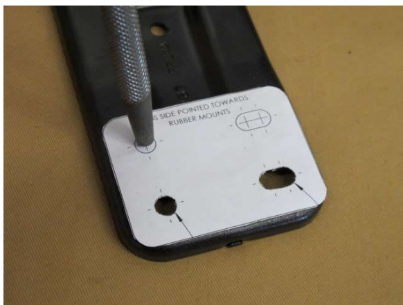
Fig. 3-c: Center Punch The Holes To Be Drilled
