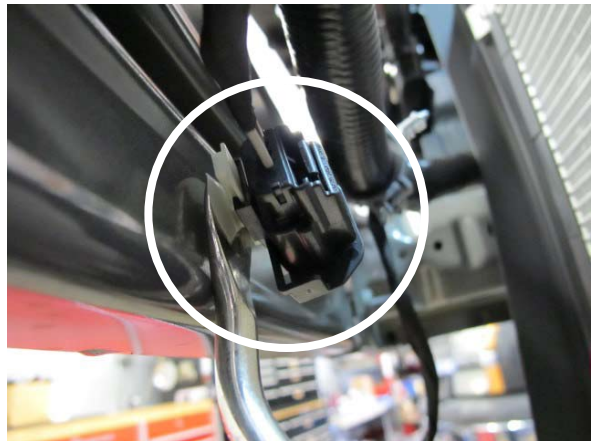
Fig. 4-n: Remove Unused Plug From Front Bumper Support
