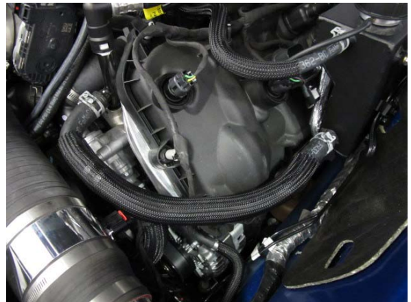
Fig. 3-w: Secure Modified OEM 3/4" Coolant Hose
