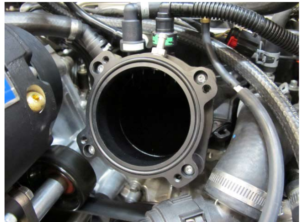
Fig. 4-b: Install Throttle Body Spacer
