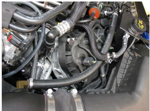
Fig. 7-i: Attach Breather Hose To Air Inlet
