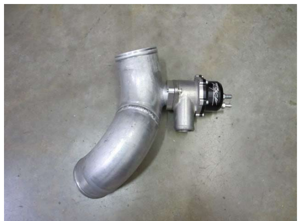
Fig. 4-ag: Install Bypass Valve (Manual Transmission Vehicles)
