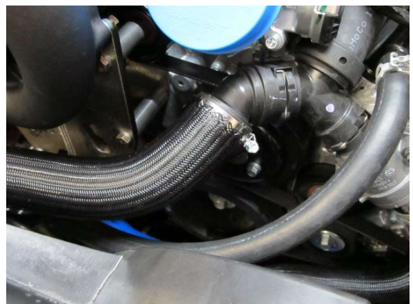
Fig. 3-l: Secure Quick-Release To Hose Using #24 Hose Clamp
