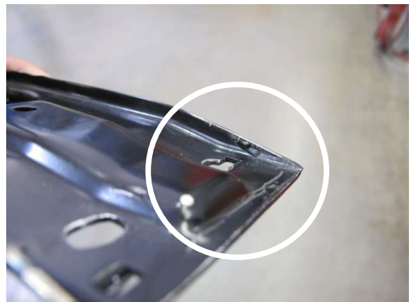
Fig. 3-f: Grind Down Raised Edges To A Taper
