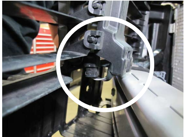
Fig. 1-s: Unplug Motor & Remove Active Grille Shutter Assembly
