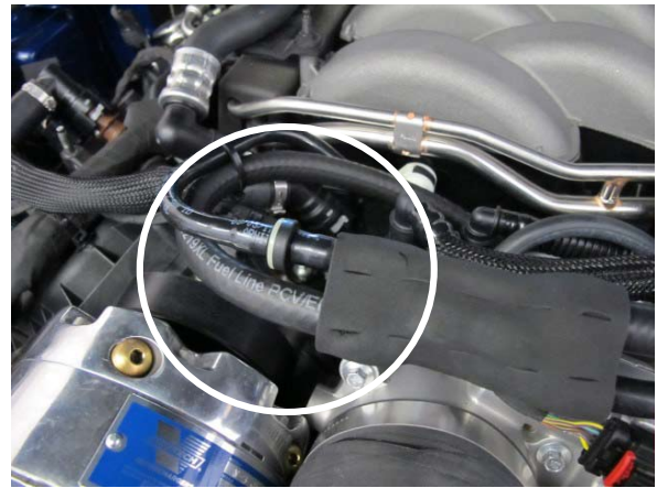
Fig. 7-k: Install 24" Length Of 3/8" Hose
