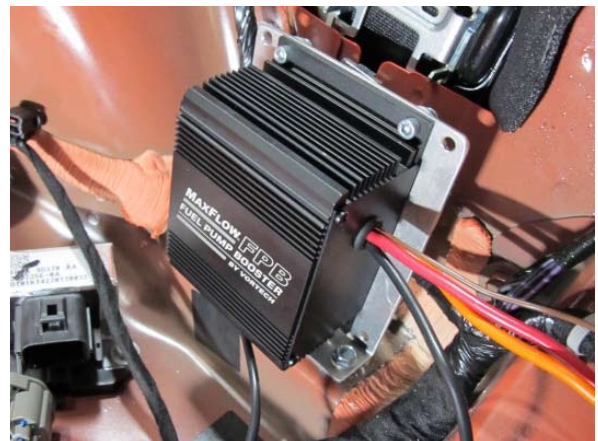
Fig. 6-l: Mount Fuel Pump Booster
