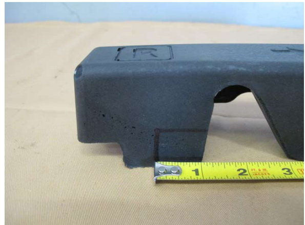
Fig. 5-m: Modify Passenger Side Fuel Rail Cover
