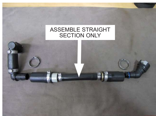
Fig. 7-c: Assemble Straight Section Of PCV Assembly
