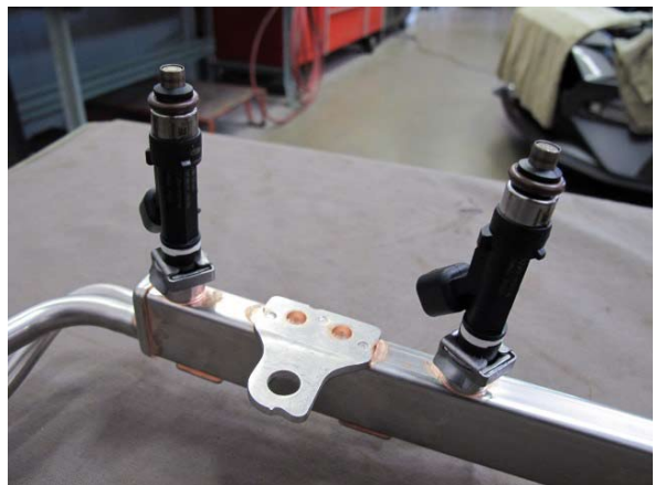
Fig. 5-i: Make Note Of Fuel Injector Orientation
