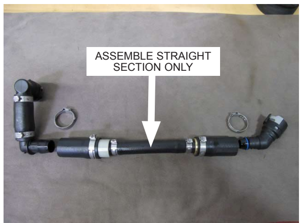
Fig. 7-c: Assemble Straight Section Of PCV Assembly
