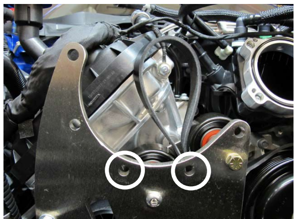
Fig. 2-o: Use long 9/16" Wrench To Install These Screws
