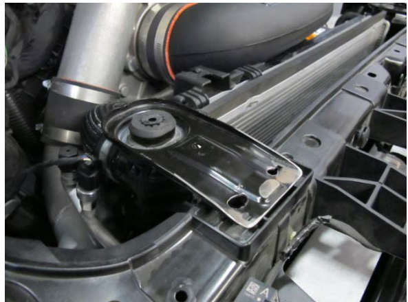
Fig. 3-g: Reinstall Modified Upper Radiator Brackets
