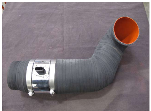
Fig. 4-ap: Assemble MAF Sensor Housing & Sleeves As Shown
