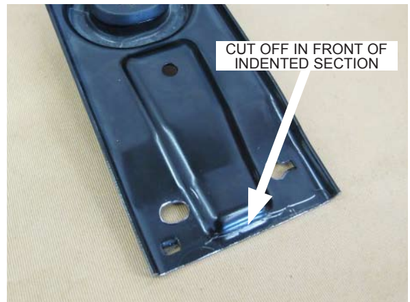
Fig. 3-e: Cut The Upper Radiator Bracket As Shown
