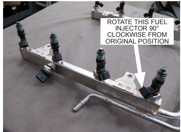
Fig. 5-j: Rotate Fuel Injector 90° Clockwise
