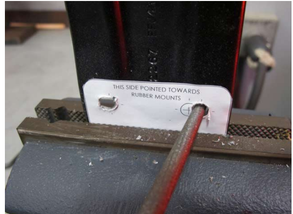
Fig. 3-d: Use Round File To Slot Hole
