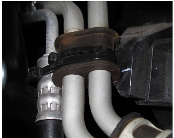
Fig. 10-d: Secure Transmission Cooler Lines To A/C Line via Rubber Isolator
