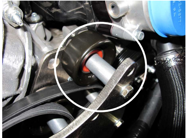
Fig. 3-m: Re-Install Upper Smooth Idler
