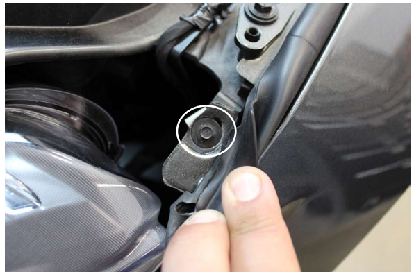
Fig. 1-b: Remove 5.5mm-Headed Fastener
