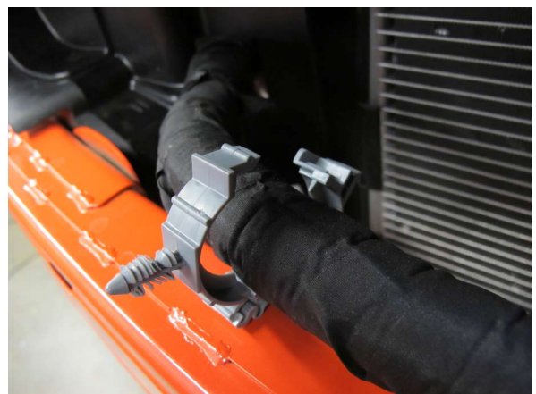
Fig. 1-l: Gray Clip Removal
