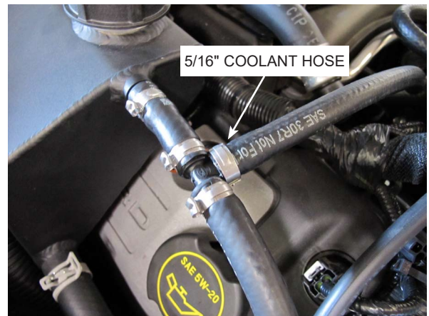
Fig. 7-k: Small Coolant Hose
