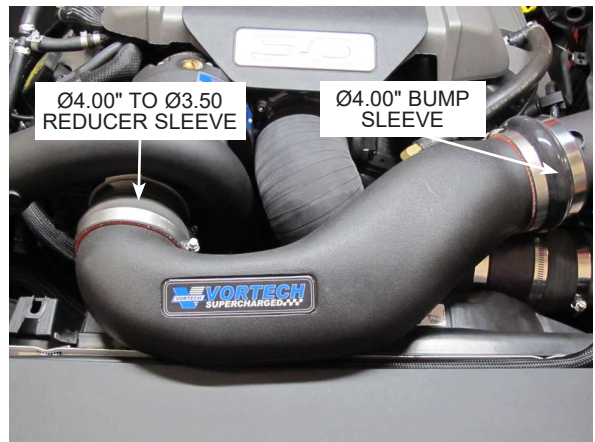
Fig. 8-b: Attach Air Inlet Duct To Air Box
