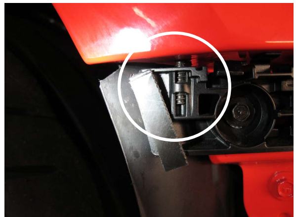
Fig. 1-f: Bumper Corner Fastener (Bumper Removed)
