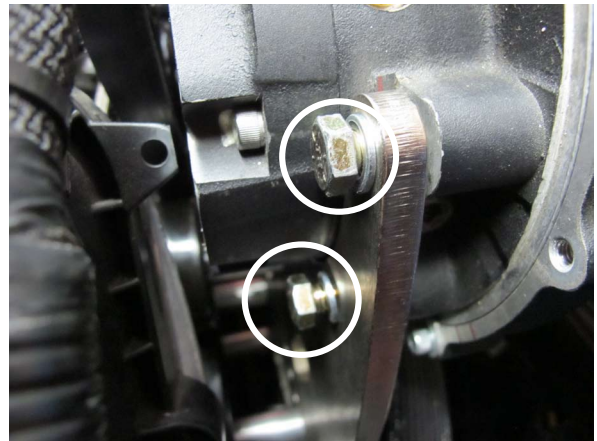
Fig. 3-q: Mount Supercharger To Bracket & Secure
