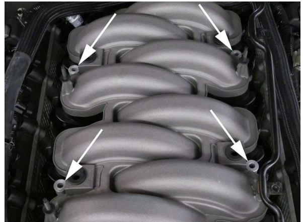
Fig. 6-d: Aluminum Fuel Rail Spacers
