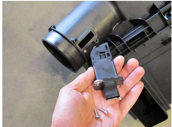
Fig. 1-s: MAF Insert (shown with OEM airbox removed)
