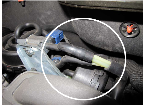
Fig. 8-d: Recirculating IMRC Solenoids
