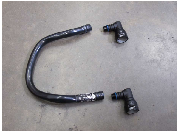
Fig. 4-a: OEM Passenger Side PCV Hose (Fittings Removed)
