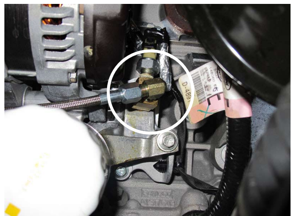
Fig. 11-f: Oil Feed Assembly Orientation
