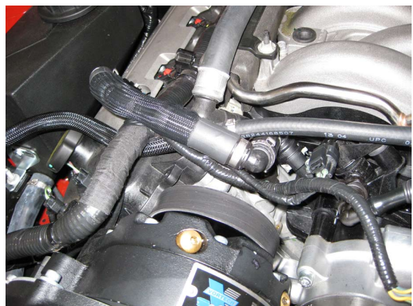
Fig. 4-c: Modified Passenger Side PCV Hose
