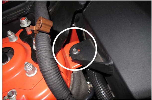
Fig. 7-g: Coolant Reservoir Mount #2
