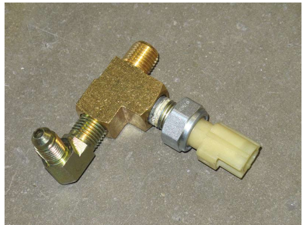
Fig. 11-e: Oil Feed Assembly (shown removed for clarity)
