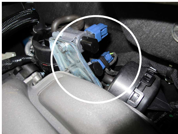
Fig. 8-p: Vented IMRC Solenoids
