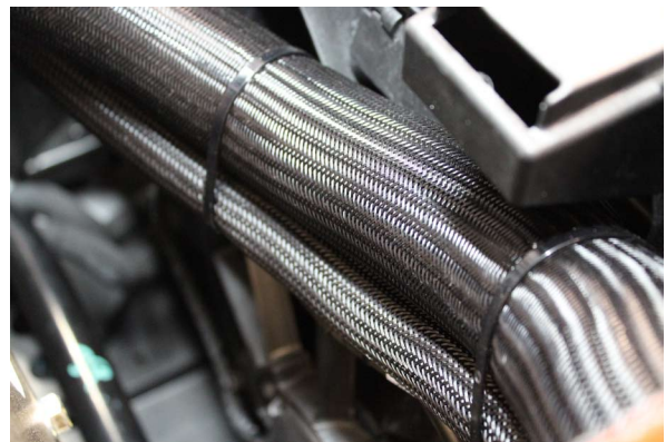
Fig. 7-o: 3/4" Coolant Hose Routing
