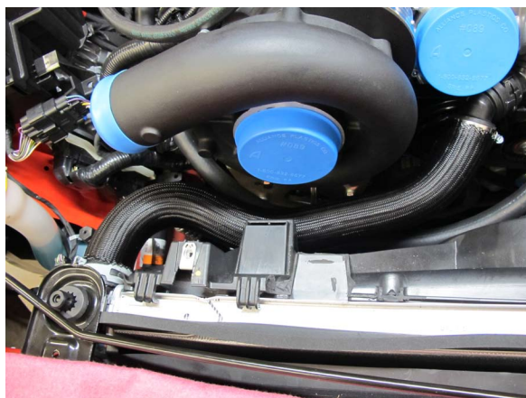
Fig. 7-c: Upper Radiator Hose (New Configuration)
