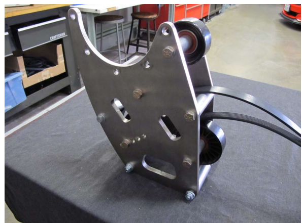
Fig. 3-c: Inspect Mounting Bracket Assembly
