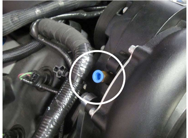
Fig. 11-a: Supercharger Oil Feed Location
