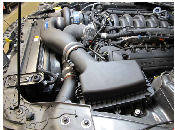
Fig. 8-c: Leave Air Inlet Assembly Loose At This Time
