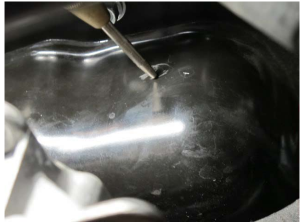
Fig. 12-d: Punch Hole In Oil Pan
