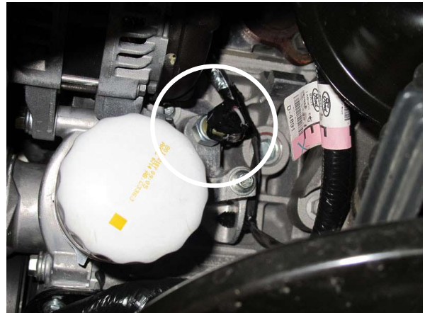
Fig. 11-d: OEM Oil Pressure Sensor
