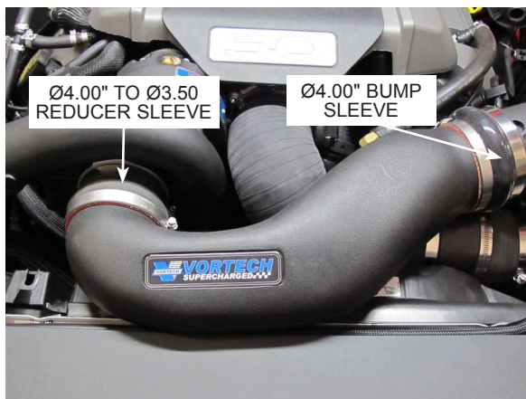
Fig. 8-b: Attach Air Inlet Duct To Air Box
