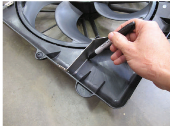
Fig. 3AD: Marking Air Dam Cut Lines
