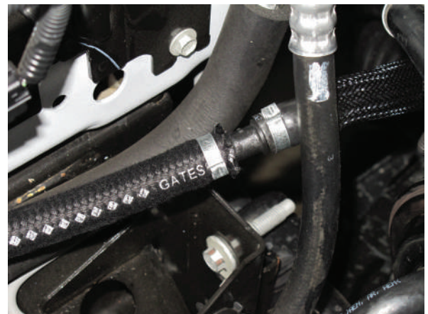
Fig. 2H-1: Joining A/T Hoses
