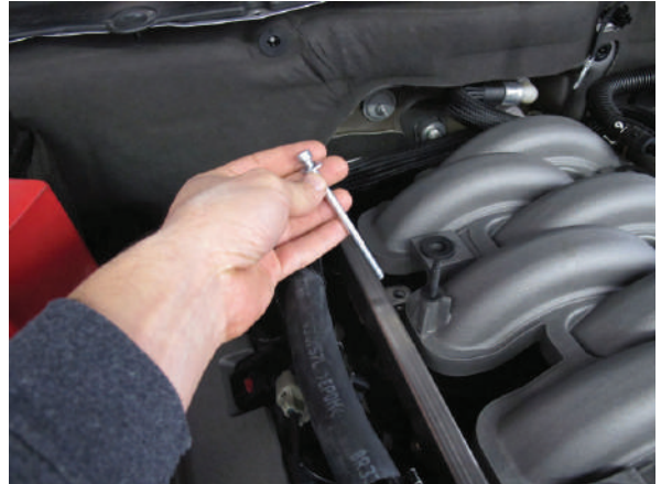
Fig. 9M: Re-securing Fuel Rails
