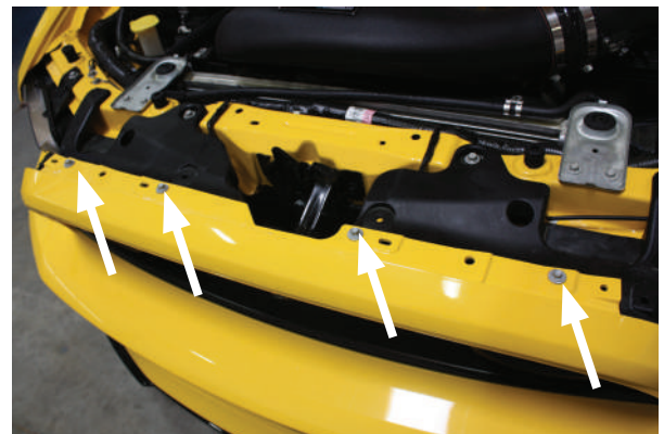
Fig. 1G: Top Bumper Cover Fasteners ('13-'14 Mustang)
