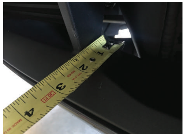
Fig. 12D-5: Bumper Cover, Center; Cut Line Reference
