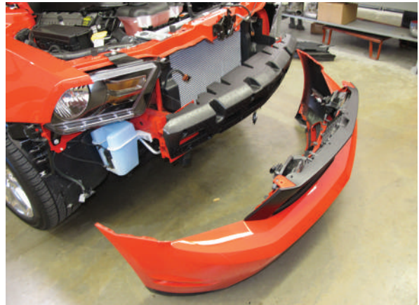
Fig. 1J: Front Fascia Removal
