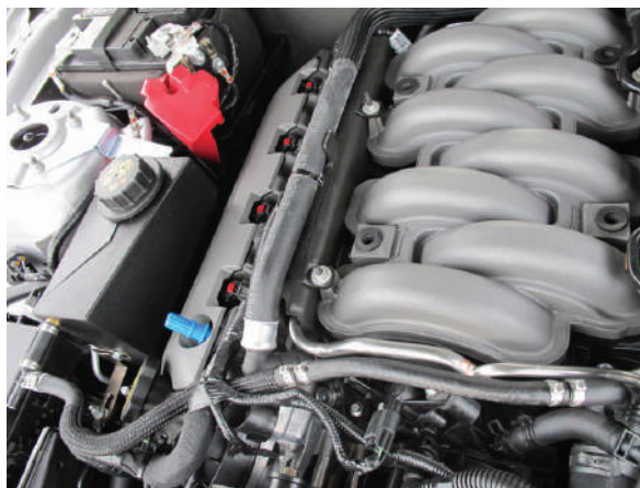
Fig. 3X: 5/16" Coolant Hose, Extended
