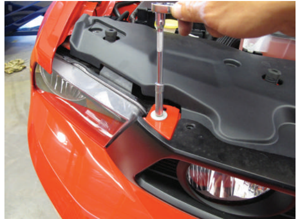
Fig. 1F: Top Edge Fasteners ('11-'12 Mustang)
