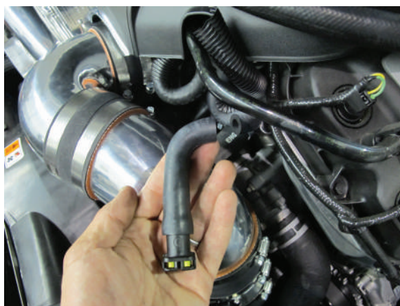
Fig. 11E: Auto Trans Vacuum Hose Cut
