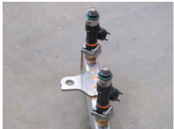
Fig. 9K: Fuel Rail / Injector Assembly Detail
