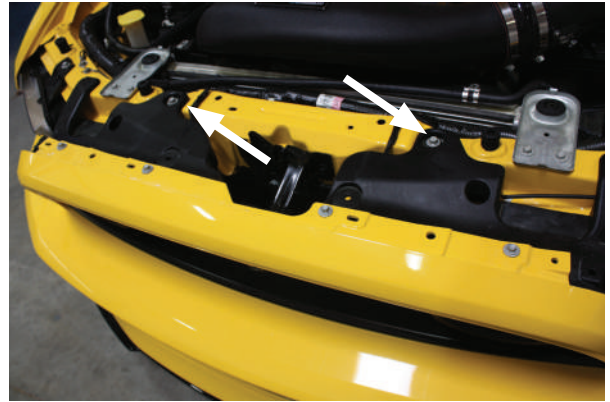
Fig. 1N: Bumper Cover Support Fasteners ('13-'14 Mustang)
