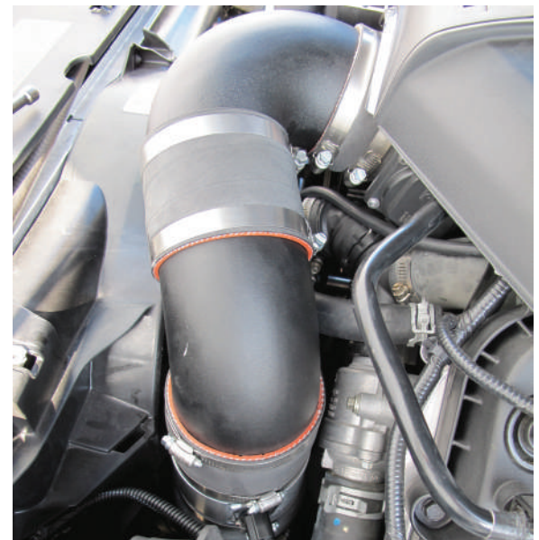
Fig. 7C-7: Cast Elbows, Final Position
