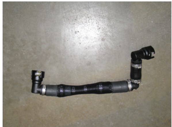
Fig. 5D-3: Modified Passenger Side PCV Hose
