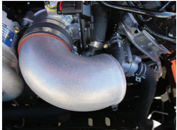
Fig. 7C-6: \text{\O}3.5 " x 120^\circ Cast Aluminum Elbow
