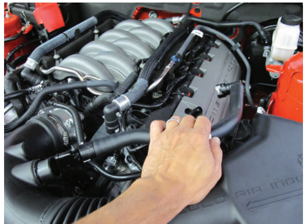
Fig. 1S: PCV Hoses
