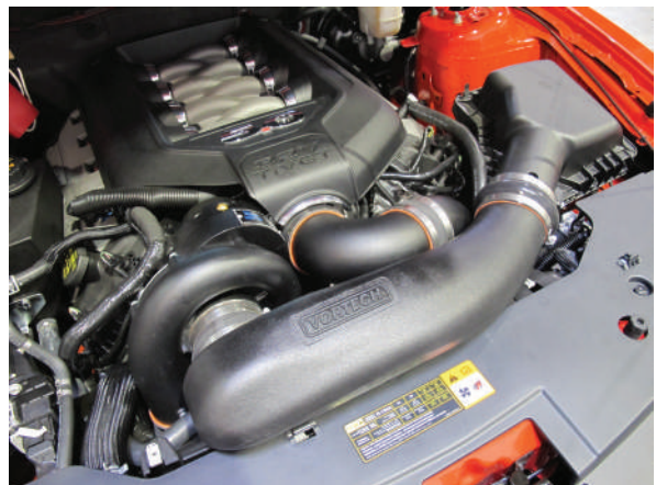
Fig. 11K: Complete Air Inlet Assembly
