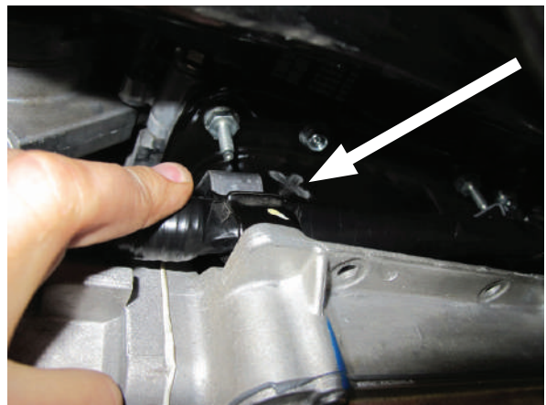
Fig. 14B: Oil Drain Fitting Installation Location
