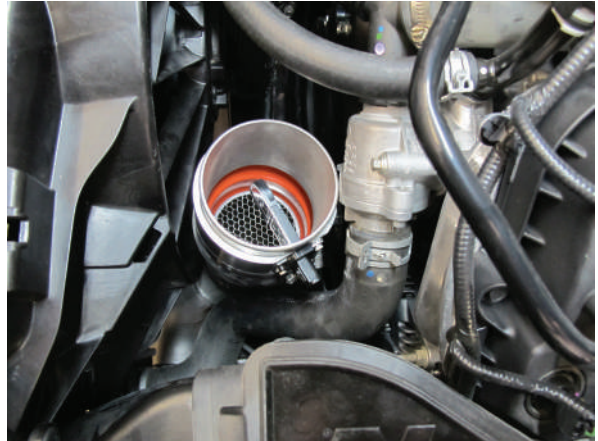
Fig. 7C-5: MAF Location (orientation will vary)
