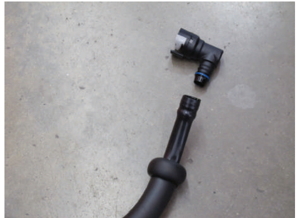
Fig. 5B: OEM Driver Side PCV Hose
