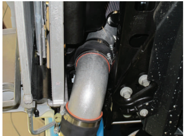
Fig. 7B-2: 90^\circ Tube and Bump Coupler
