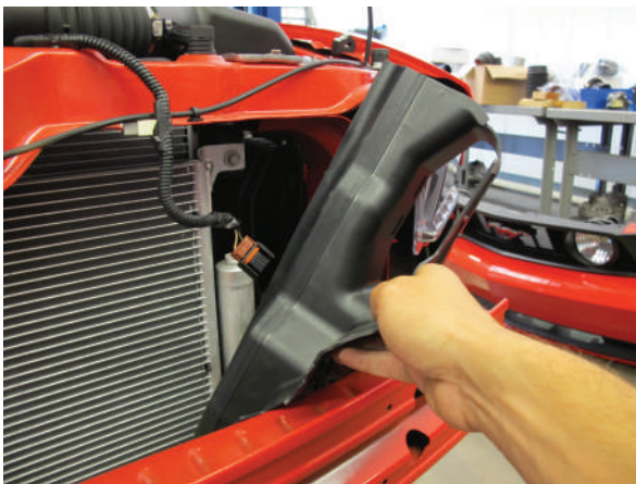
Fig. 1M: Radiator Side Shroud, Driver ('11-'12 Mustang)
