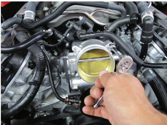
Fig. 1AG: Throttle Body Fasteners
