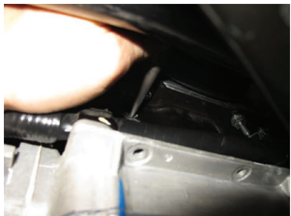
Fig. 14D: Punching Hole in Oil Pan
