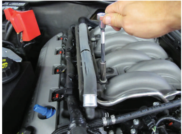
Fig. 9B: Hose Guide Removal
