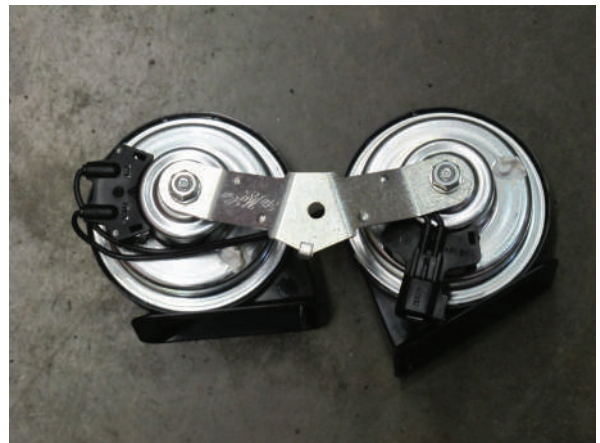
Fig. 6B: Modified Horn Bracket Orientation
