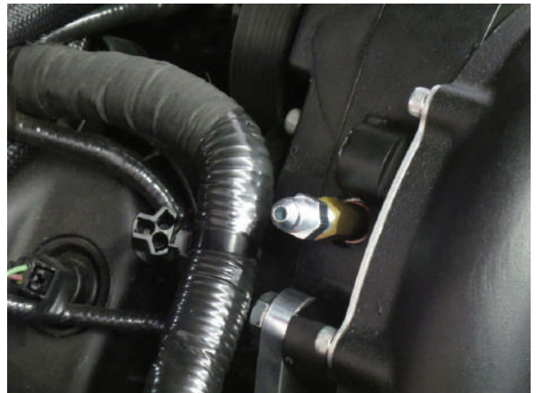
Fig. 13B: -4AN Oil Feed Fitting Installed
