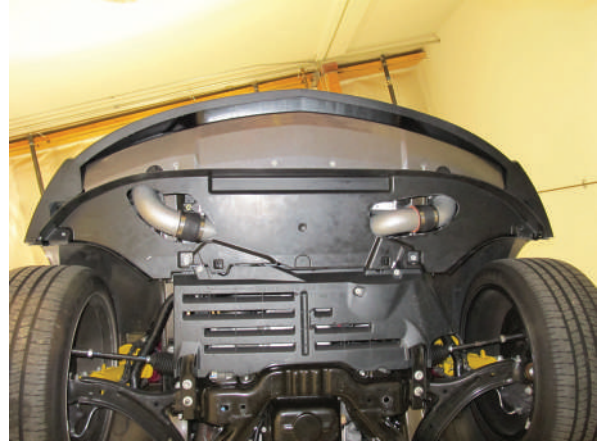
Fig. 12E-3: Plastic Undertray Trimming
