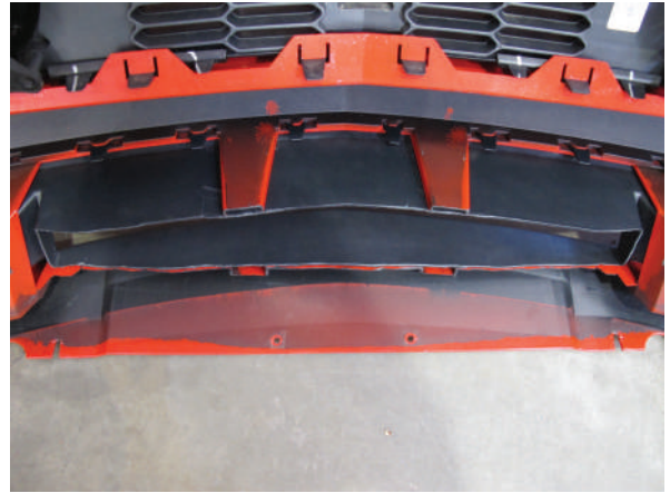
Fig. 12D-4: Bumper Cover, Center; Cut Line Reference
