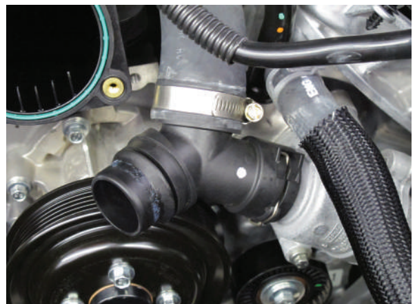
Fig. 2C: #28 Hose Clamp Orientation
