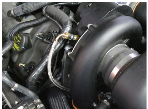
Fig. 13C: 90° Oil Feed Hose Installed
