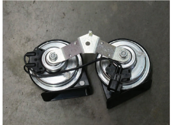
Fig. 6A: OEM Horn Bracket Orientation
