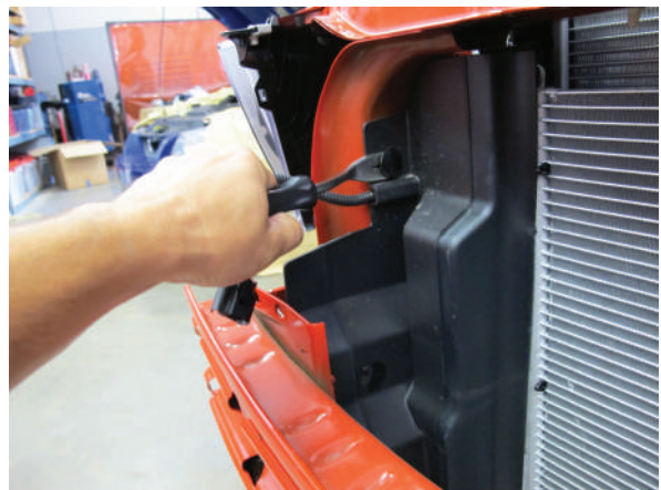
Fig. 1L: Radiator Side Shroud, Passenger ('11-'12 Mustang)
