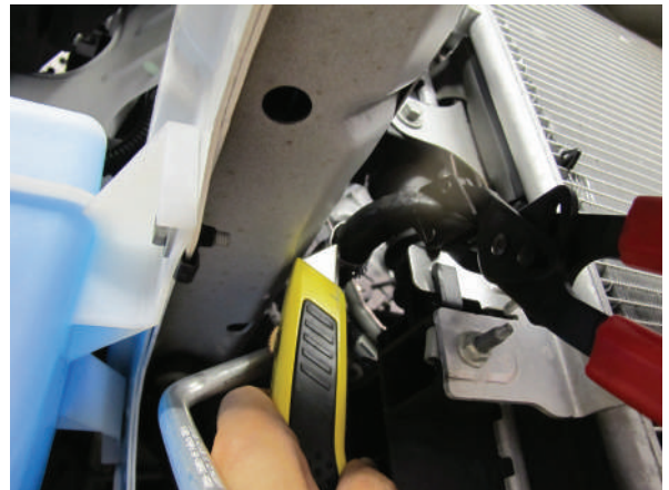
Fig. 2G: Clamping and Cutting A/T Hoses
