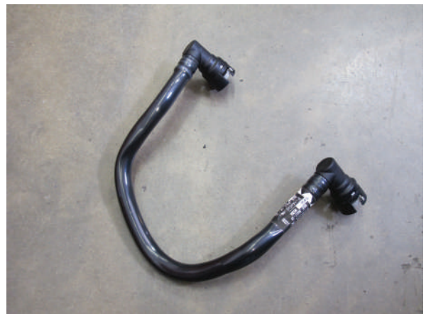
Fig. 5C: OEM Passenger Side PCV Hose
