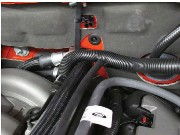
Fig. 8A-4: Vacuum Hose, Complete
