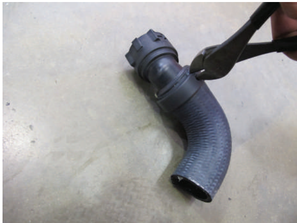
Fig. 3E: OEM Plastic Hose Clamp
