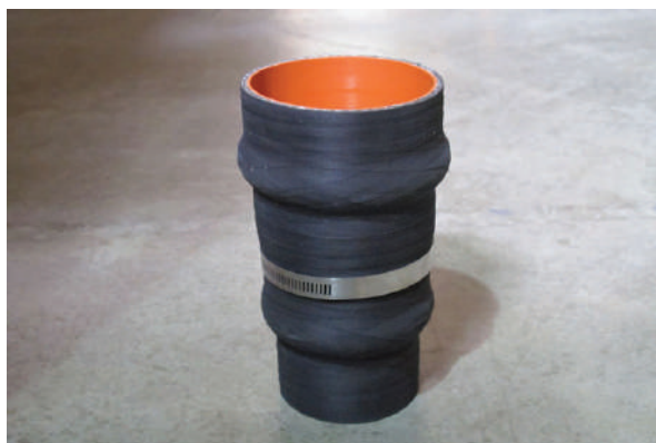
Fig. 7C-4: Stepped Coupler with Flow Straightener
