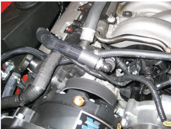
Fig. 5D-4: Modified Passenger Side PCV Hose, Installed
