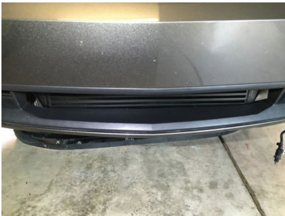
Fig. 12D-7: Bumper Cover, Center; Cut Line Reference
