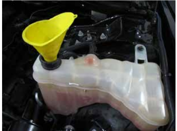
Fig. 5-g: Close coolant drain valve and refill engine coolant system
