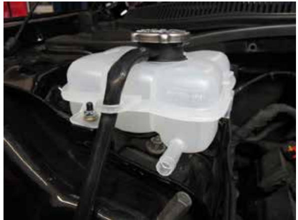
Fig. 9-m: Install air/water cooler system reservoir to mount
