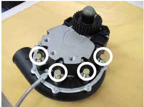
Fig. 8-b: Lubricate supercharger mounting boss threads
