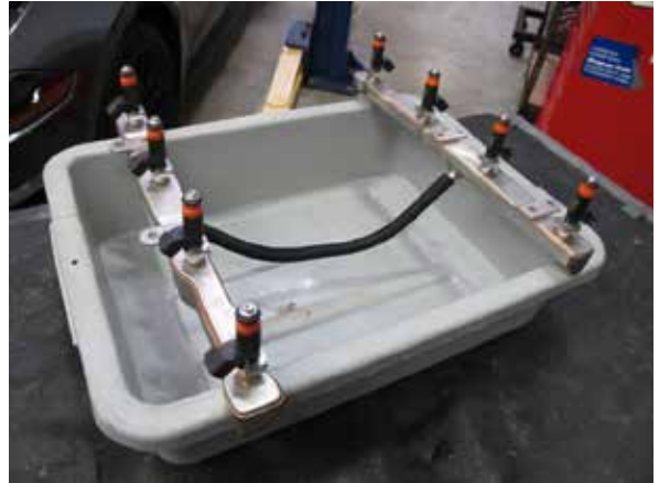
Fig. 10-g: Install provided high-flow injectors
