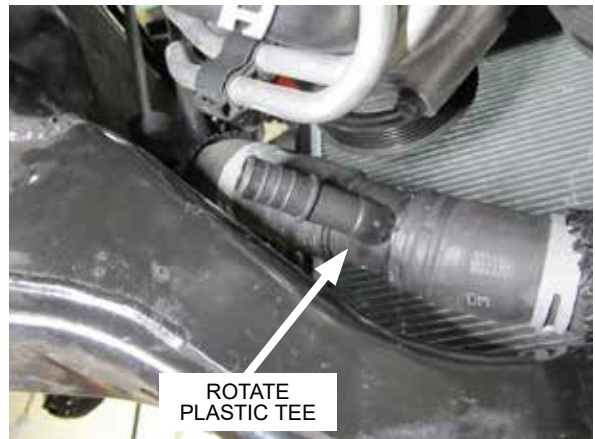
Fig. 5-d: Rotate plastic tee 180° clockwise
