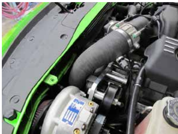
Fig. 7-ae: Install discharge sleeve 'E' and reconnect IAT sensor
