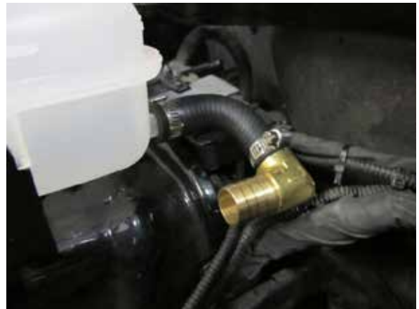
Fig. 9-q: Install hose and brass fitting assembly to air/water cooling system reservoir
