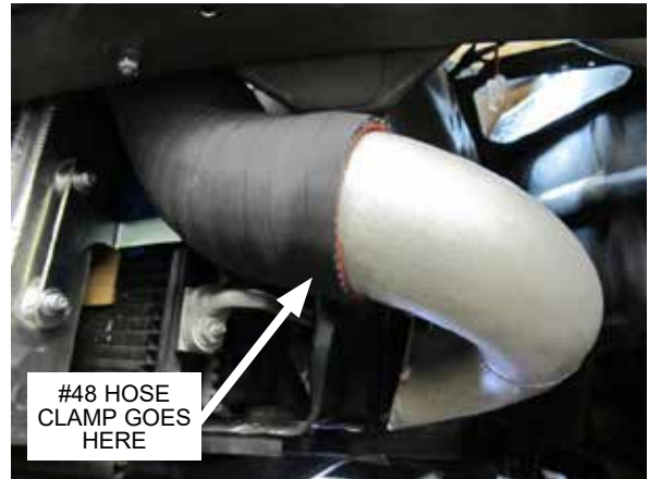
Fig. 7-ab: Loosely install discharge tube 'D'
