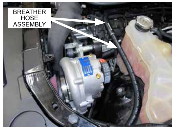
Fig. 8-f: Install breather hose assembly
