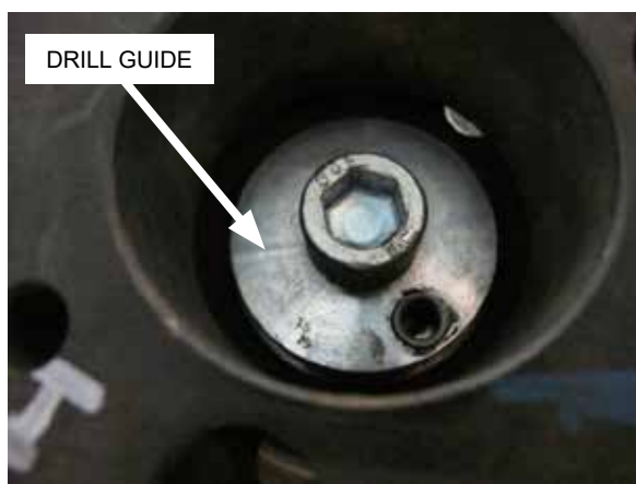
Fig. 3-b: Install drill guide
