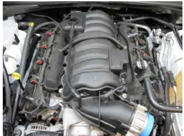
Fig. 10-h: Reinstall fuel rail assembly, fuel rail covers, and engine covers
