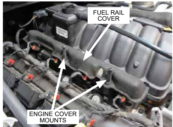
Fig. 10-d: Remove fuel rail covers, engine covers, and engine cover mounts (Passenger side shown)
