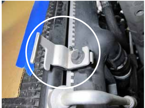
Fig. 7-g: Remove aluminum bracket and screw
