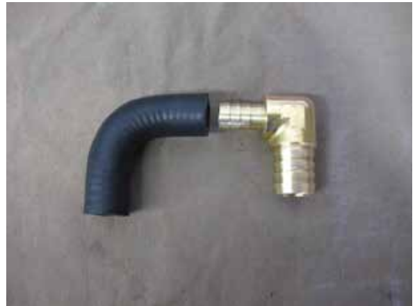
Fig. 9-p: Insert brass fitting to 1/2" x 90° coolant hose elbow
