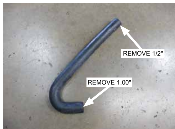
Fig. 9-i: Modify 150° molded hose as shown
