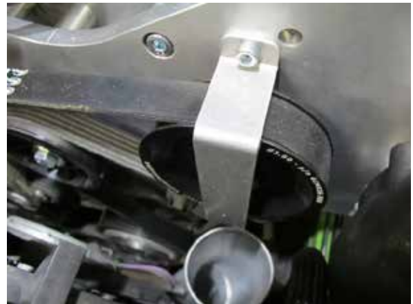
Fig. 6-k: Reinstall pulley guard
