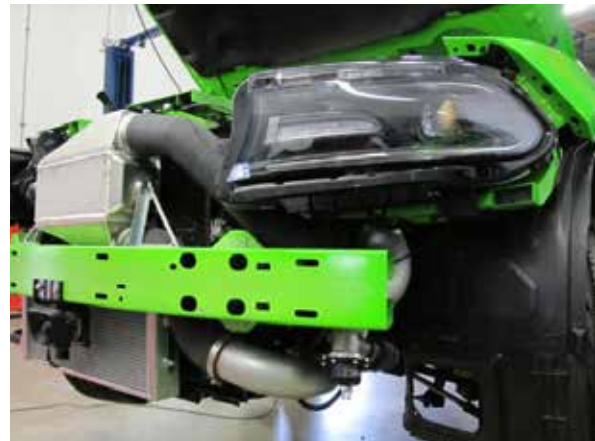
Fig. 8-h: Secure discharge tubes and discharge sleeves
