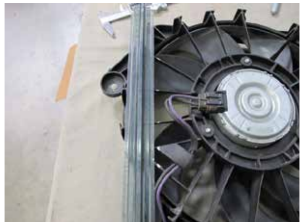
Fig. 4-c: Mark ribs using straight edge and marker
