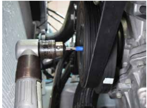
Fig. 3-d: Drill crankshaft / damper assembly
