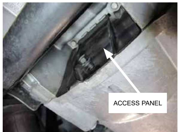
Fig. 3-i: Reinstall flywheel / flexplate access panel
