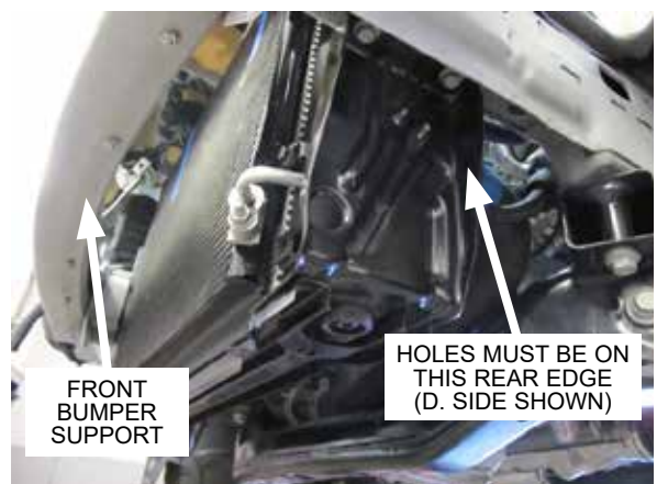
Fig. 4-l: Reinstall lower radiator support
