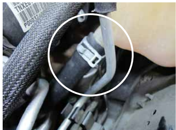
Fig. 5-f: Attach coolant hose to coolant reservoir
