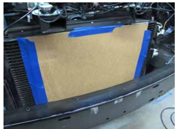
Fig. 7-f: Cover A/C condenser with cardboard
