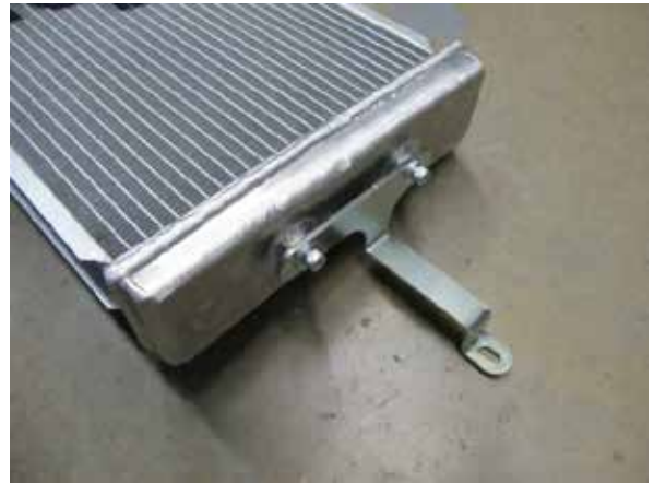
Fig. 7-j: Install driver side heat exchanger bracket
