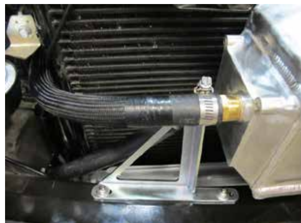
Fig. 9-u: Attach 3/4" coolant hose to air/water cooler
