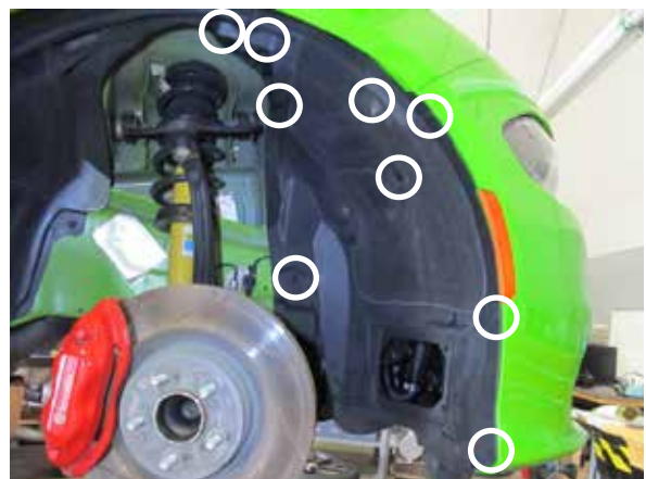
Fig. 2-c: Remove fender liner fasteners
