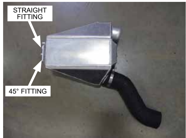
Fig. 7-w: Install discharge sleeve 'C' to the air/water cooler as shown
