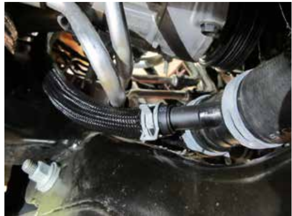
Fig. 5-e: Assemble new coolant reservoir hose as shown
