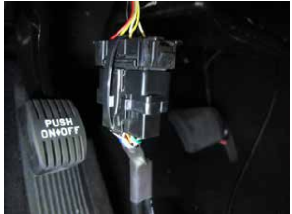
Fig. 13-d: Secure programming cable to factory OBD II port
