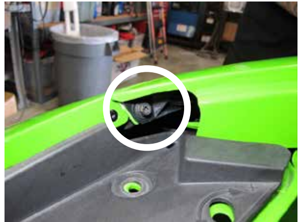
Fig. 2-g: Remove each upper front bumper cover screw
