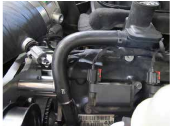
Fig. 8-e: Modify OEM breather hose
