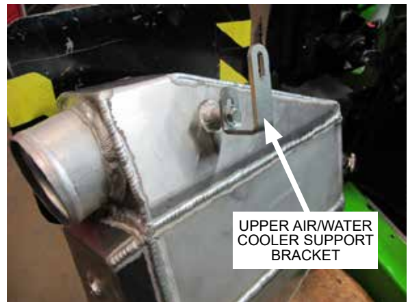
Fig. 7-q: Install upper air/water cooler support bracket
