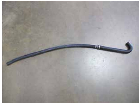
Fig. 9-w: 3/4" x 150° to 1/2" coolant hose assembly
