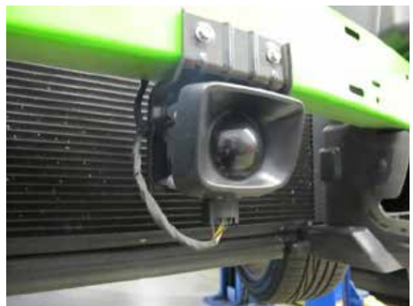
Fig. 2-i: Disconnect adaptive cruise control sensor
