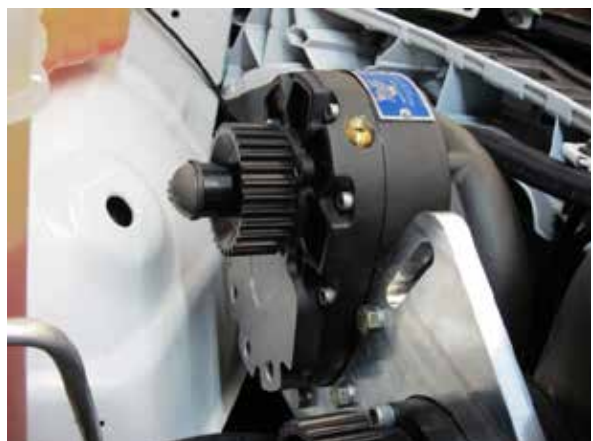
Fig. 8-c: Install supercharger to supercharger mounting bracket assembly
