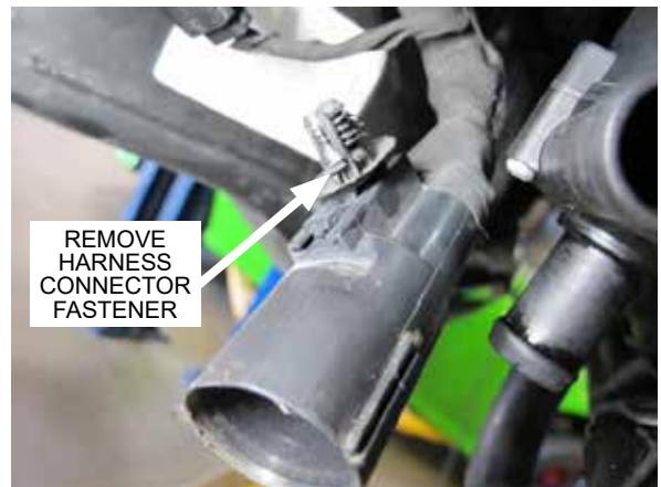
Fig. 9-e: Remove plastic harness connector fastener
