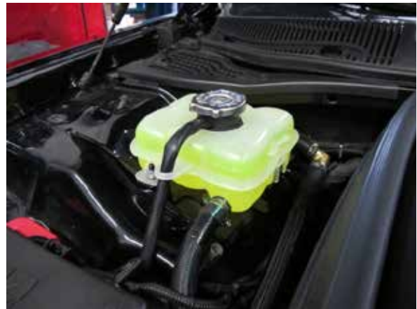
Fig. 9-z: Fill air/water cooling system with 50/50 water/coolant mix
