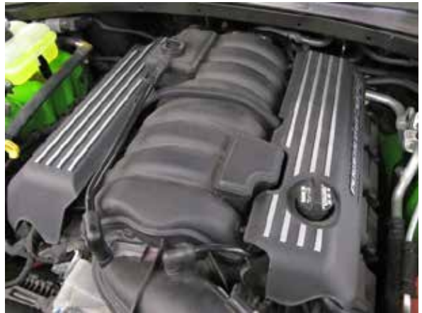
Fig. 10-a: Remove engine covers
