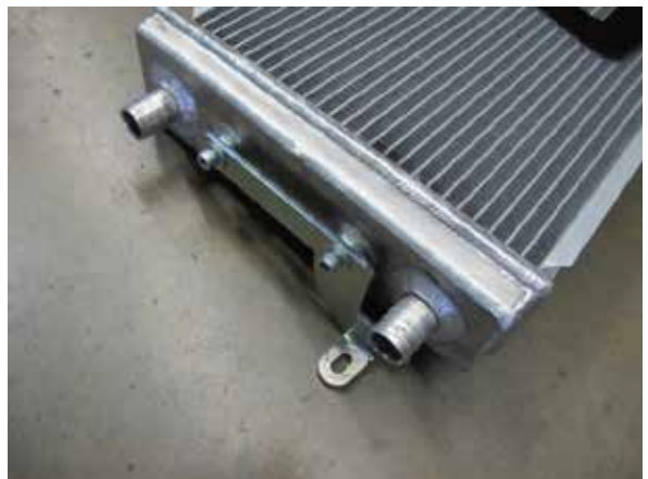
Fig. 7-i: Install passenger side heat exchanger bracket
