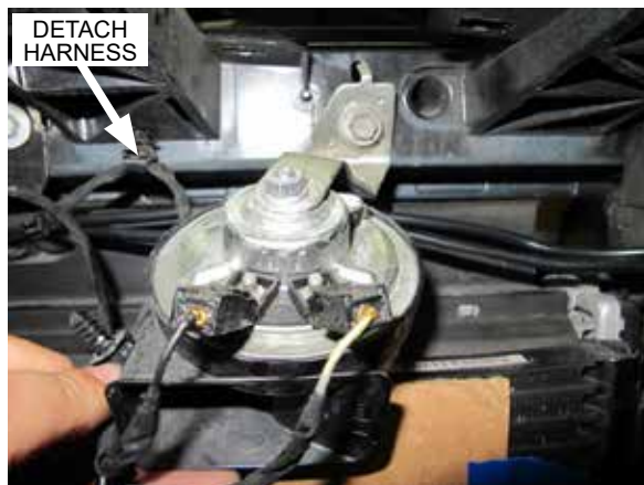
Fig. 7-m: Remove driver side horn
