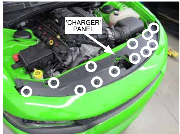
Fig. 2-a: Remove upper front bumper fasteners
