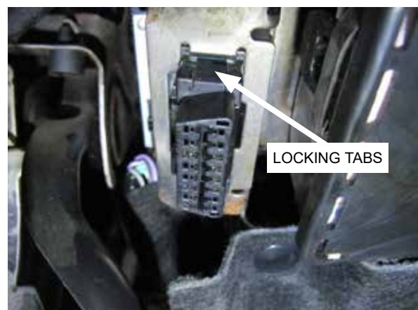
Fig. 13-c: Factory OBD II port locking tabs
