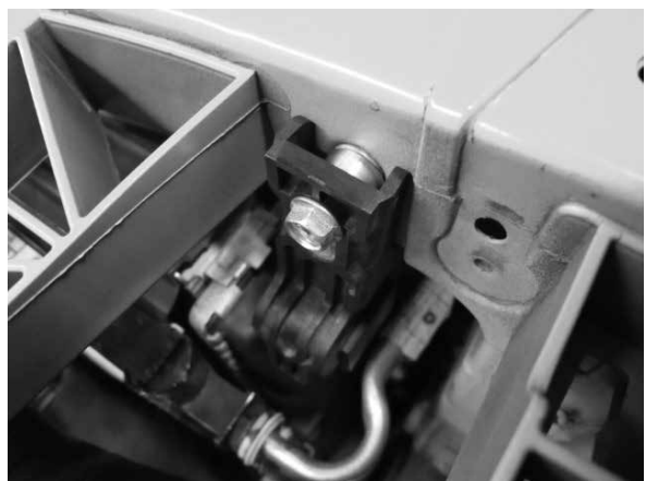
Fig. 7-c: Install upper radiator bracket as shown
