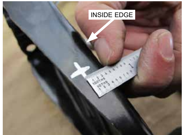
Fig. 4-h: Measure 1/2" from inside edge
