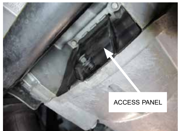
Fig. 3-f: Remove flywheel / flexplate access panel
