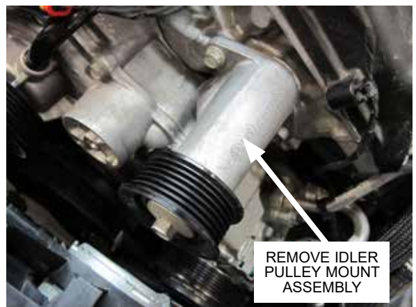
Fig. 2-u: Remove idler pulley mount assembly
