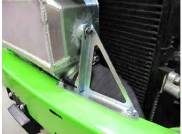
Fig. 7-y: Loosely install driver side air/water cooler support bracket
