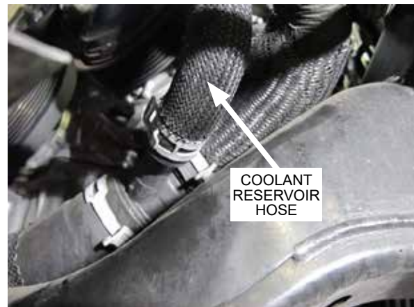
Fig. 5-b: Detach coolant reservoir hose from plastic tee
