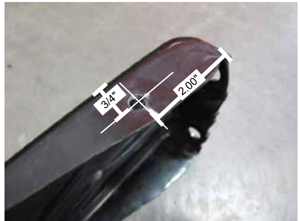
Fig. 4-k: Drill hole on passenger side rear edge of lower radiator support
