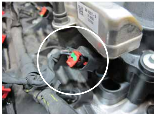
Fig. 10-c: Disconnect fuel injectors
