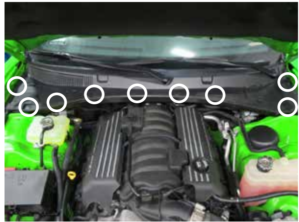
Fig. 1-b: Remove plastic fasteners
