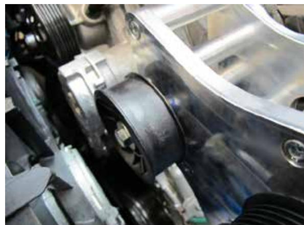
Fig. 6-i: Reinstall serpentine belt idler pulley
