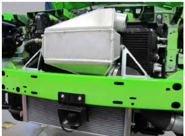
Fig. 7-aa: Install air/water cooler
