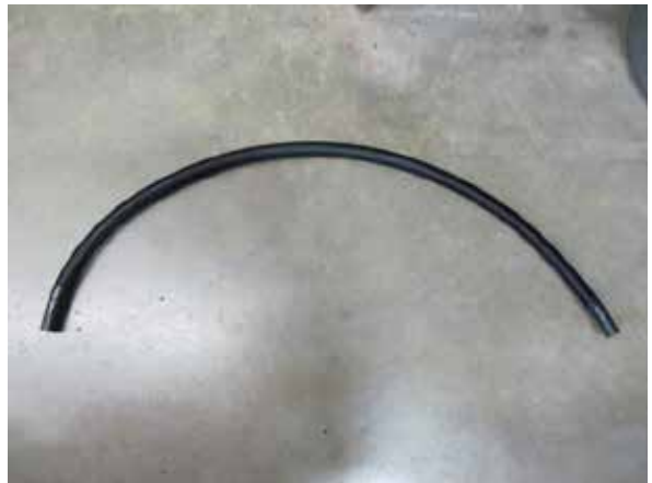
Fig. 9-n: 44" length of the 3/4" coolant hose
