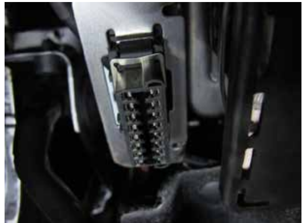
Fig. 13-e: Programming cable OBD II port installed
