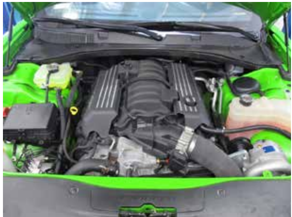
Fig. 12-b: Reinstall both engine covers
