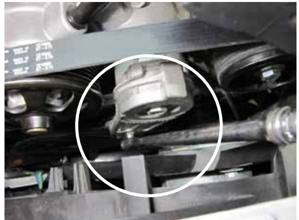
Fig. 2-t: Remove accessory drive belt
