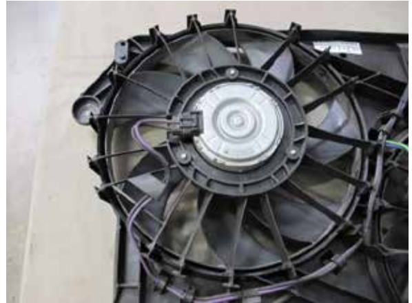
Fig. 4-a: Radiator fan shroud - Driver side
