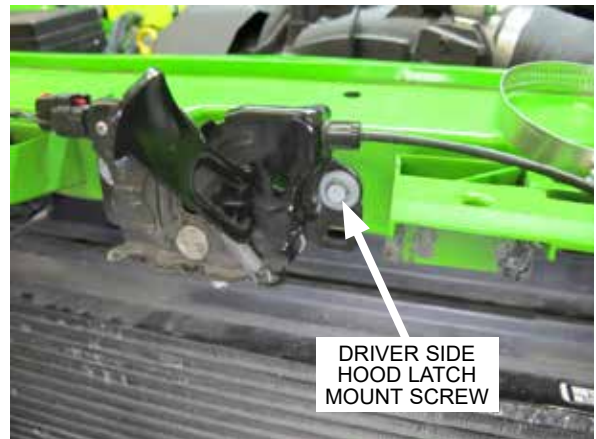
Fig. 7-p: Remove driver side hood latch mount screw
