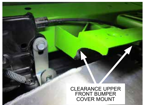
Fig. 7-r: Clearance the front bumper cover mount
