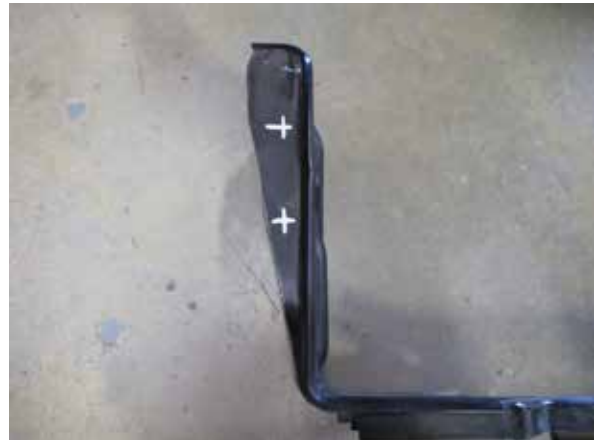
Fig. 4-j: Drill holes on driver side rear edge of lower radiator support
