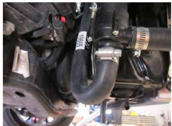
Fig. 9-x: Install coolant hose to electric water pump inlet
