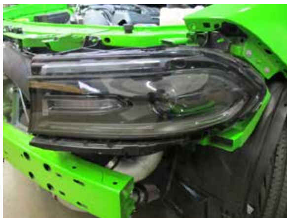
Fig. 7-af: Remove driver side headlight
