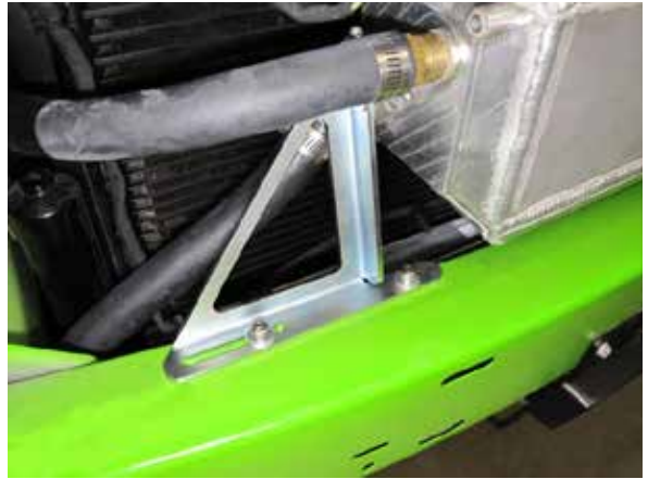
Fig. 7-z: Loosely install passenger side air/water cooler support bracket
