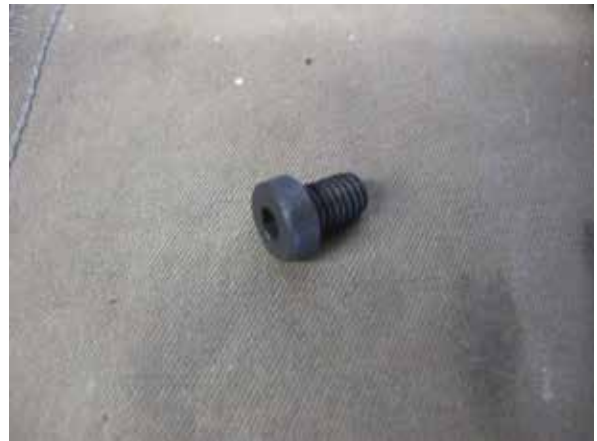
Fig. 9-h: Shorter front bumper support screw
