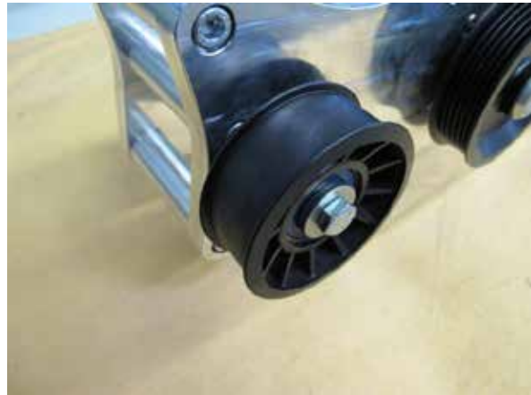
Fig. 6-b: Remove serpentine belt idler pulley
