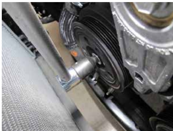
Fig. 3-a: Remove crankshaft damper bolt
