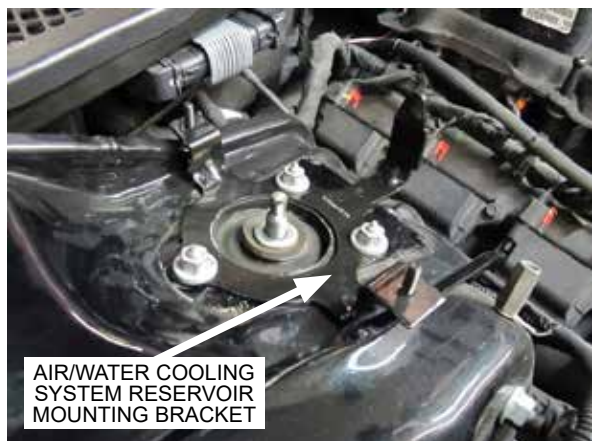
Fig. 9-l: Install air/water cooler system reservoir mount
