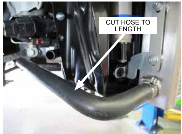
Fig. 9-v: Install 3/4" x 90° hose
