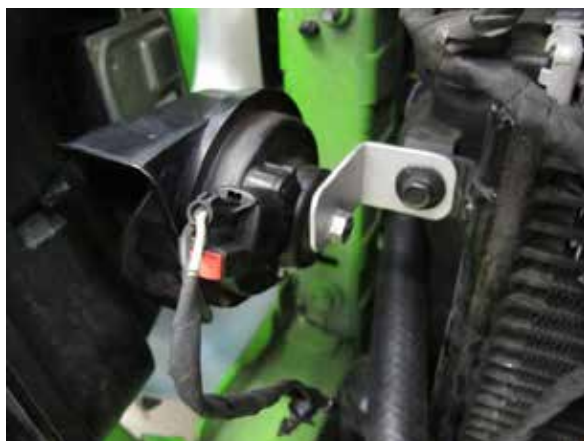
Fig. 7-o: Relocate driver side horn to upper radiator
