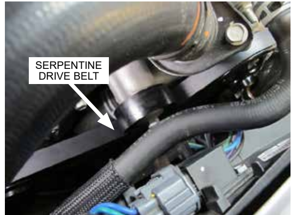
Fig. 6-j: Slide serpentine belt under OEM passenger side smooth idler pulley
