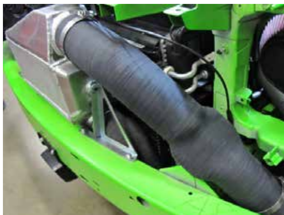
Fig. 7-ag: Install discharge sleeve 'B'
