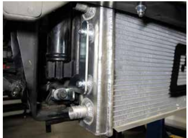
Fig. 7-k: Install passenger side of heat exchanger assembly
