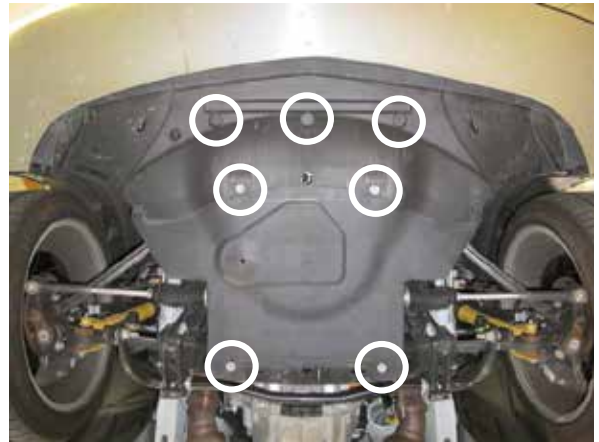
Fig. 2-d: Remove engine service panel fasteners
