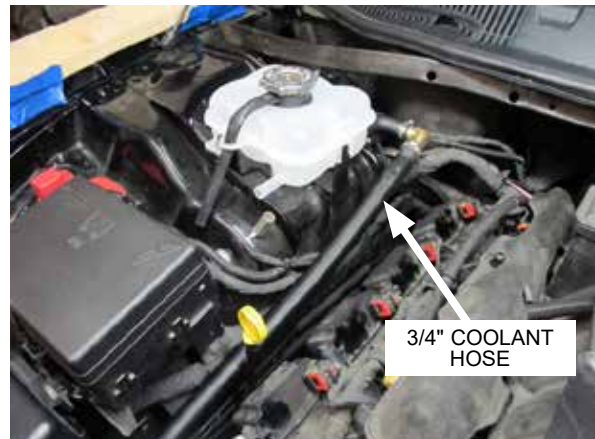
Fig. 9-s: Route 3/4" coolant hose towards air/water cooler
