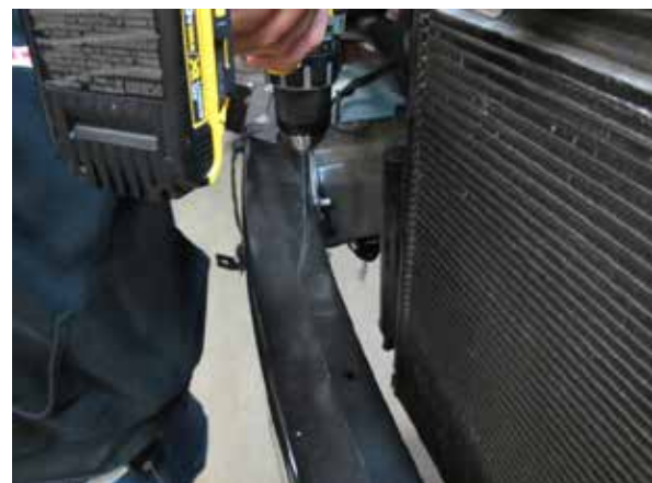
Fig. 7-u: Drill holes in front bumper support
