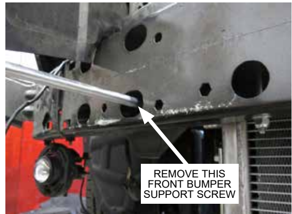
Fig. 9-g: Remove front bumper support screw
