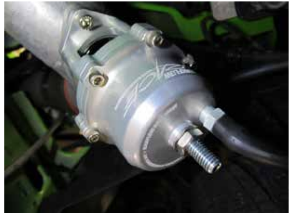
Fig. 8-j: Attach vacuum hose to bypass valve
