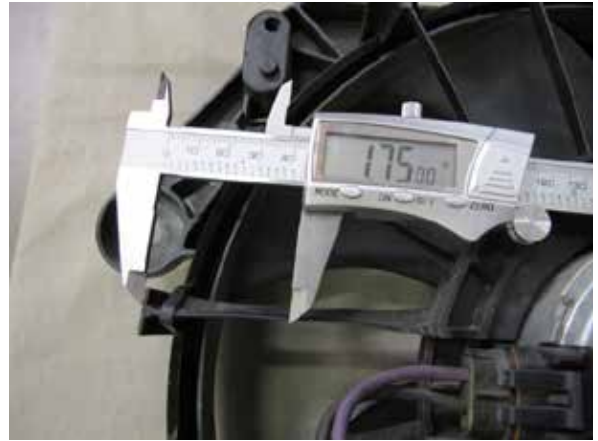
Fig. 4-b: Measure 1.75" from outer edge
