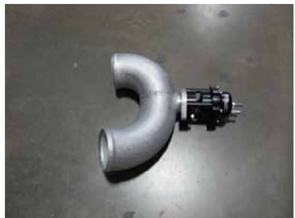
Fig. 7-aj: Assemble discharge tube 'A' as shown
