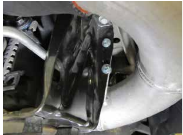
Fig. 7-ac: Secure discharge tube 'D' to lower radiator support
