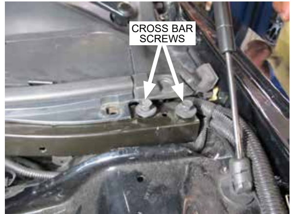
Fig. 1-d: Remove cross bar screws
