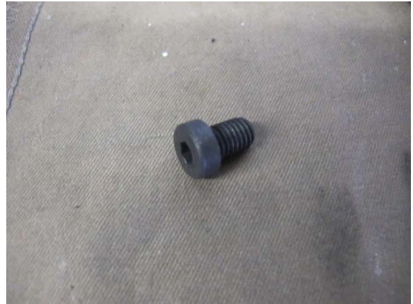
Fig. 9-h: Shorter front bumper support screw
