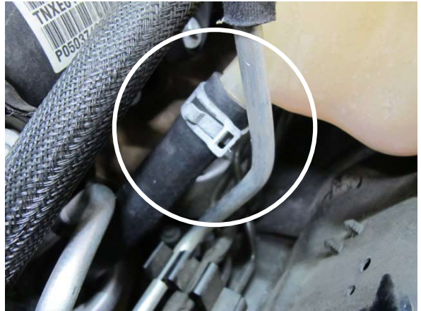
Fig. 5-g: Attach coolant hose to coolant reservoir
