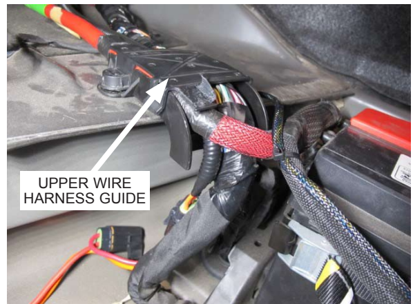
Fig. 11-q: Secure fuel pump booster adapter harness
