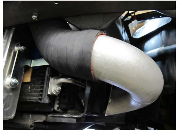
Fig. 7-ab: Loosely install discharge tube 'D'
