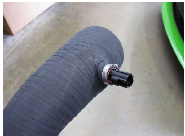
Fig. 7-ad: Install IAT sensor to molded boss on discharge sleeve 'E'
