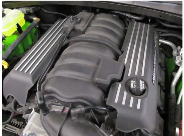
Fig. 10-a: Remove engine covers
