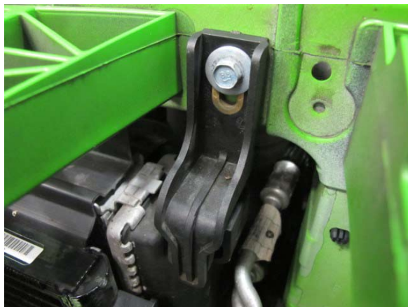
Fig. 7-a: Remove upper radiator bracket
