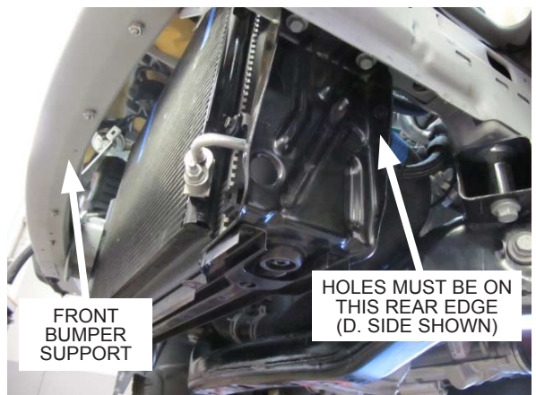
Fig. 4-i: Reinstall lower radiator support
