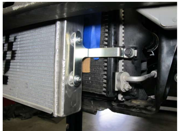
Fig. 7-l: Install driver side of heat exchanger assembly
