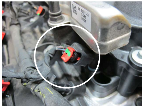
Fig. 10-c: Disconnect fuel injectors
