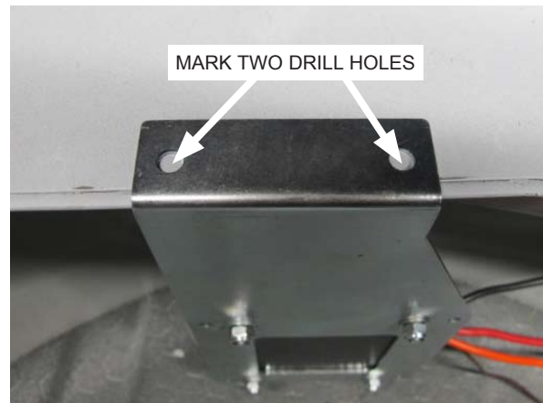
Fig. 11-b: Mark two drill holes
