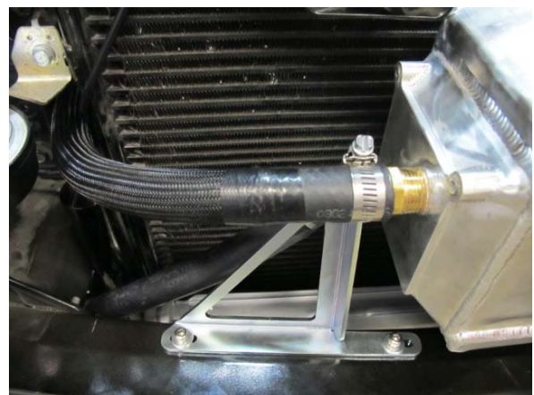
Fig. 9-u: Attach 3/4" coolant hose to air/water cooler
