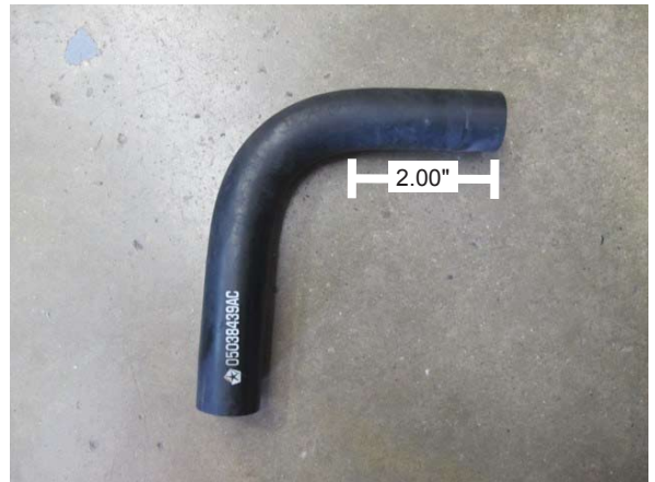
Fig. 8-e: Modify OEM breather hose
