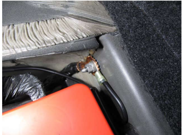
Fig. 11-h: Attach ground strap to grounding stud
