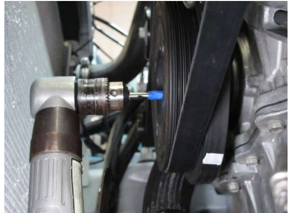
Fig. 3-d: Drill crankshaft / damper assembly
