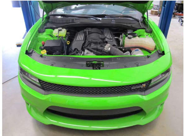
Fig. 12-a: Reinstall front bumper cover
