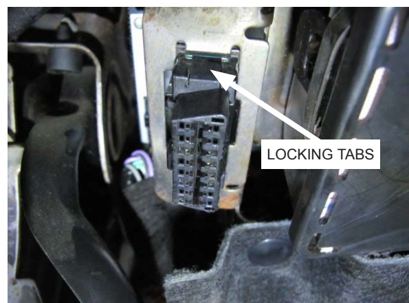
Fig. 13-c: Factory OBD II port locking tabs
