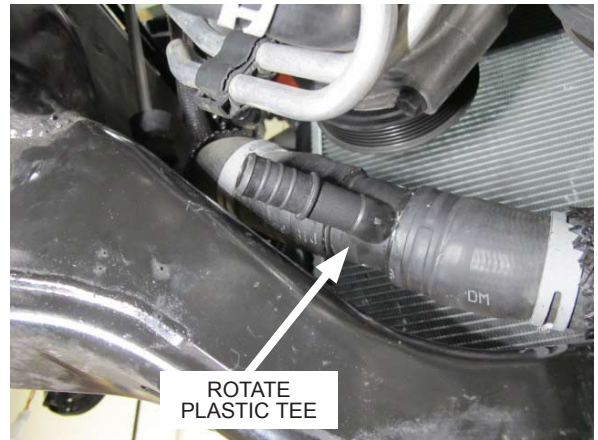
Fig. 5-d: Rotate plastic tee 180° clockwise
