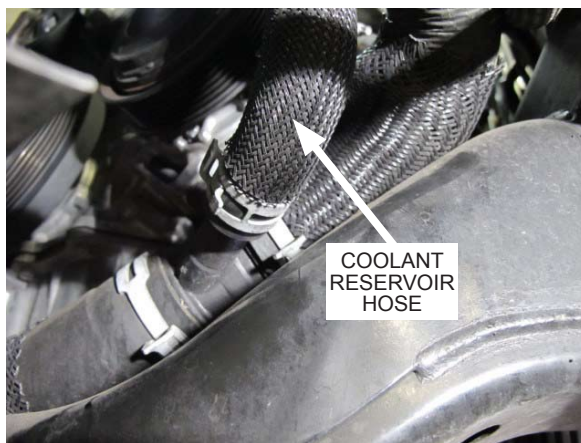
Fig. 5-b: Detach coolant reservoir hose from plastic tee
