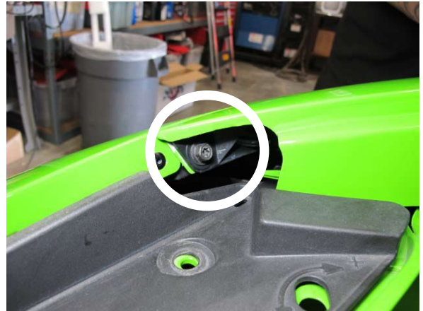
Fig. 2-g: Remove each upper front bumper cover screw
