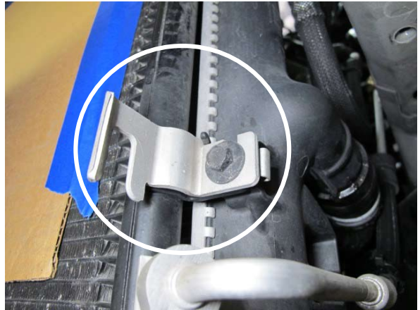
Fig. 7-g: Remove aluminum bracket and screw
