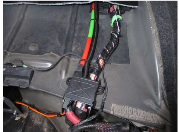
Fig. 11-p: Route the fuel pump booster adapter harness along the large power wire
