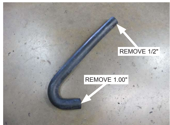
Fig. 9-i: Modify 150° molded hose as shown
