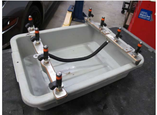
Fig. 10-g: Install provided high-flow injectors
