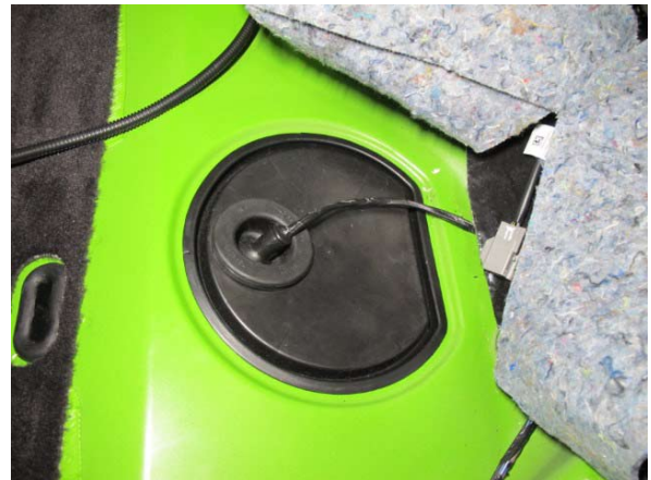
Fig. 11-k: Remove fuel pump access panel
