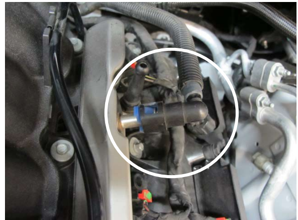
Fig. 10-e: Disconnect fuel feed line
