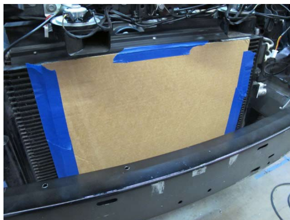
Fig. 7-f: Cover A/C condenser with cardboard
