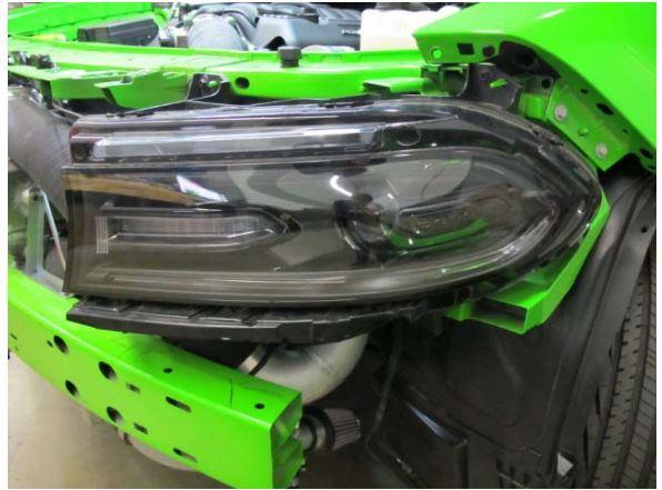
Fig. 7-af: Remove driver side headlight
