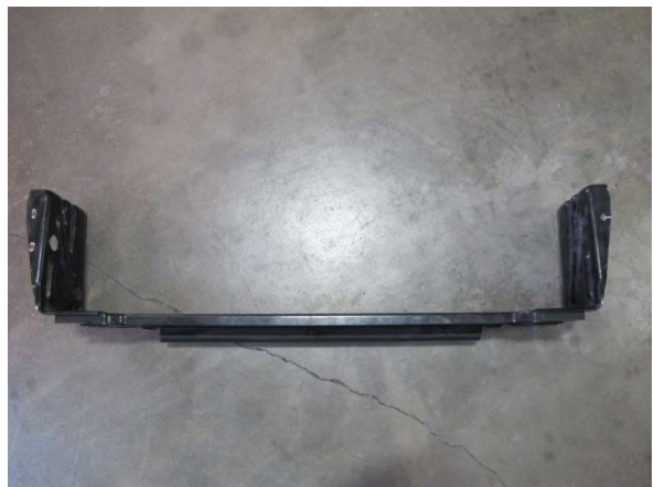
Fig. 4-c: Lower radiator support
