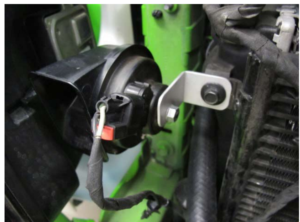
Fig. 7-o: Relocate driver side horn to upper radiator
