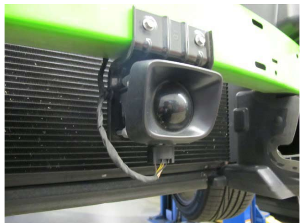
Fig. 2-i: Disconnect adaptive cruise control sensor
