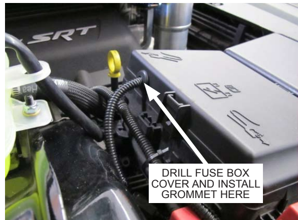
Fig. 9-b: Drill fuse box cover, install grommet and route wire into fuse box
