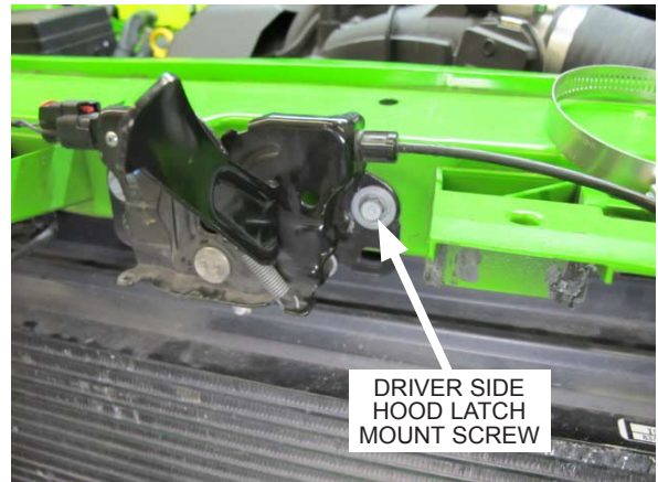
Fig. 7-p: Remove driver side hood latch mount screw
