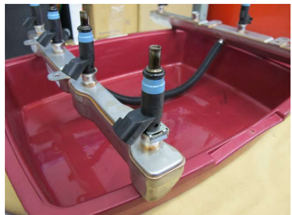
Fig. 10-f: Remove OEM fuel injectors
