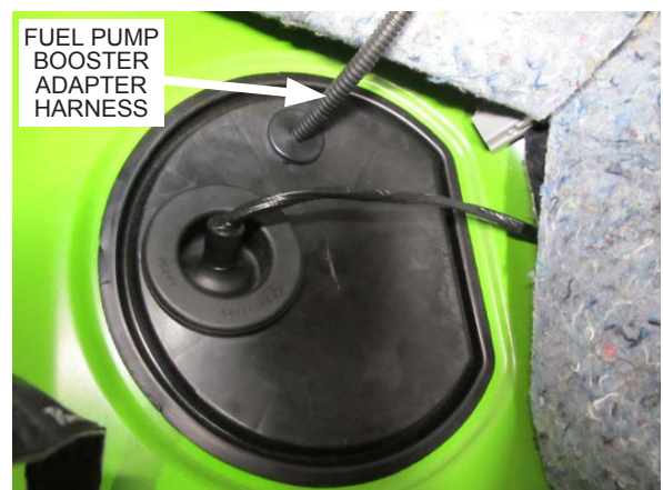
Fig. 11-o: Reinstall fuel pump access panel
