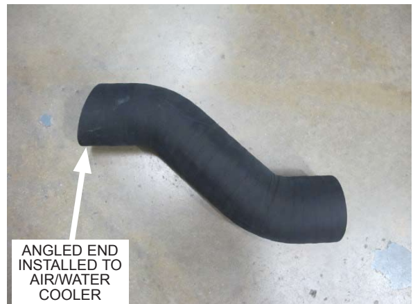
Fig. 7-v: Discharge sleeve 'C'
