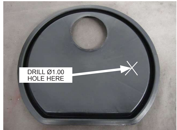
Fig. 11-m: Modify fuel pump access panel
