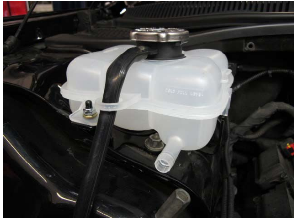
Fig. 9-m: Install air/water cooler system reservoir to mount
