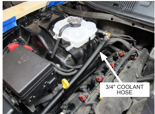
Fig. 9-s: Route 3/4" coolant hose towards air/water cooler
