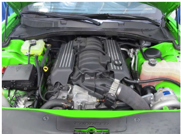
Fig. 12-c: Reinstall both engine covers
