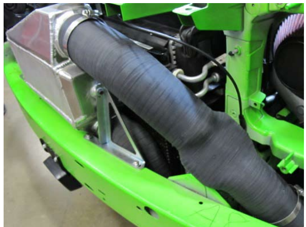
Fig. 7-ag: Install discharge sleeve 'B'
