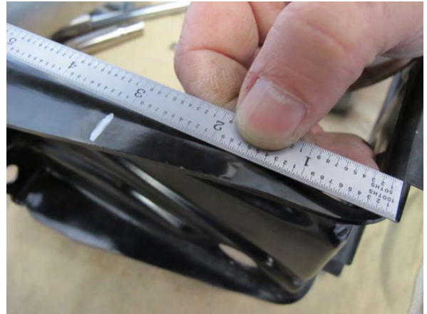
Fig. 4-d: Measure 3.25" from bottom edge
