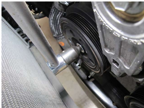
Fig. 3-a: Remove crankshaft damper bolt
