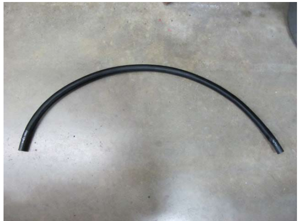
Fig. 9-n: 44" length of the 3/4" coolant hose
