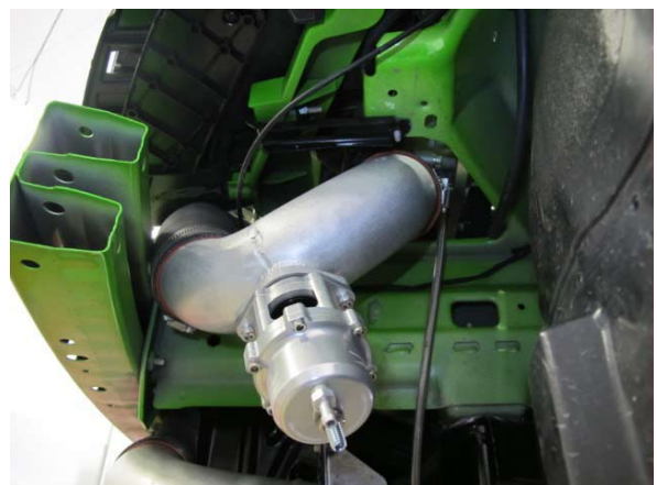
Fig. 7-aj: Loosely install discharge tube 'A' to discharge tube 'B'
