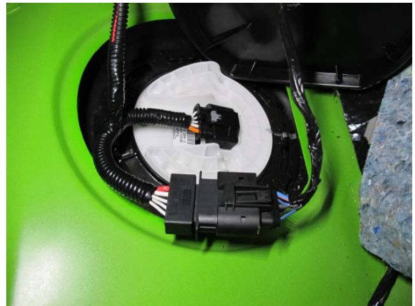
Fig. 11-n: Install fuel pump booster harness
