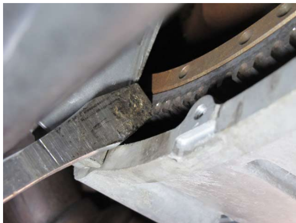
Fig. 3-g: Lock engine in position
