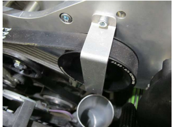
Fig. 6-j: Reinstall pulley guard
