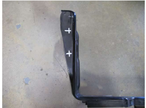
Fig. 4-g: Drill holes on driver side rear edge of lower radiator support
