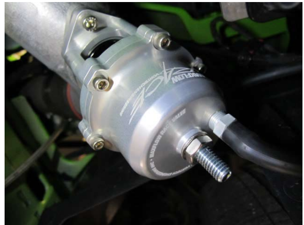
Fig. 8-k: Attach vacuum hose to bypass valve
