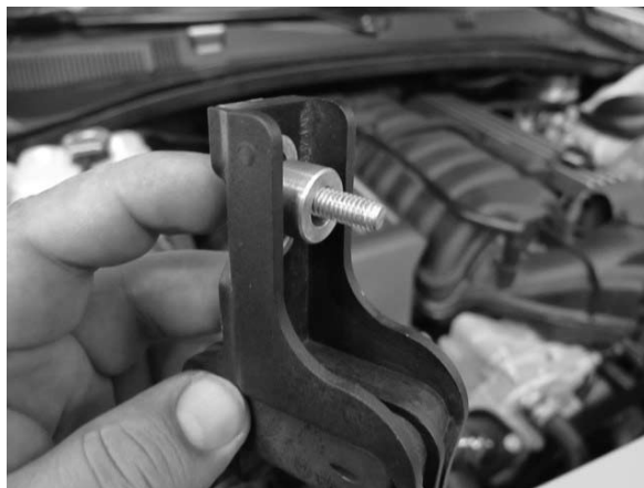
Fig. 7-b: Assemble hardware and spacer as shown
