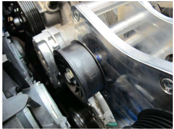
Fig. 6-h: Reinstall serpentine belt idler pulley
