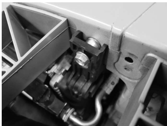
Fig. 7-c: Install upper radiator bracket as shown
