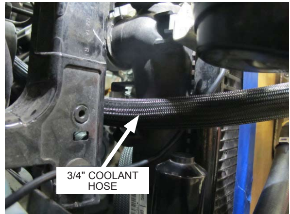
Fig. 9-t: Pass 3/4" coolant hose between radiator and core support
