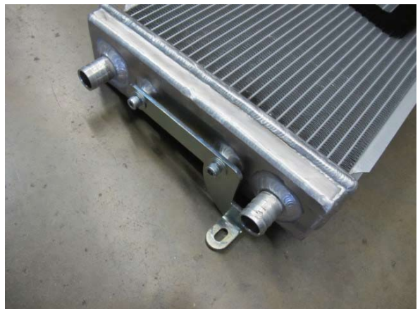
Fig. 7-i: Install passenger side heat exchanger bracket
