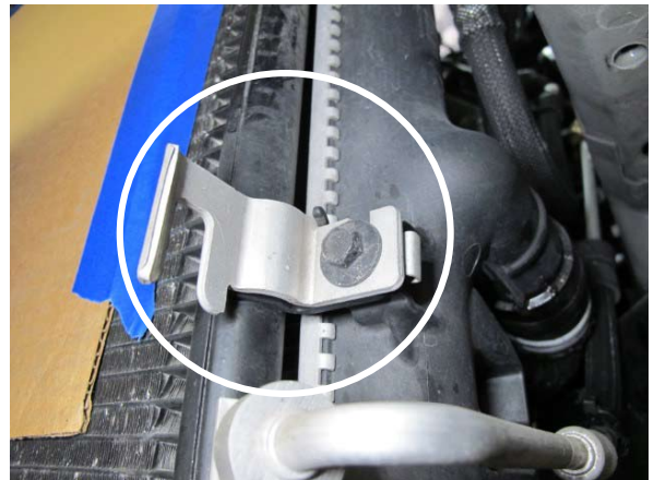
Fig. 7-d: Remove aluminum bracket and screw
