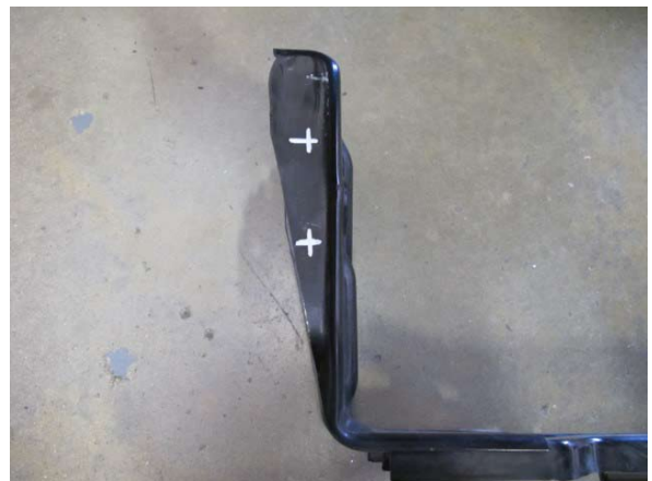
Fig. 4-i: Drill holes on driver side rear edge of lower radiator support
