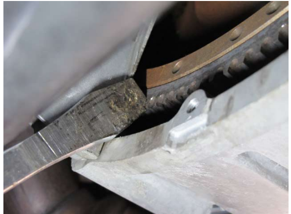
Fig. 3-g: Lock engine in position
