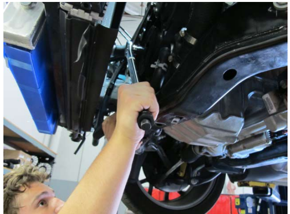
Fig. 3-h: Torque crank bolt
