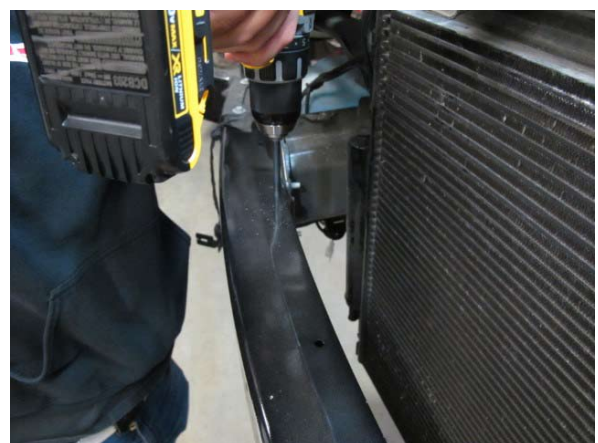
Fig. 7-r: Drill holes in front bumper support
