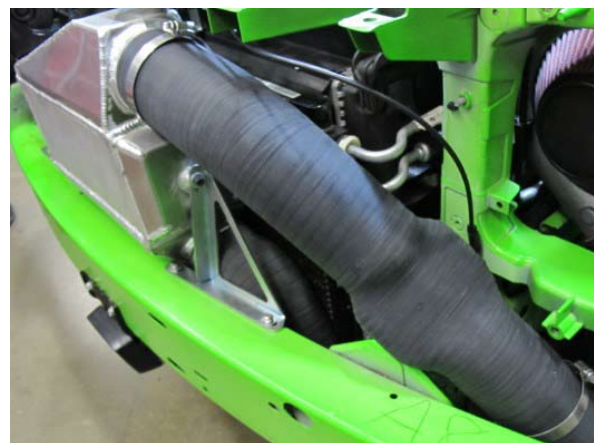
Fig. 7-ad: Install discharge sleeve 'B'
