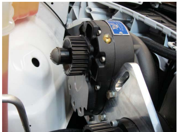
Fig. 8-c: Install supercharger to supercharger mounting bracket assembly
