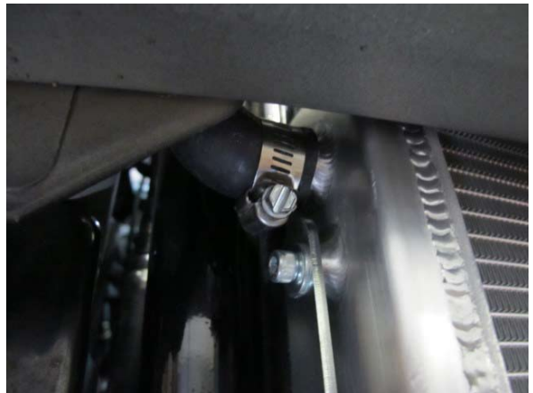
Fig. 9-j: Install short end of 150° molded hose to heat exchanger
