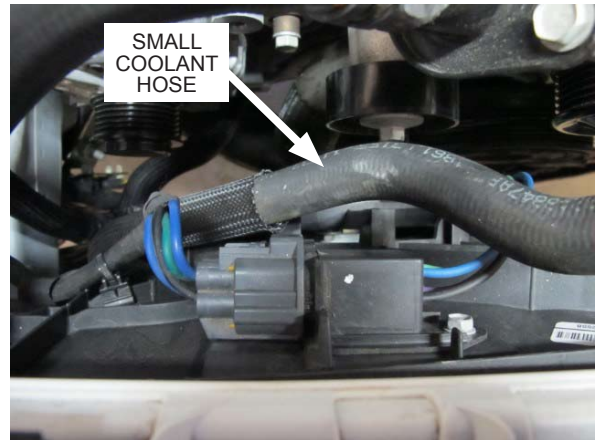
Fig. 2-p: Detach coolant hose and unplug radiator fan connector
