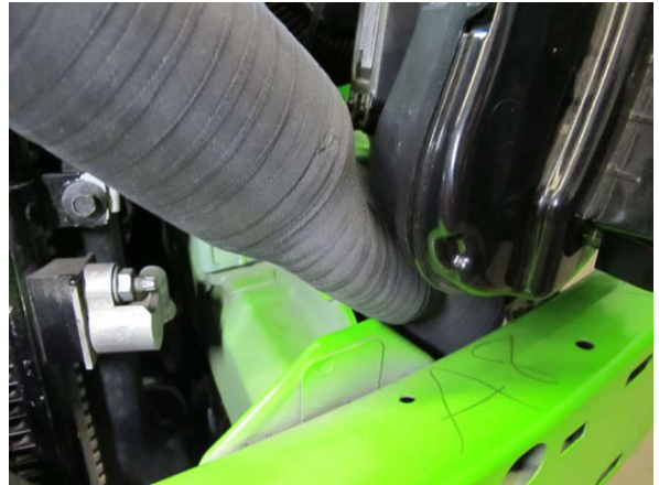
Fig. 7-ae: Adjust discharge sleeve 'B' and install driver side headlight
