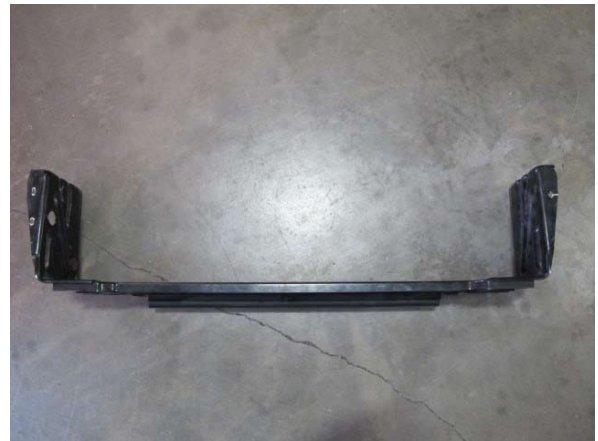
Fig. 4-e: Lower radiator support
