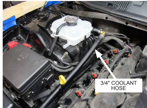
Fig. 9-s: Route 3/4" coolant hose towards air/water cooler
