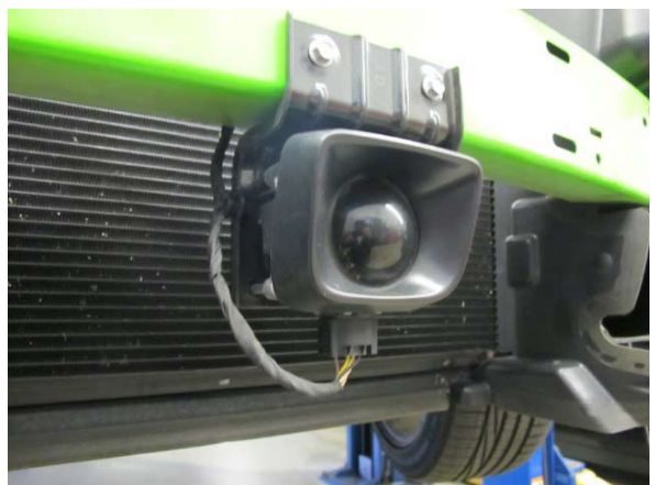
Fig. 2-i: Disconnect adaptive cruise control sensor
