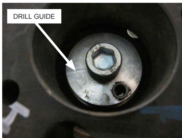
Fig. 3-b: Install drill guide
