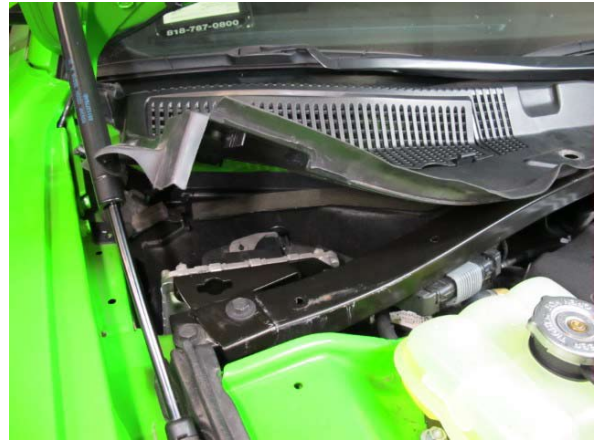
Fig. 1-d: Lift up passenger side of windshield cowl
