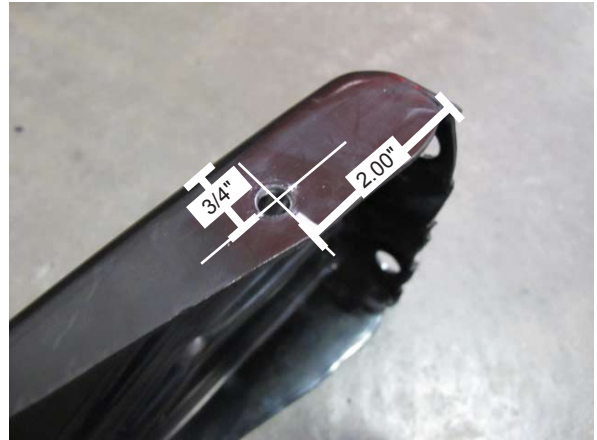
Fig. 4-j: Drill hole on passenger side rear edge of lower radiator support
