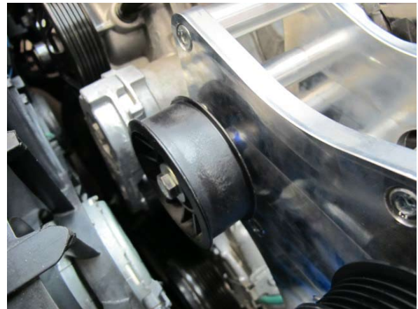
Fig. 6-h: Reinstall serpentine belt idler pulley
