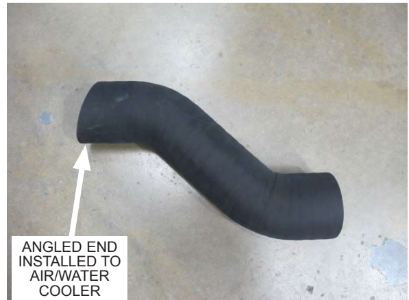
Fig. 7-s: Discharge sleeve 'C'
