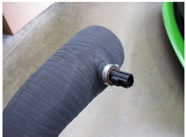
Fig. 7-aa: Install IAT sensor to molded boss on discharge sleeve 'E'
