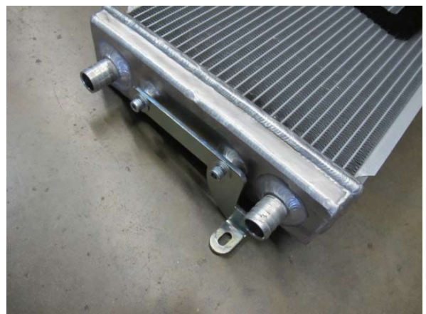
Fig. 7-f: Install passenger side heat exchanger bracket
