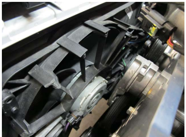
Fig. 4-c: Reinstall radiator fan assembly
