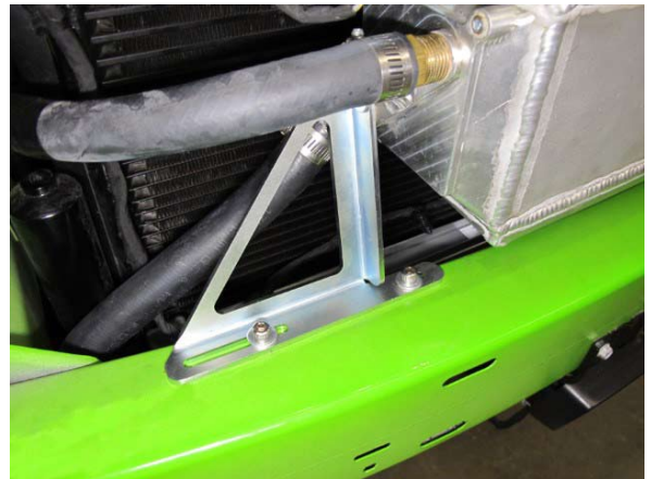
Fig. 7-w: Loosely install passenger side air/water cooler support bracket
