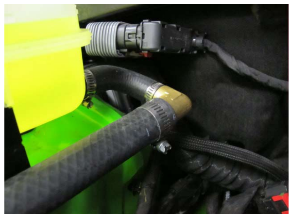
Fig. 9-r: Attach 44" length of 3/4" coolant hose to the brass fitting as shown
