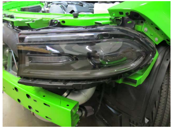
Fig. 7-ac: Remove driver side headlight
