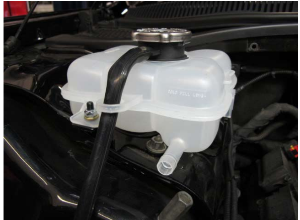
Fig. 9-m: Install air/water cooler system reservoir to mount
