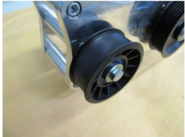
Fig. 6-b: Remove serpentine belt idler pulley
