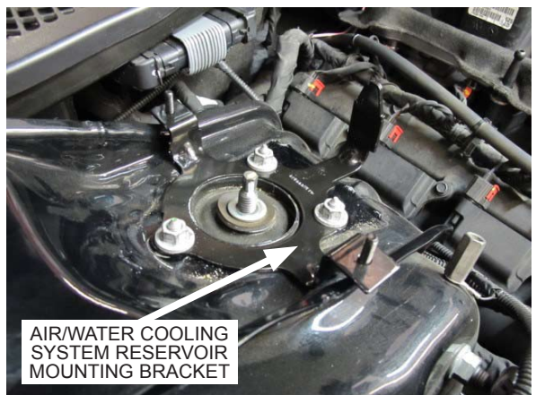
Fig. 9-l: Install air/water cooler system reservoir mount
