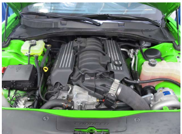
Fig. 10-c: Reinstall both engine covers
