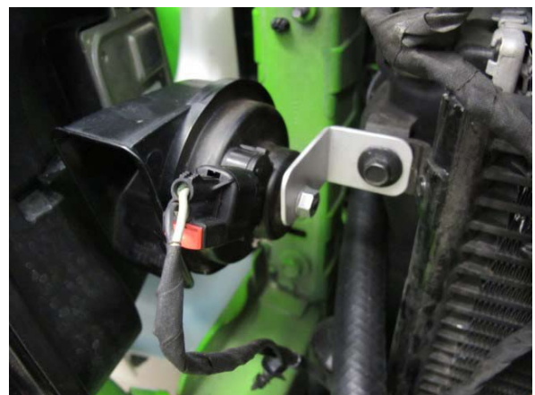
Fig. 7-l: Relocate driver side horn to upper radiator
