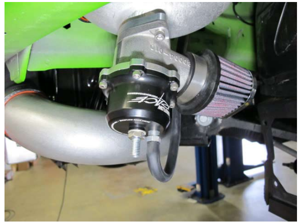
Fig. 8-k: Attach vacuum hose to bypass valve
