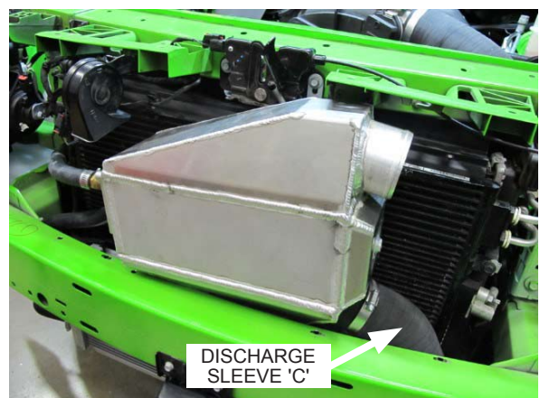
Fig. 7-u: Loosely install upper air/water cooler support bracket and air/water cooler
