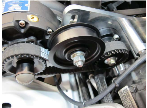
Fig. 8-d: Tension cog belt
