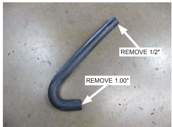
Fig. 9-i: Modify 150° molded hose as shown
