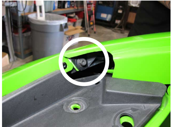
Fig. 2-g: Remove each upper front bumper cover screw
