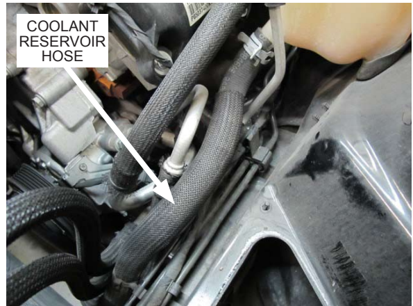
Fig. 5-a: Detach coolant reservoir hose from bottom side of coolant reservoir
