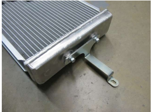
Fig. 7-g: Install driver side heat exchanger bracket
