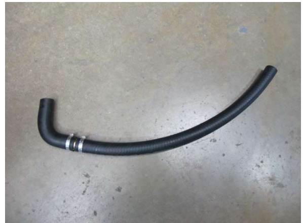
Fig. 5-e: Assemble new coolant reservoir hose as shown
