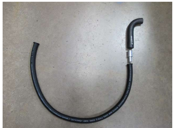
Fig. 8-f: Breather hose assembly
