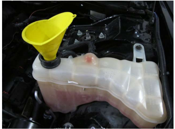
Fig. 5-h: Close coolant drain valve and refill engine coolant system
