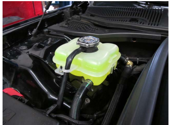
Fig. 9-z: Fill air/water cooling system with 50/50 water/coolant mix
