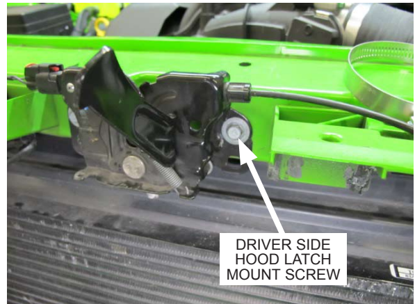
Fig. 7-m: Remove driver side hood latch mount screw
