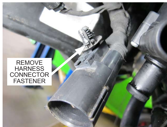
Fig. 9-e: Remove plastic harness connector fastener
