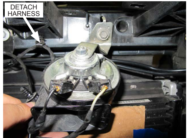
Fig. 7-j: Remove driver side horn
