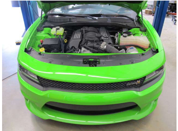
Fig. 10-a: Reinstall front bumper cover
