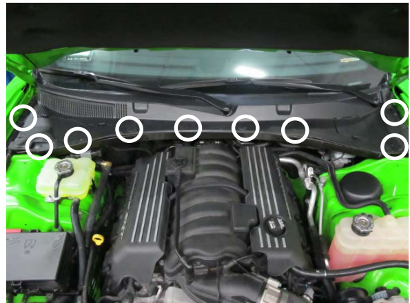
Fig. 1-b: Remove plastic fasteners
