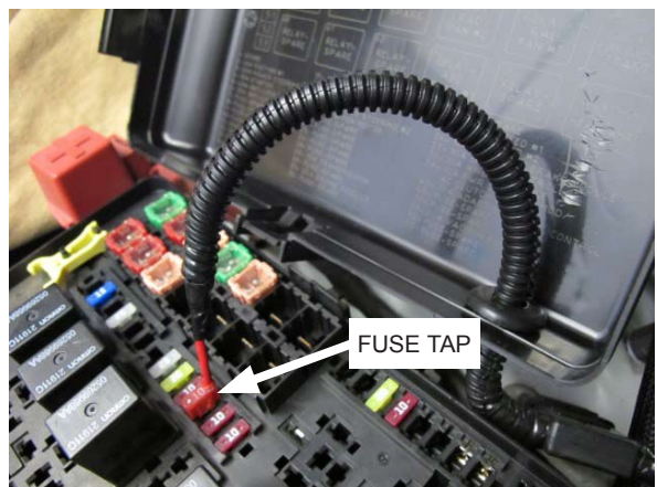
Fig. 9-c: Install fuse from water pump harness as shown
