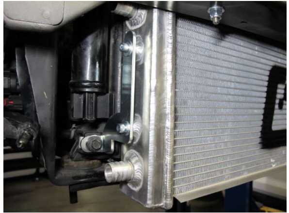
Fig. 7-h: Install passenger side of heat exchanger assembly
