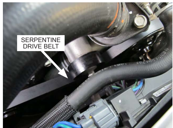
Fig. 6-i: Slide serpentine belt under OEM passenger side smooth idler pulley
