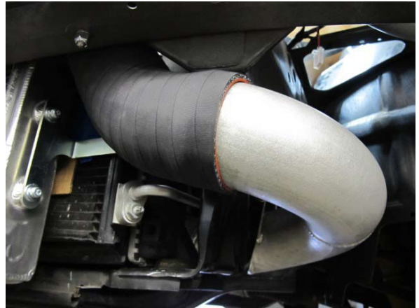
Fig. 7-y: Loosely install discharge tube 'D'
