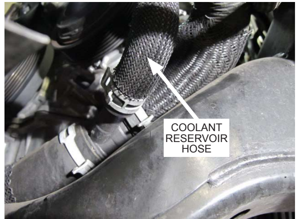
Fig. 5-b: Detach coolant reservoir hose from plastic tee
