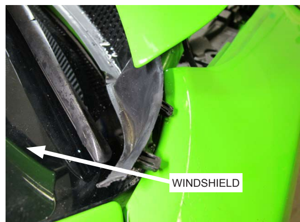
Fig. 1-c: Detach windshield cowl from passenger side fender
