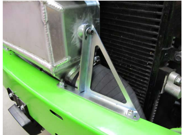
Fig. 7-v: Loosely install driver side air/water cooler support bracket
