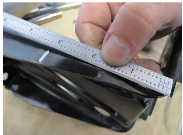
Fig. 4-f: Measure 3.25" from bottom edge
