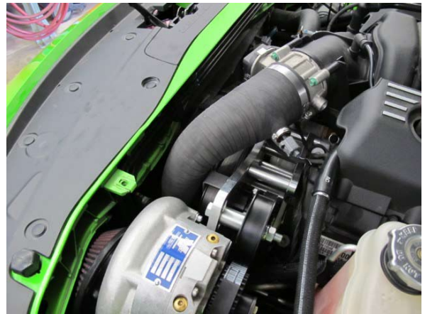
Fig. 7-ab: Install discharge sleeve 'E' and reconnect IAT sensor
