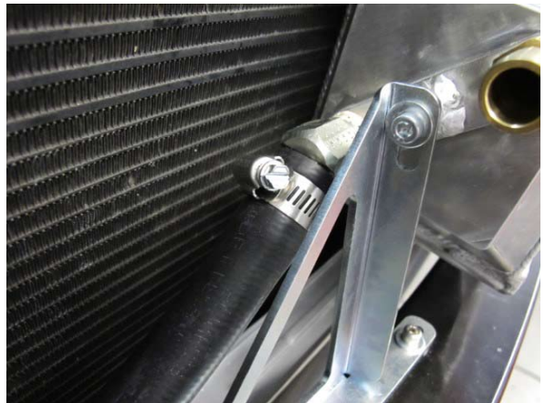
Fig. 9-k: Install long end of 150° molded hose to air/water cooler
