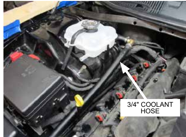
Fig. 9-s: Route 3/4" coolant hose towards air/water cooler
