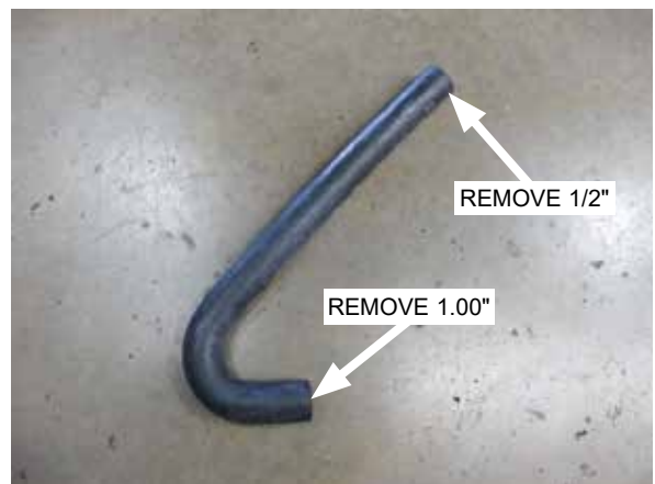
Fig. 9-i: Modify 150° molded hose as shown
