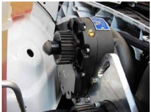
Fig. 8-c: Install supercharger to supercharger mounting bracket assembly
