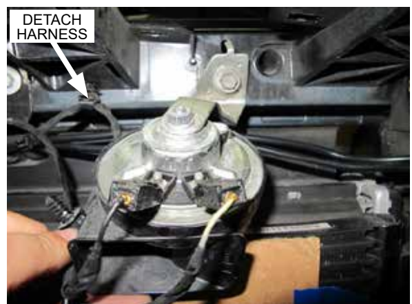
Fig. 7-l: Remove driver side horn
