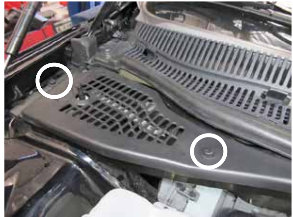
Fig. 1-d: Remove two plastic fasteners
