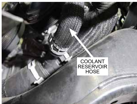
Fig. 5-b: Detach coolant reservoir hose from plastic tee
