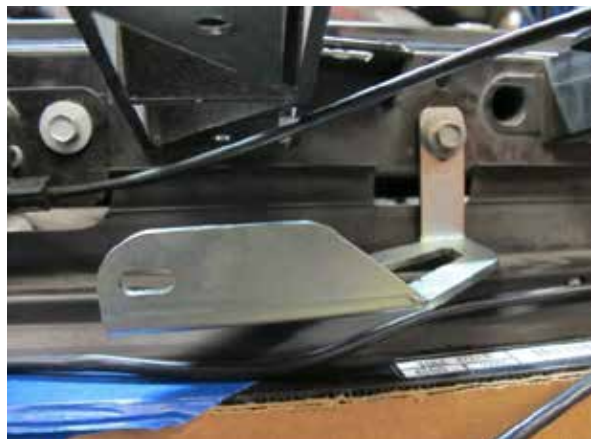
Fig. 7-o: Install upper air/water cooler support bracket
