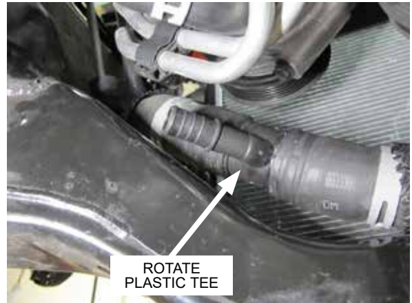
Fig. 5-d: Rotate plastic tee 180° clockwise
