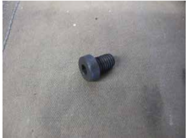
Fig. 9-h: Shorter front bumper support screw
