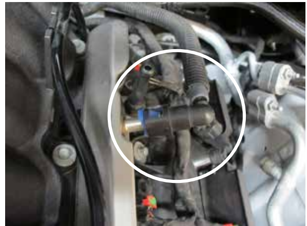
Fig. 11-e: Disconnect fuel feed line
