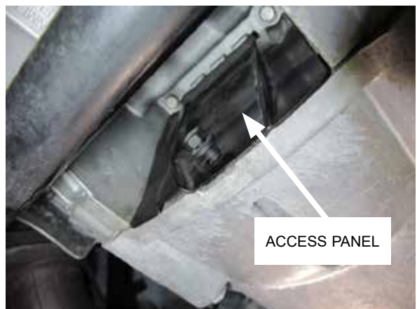
Fig. 3-f: Reinstall flywheel / flexplate access panel
