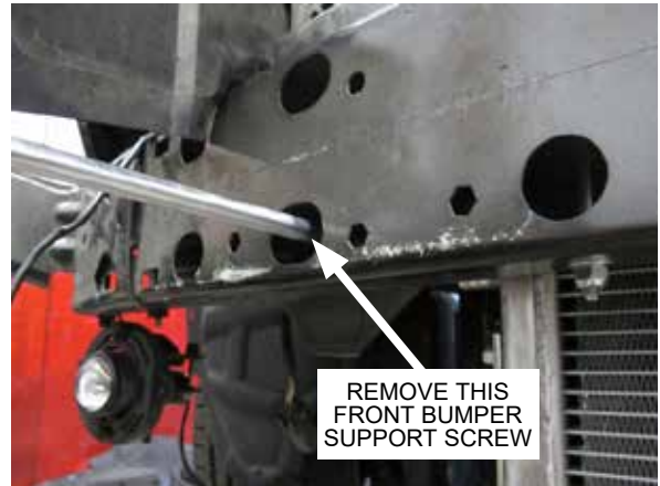
Fig. 9-g: Remove front bumper support screw
