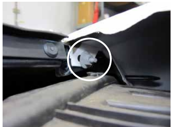
Fig. 2-f: Remove two nuts
