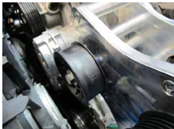
Fig. 6-i: Reinstall serpentine belt idler pulley
