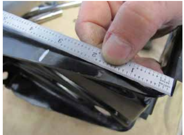
Fig. 4-d: Measure 3.25" from bottom edge
