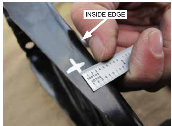
Fig. 4-e: Measure 1/2" from inside edge
