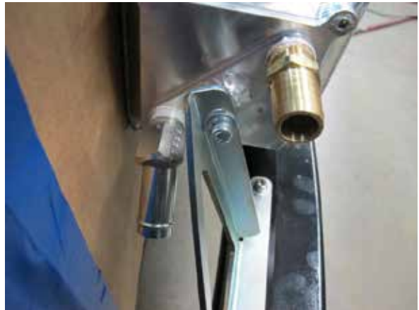
Fig. 7-s: Temporarily secure passenger side of air/water cooler
