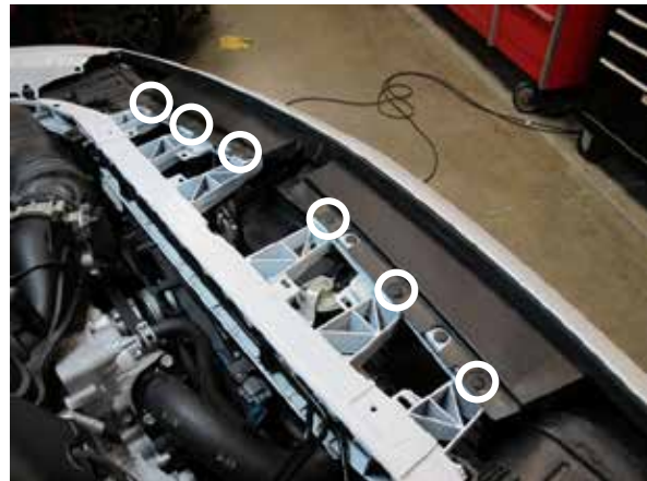
Fig. 2-b: Remove six plastic fasteners
