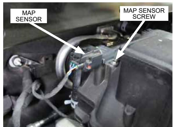
Fig. 11-i: Install 3-Bar MAP sensor
