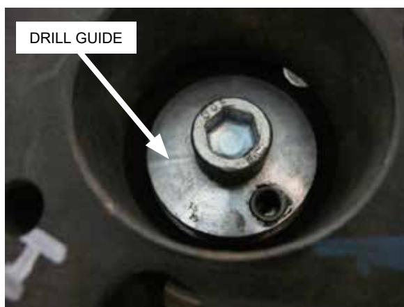
Fig. 3-b: Install drill guide
