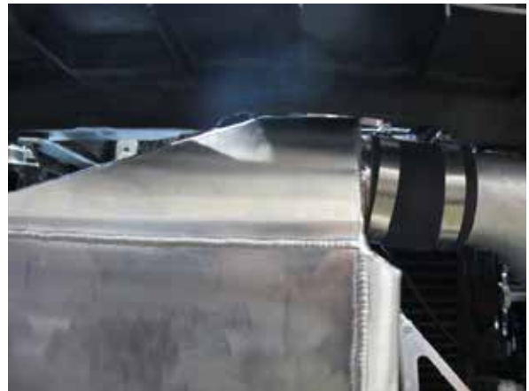
Fig. 10-e: Modified radiator shroud to air/water cooler clearance
