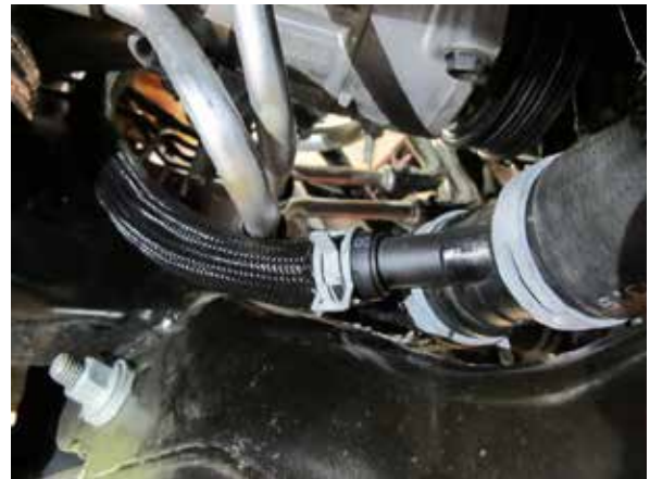
Fig. 5-e: Assemble new coolant reservoir hose as shown
