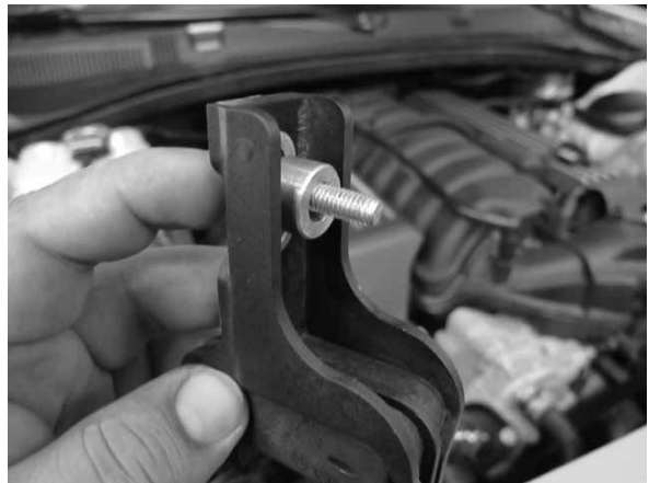
Fig. 7-b: Assemble hardware and spacer as shown
