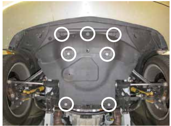
Fig. 2-e: Remove splash guard
