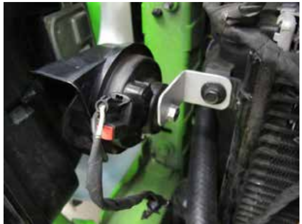
Fig. 7-n: Relocate driver side horn to upper radiator
