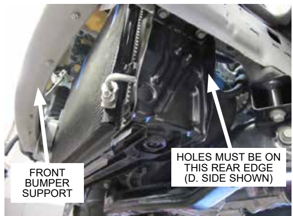
Fig. 4-i: Reinstall lower radiator support
