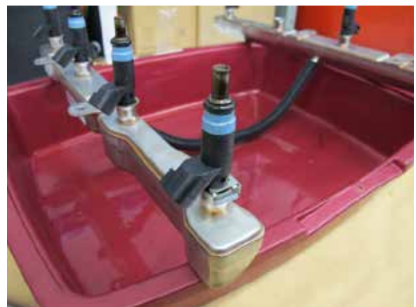
Fig. 11-f: Remove OEM fuel injectors
