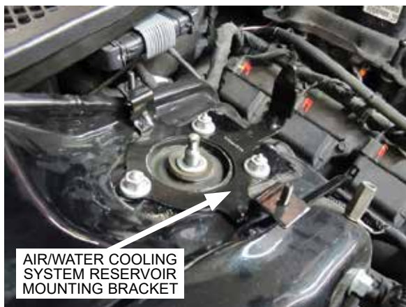
Fig. 9-l: Install air/water cooler system reservoir mount
