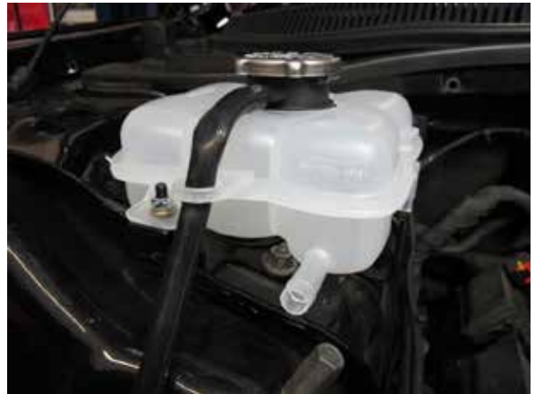
Fig. 9-m: Install air/water cooler system reservoir to mount
