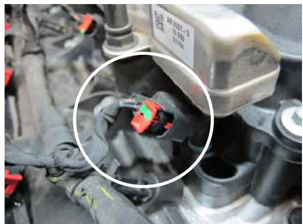
Fig. 11-c: Disconnect fuel injectors
