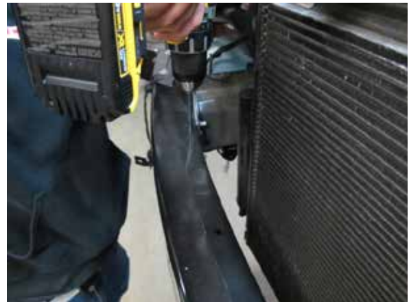
Fig. 7-q: Drill through two holes on front bumper support
