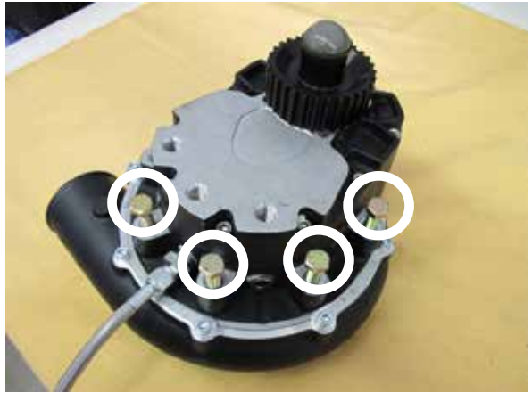
Fig. 8-b: Lubricate supercharger mounting boss threads
