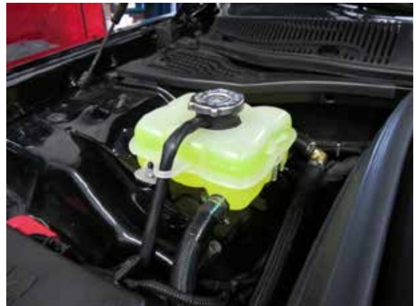
Fig. 9-z: Fill air/water cooling system with 50/50 water/coolant mix
