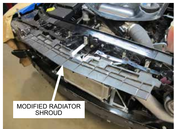
Fig. 10-f: Secure modified radiator shroud and three radiator shroud brackets
