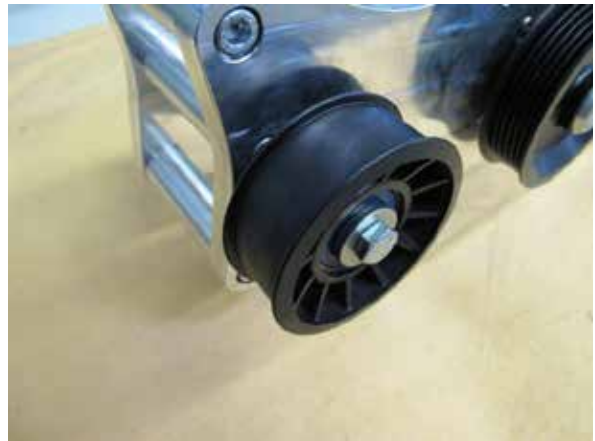
Fig. 6-b: Remove serpentine belt idler pulley
