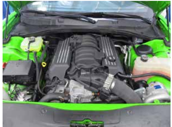
Fig. 13-d: Reinstall both engine covers
