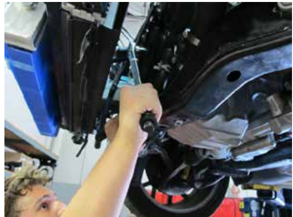
Fig. 3-h: Torque crank bolt
