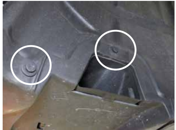
Fig. 2-d: Remove two plastic fasteners
