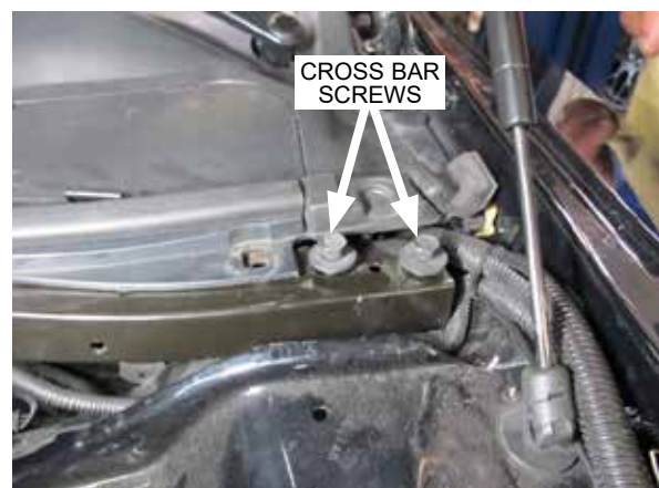
Fig. 1-c: Remove cross bar screws
