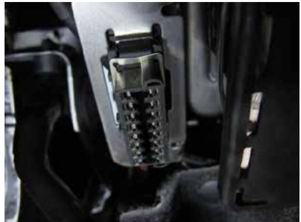
Fig. 14-e: Programming cable OBD II port installed
