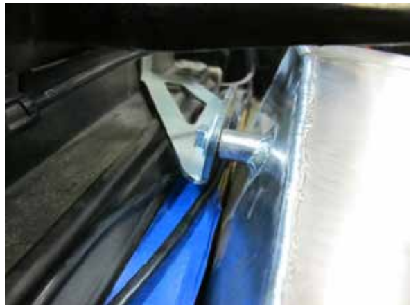
Fig. 7-t: Temporarily secure top side of air/water cooler
