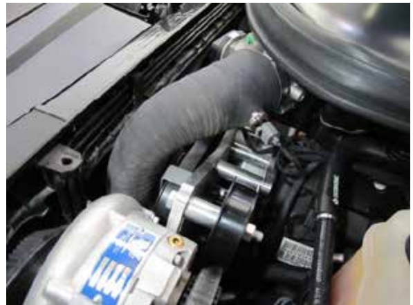
Fig. 7-ac: Install discharge sleeve 'E' and reconnect IAT sensor
