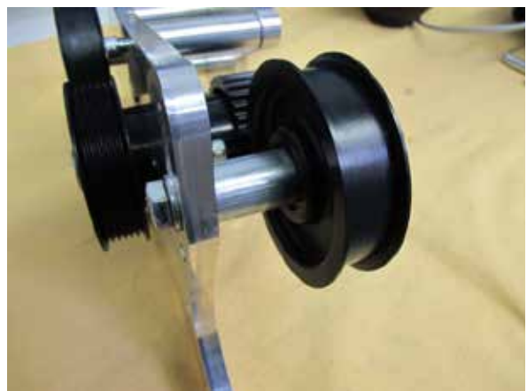
Fig. 6-c: Remove cog belt idler pulley
