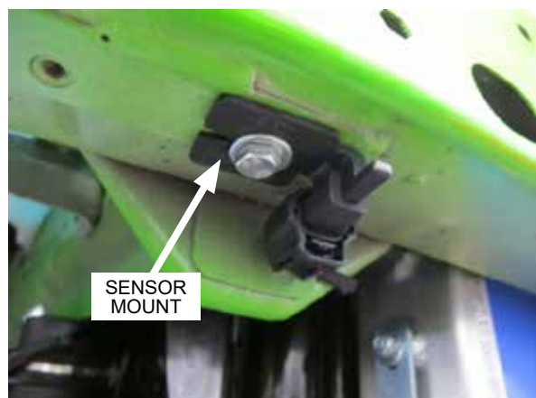
Fig. 7-ag: Reinstall ambient air temperature sensor as shown
