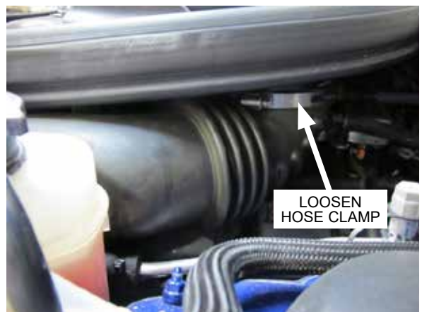
Fig. 2-o: Loosen hose clamp
