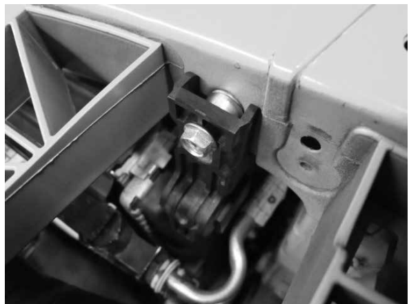
Fig. 7-c: Install upper radiator bracket as shown
