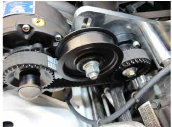
Fig. 8-d: Tension cog belt
