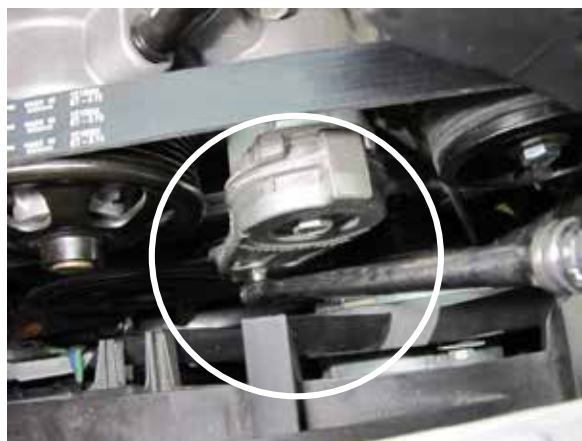
Fig. 2-x: Remove accessory drive belt
