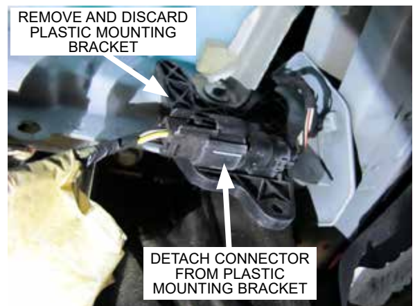
Fig. 2-i: Disconnect fog light connector
