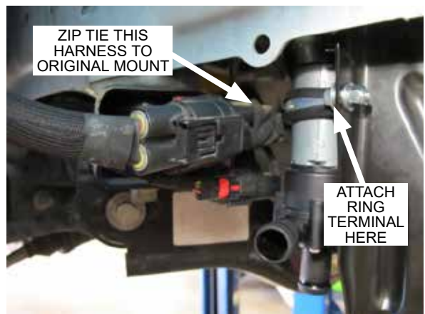
Fig. 9-f: Install the auxiliary water pump
