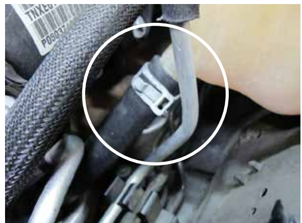
Fig. 5-f: Attach coolant hose to coolant reservoir
