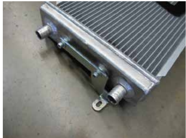
Fig. 7-h: Install passenger side heat exchanger bracket
