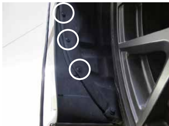
Fig. 2-c: Drill through and remove plastic rivets
