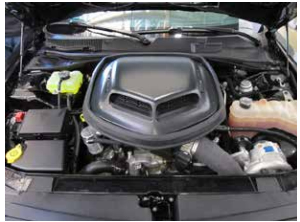
Fig. 13-e: Reinstall engine cover, shaker base, and shaker scoop
