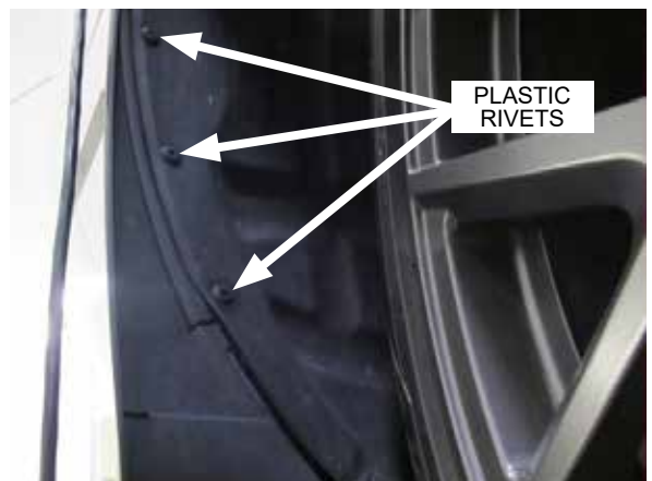
Fig. 13-c: Resecure using provided plastic rivets
