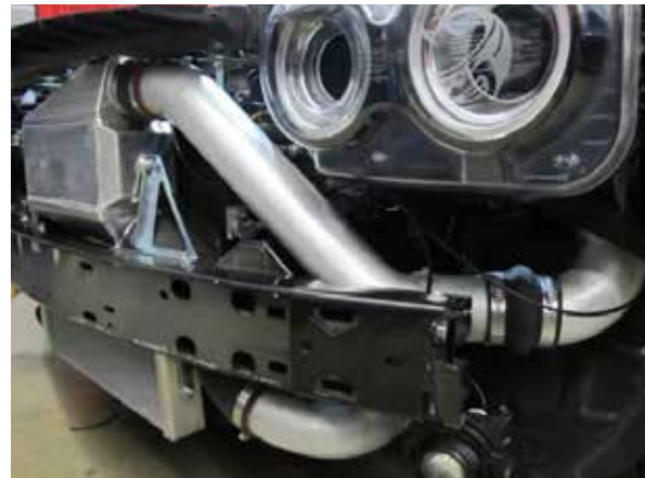
Fig. 8-i: Secure discharge tubes and discharge sleeves
