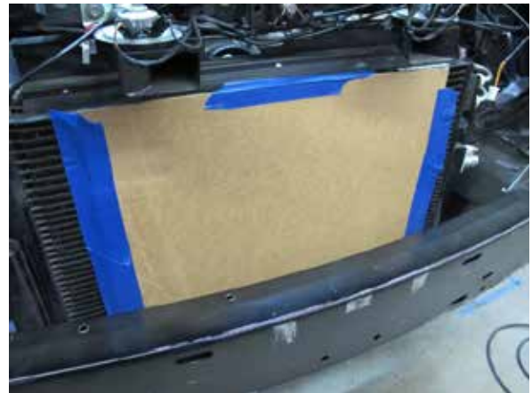
Fig. 7-e: Cover A/C condenser with cardboard
