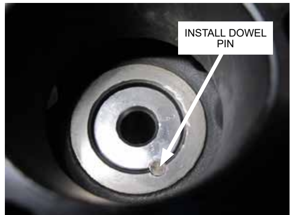
Fig. 3-e: Install dowel pin
