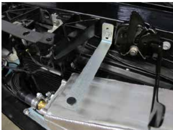
Fig. 10-a: 1.00" width radiator shroud bracket with rubber mount
