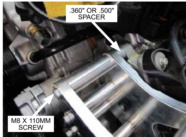
Fig. 6-g: Loosely attach S/C mounting bracket assembly to driver side cylinder head
