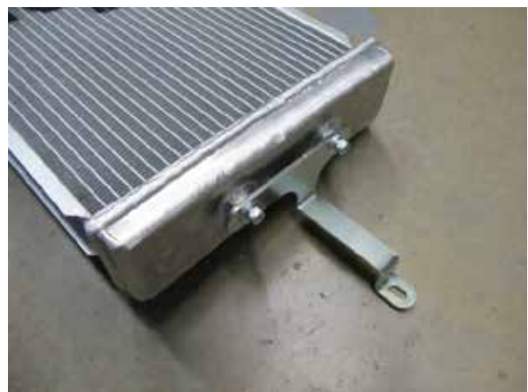
Fig. 7-i: Install driver side heat exchanger bracket
