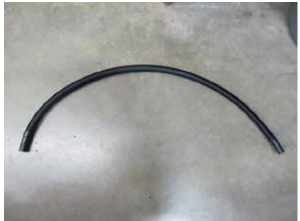
Fig. 9-n: 44" length of the 3/4" coolant hose
