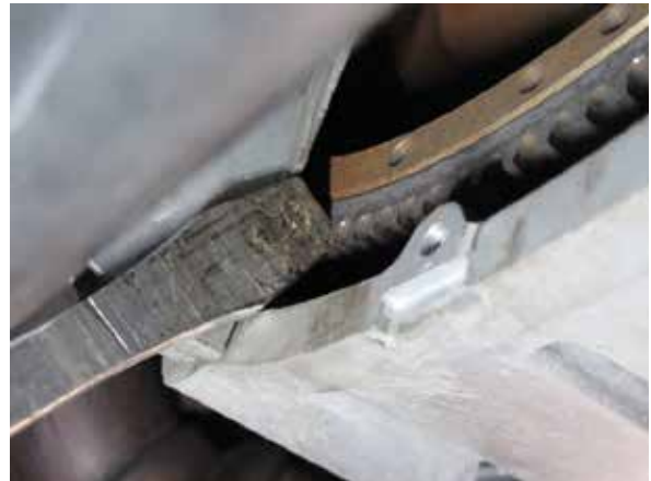
Fig. 3-g: Lock engine in position
