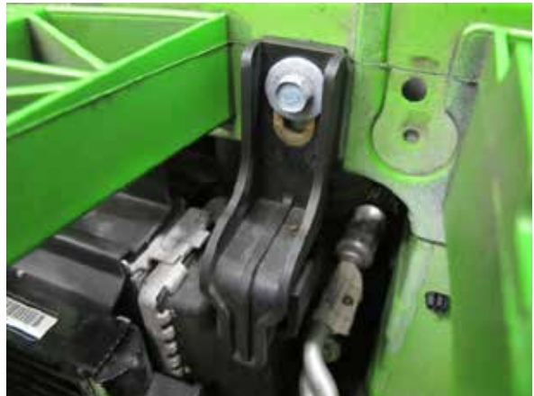
Fig. 7-a: Remove upper radiator bracket
