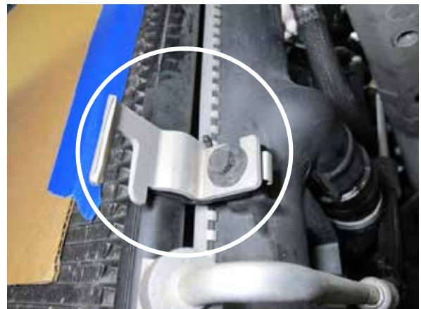
Fig. 7-f: Remove aluminum bracket and screw
