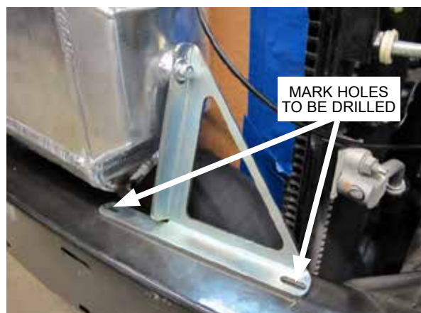
Fig. 7-u: Use driver side air/water cooler support bracket as drill template
