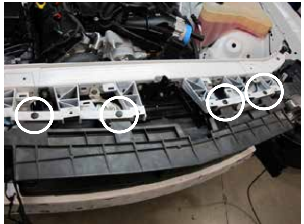
Fig. 2-m: Remove radiator shroud and fasteners
