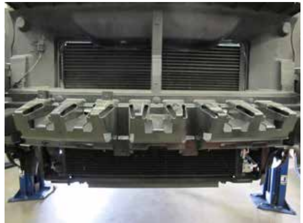
Fig. 2-k: Remove plastic bumper guard
