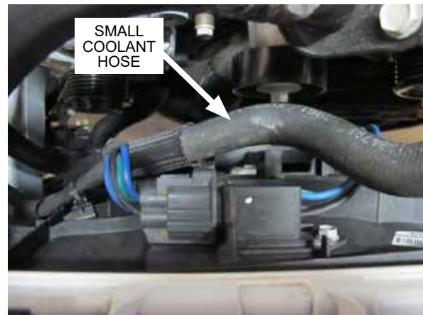
Fig. 2-t: Detach coolant hose and unplug radiator fan connector
