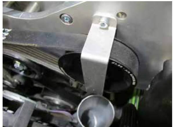
Fig. 6-k: Reinstall pulley guard
