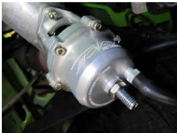
Fig. 8-k: Attach vacuum hose to bypass valve
