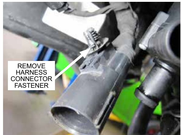
Fig. 9-e: Remove plastic harness connector fastener
