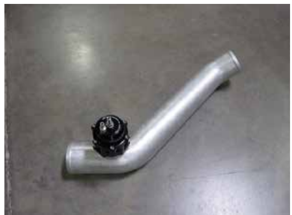
Fig. 7-ad: Install bypass valve to discharge tube 'B'
