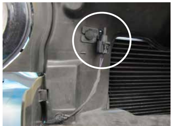
Fig. 2-l: Remove ambient air temperature sensor
