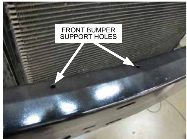
Fig. 7-p: 2x holes on front bumper support
