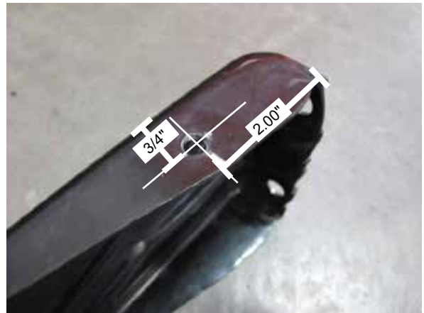
Fig. 4-h: Drill hole on passenger side rear edge of lower radiator support
