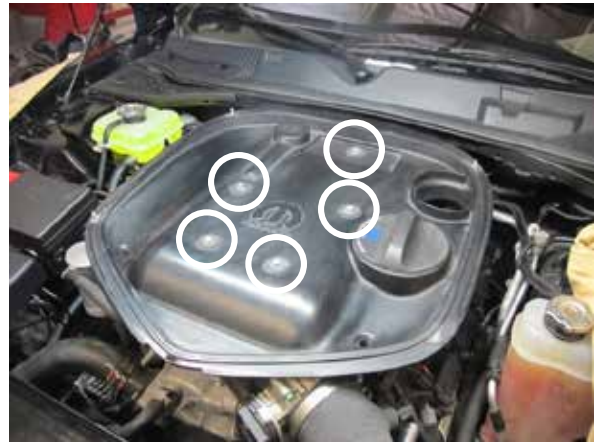
Fig. 2-p: Remove shaker base
