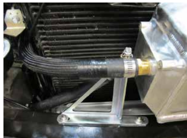
Fig. 9-u: Attach 3/4" coolant hose to air/water cooler
