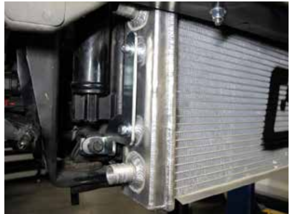
Fig. 7-j: Install passenger side of heat exchanger assembly
