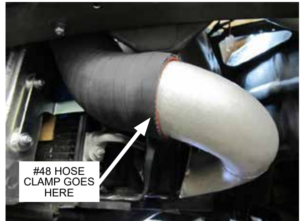
Fig. 7-z: Loosely install discharge tube 'D'
