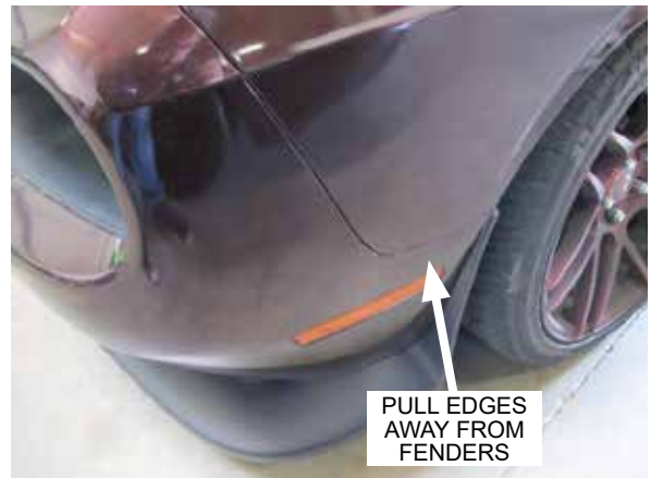
Fig. 2-j: Remove front bumper cover
