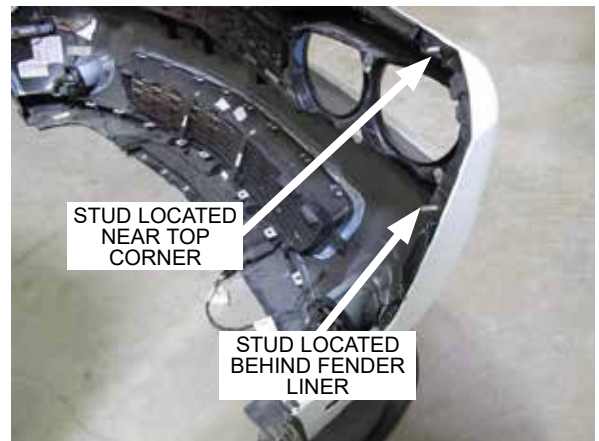
Fig. 2-h: Remove two nuts (Bumper removed for clarity)
