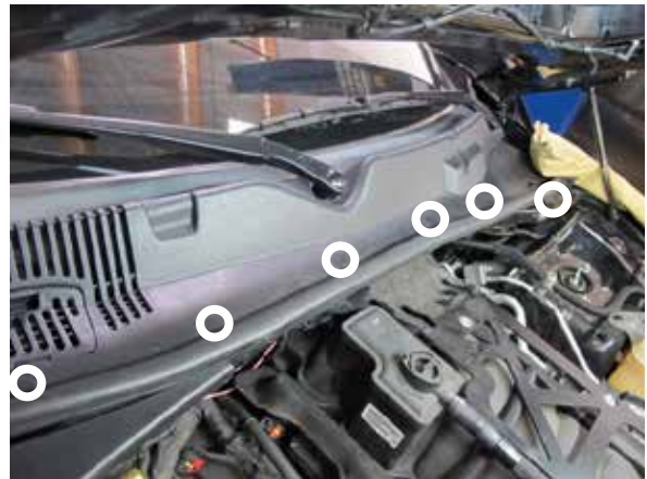
Fig. 1-b: Remove plastic fasteners
