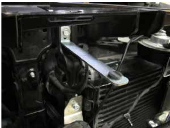
Fig. 10-b: 3/4" width radiator shroud bracket with rubber mount
