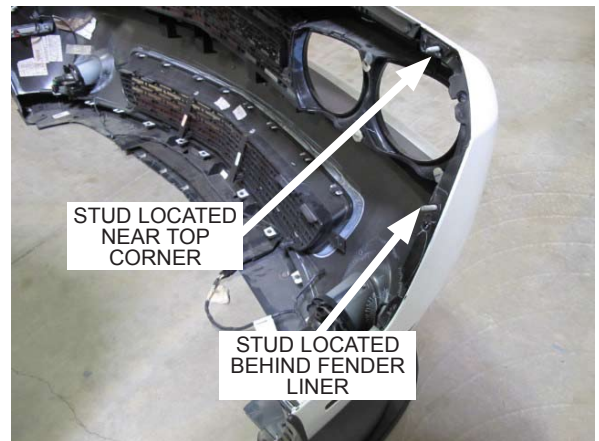
Fig. 2-h: Remove two nuts (Bumper removed for clarity)
