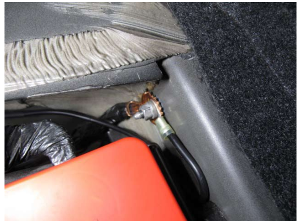
Fig. 12-h: Attach ground strap to grounding stud
