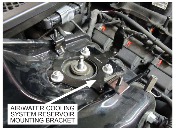
Fig. 9-l: Install air/water cooler system reservoir mount
