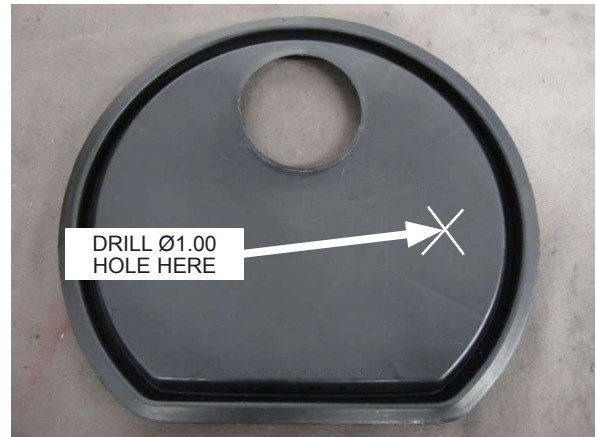
Fig. 12-m: Modify fuel pump access panel
