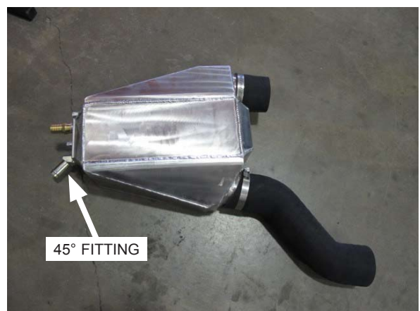
Fig. 7-x: Install silicone sleeves to air/water cooler as shown
