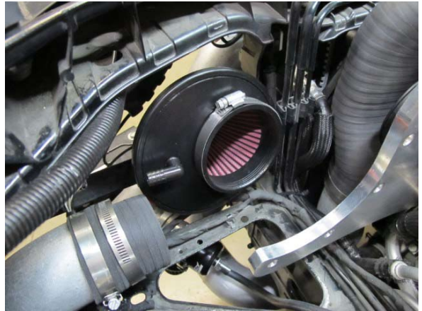
Fig. 8-a: Place air filter into position and install silicone sleeve to discharge tube 'A'
