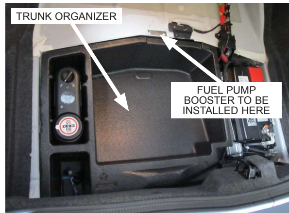
Fig. 12-a: Remove trunk carpet and trunk organizer
