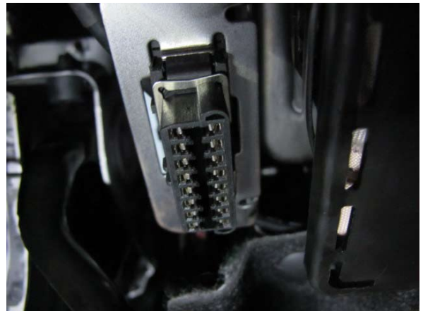
Fig. 14-e: Programming cable OBD II port installed
