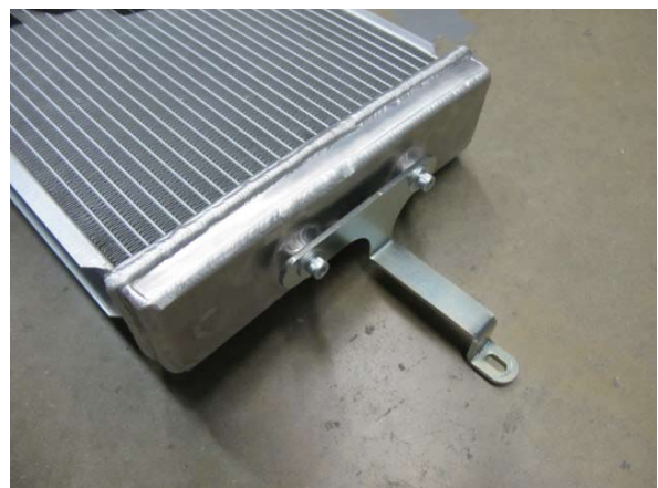
Fig. 7-i: Install driver side heat exchanger bracket
