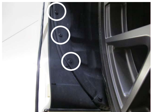
Fig. 2-c: Drill through and remove plastic rivets
