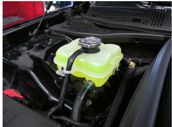
Fig. 9-z: Fill air/water cooling system with 50/50 water/coolant mix
