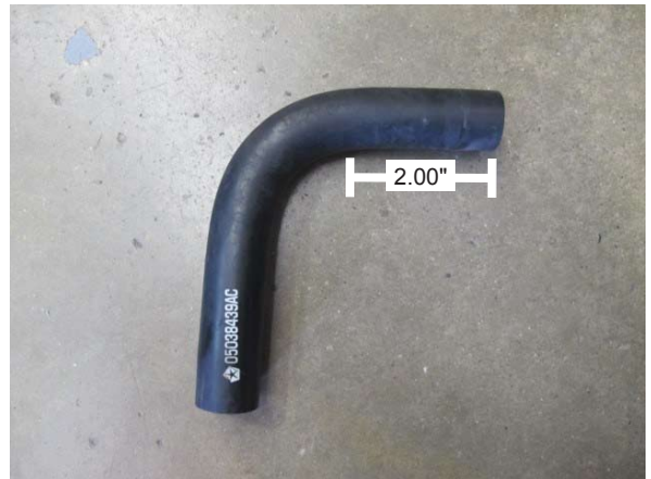
Fig. 8-e: Modify OEM breather hose
