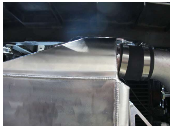
Fig. 10-e: Modified radiator shroud to air/water cooler clearance
