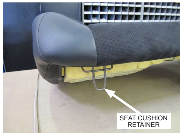
Fig. 12-i: Lower rear seat cushion retainers
