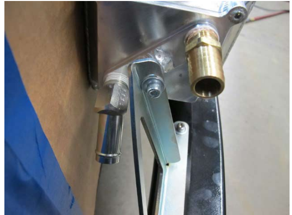
Fig. 7-s: Temporarily secure passenger side of air/water cooler
