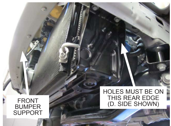
Fig. 4-i: Reinstall lower radiator support
