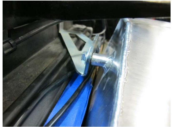
Fig. 7-t: Temporarily secure top side of air/water cooler
