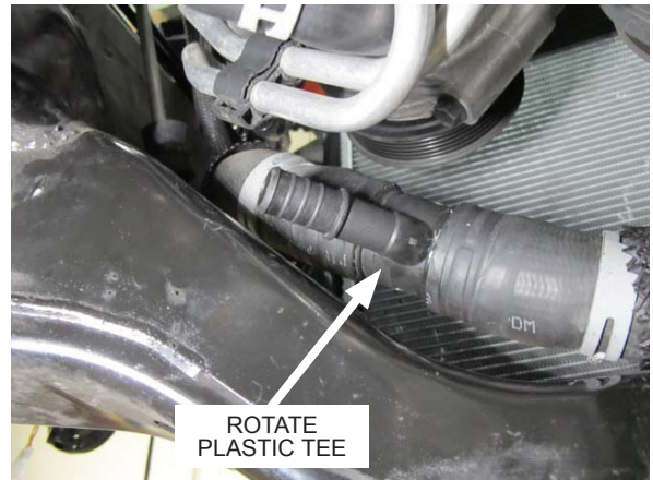
Fig. 5-d: Rotate plastic tee 180° clockwise
