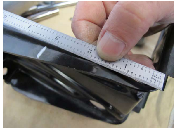
Fig. 4-d: Measure 3.25" from bottom edge
