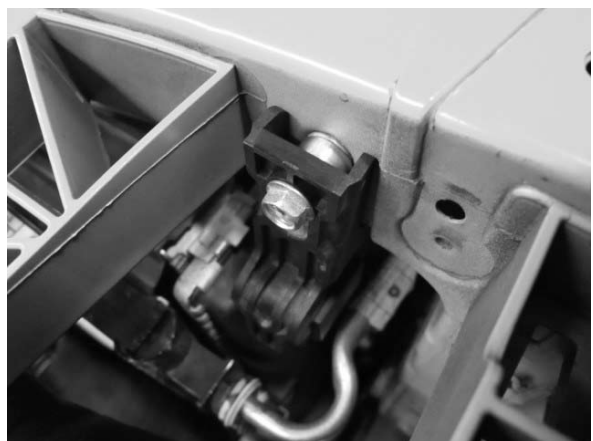
Fig. 7-c: Install upper radiator bracket as shown
