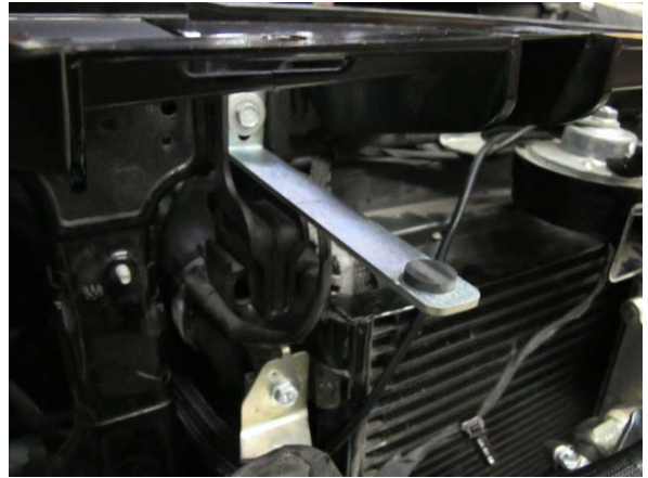
Fig. 10-b: 3/4" width radiator shroud bracket with rubber mount
