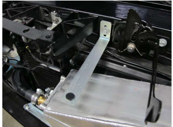
Fig. 10-a: 1.00" width radiator shroud bracket with rubber mount
