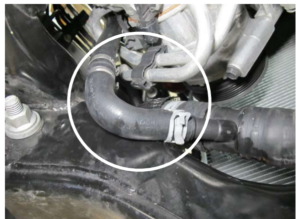
Fig. 5-f: Install 90° end of new coolant reservoir hose to plastic tee
