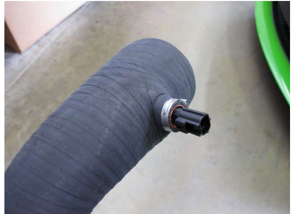
Fig. 7-ab: Install IAT sensor to molded boss on discharge sleeve 'E'
