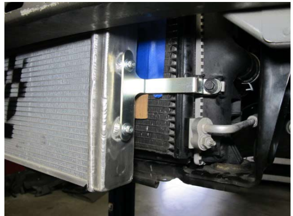
Fig. 7-k: Install driver side of heat exchanger assembly
