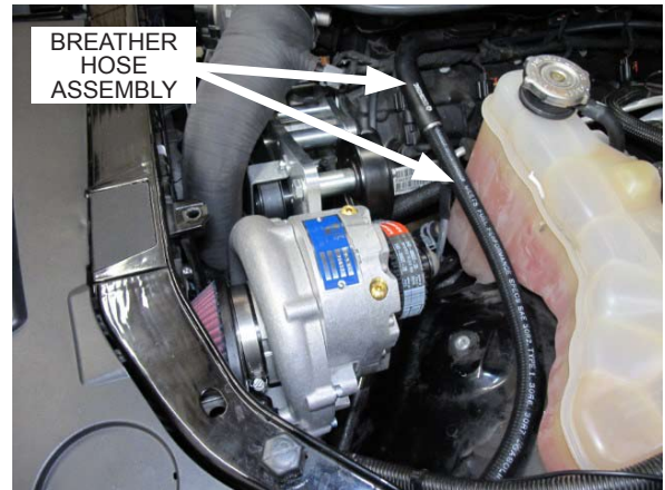
Fig. 8-g: Install breather hose assembly
