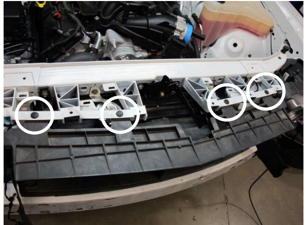
Fig. 2-m: Remove radiator shroud and fasteners
