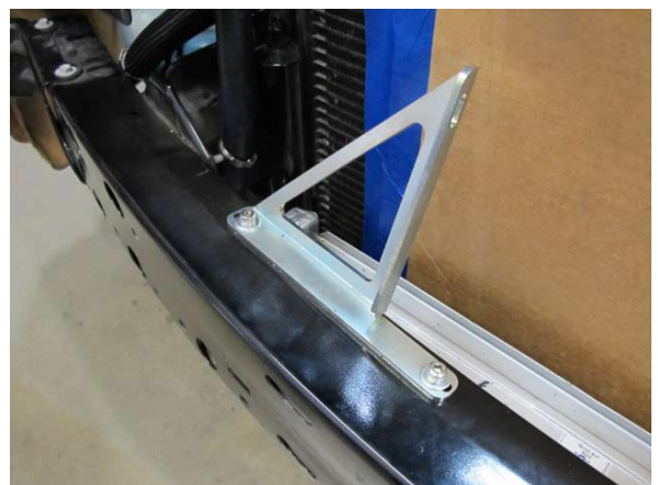
Fig. 7-r: Loosely install passenger side air/water cooler support bracket
