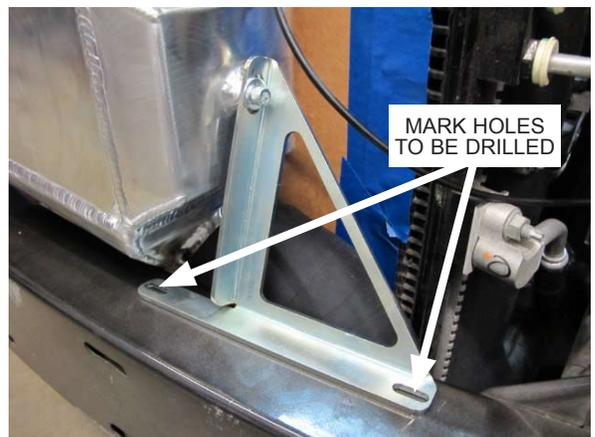
Fig. 7-r: Use driver side air/water cooler support bracket as drill template
