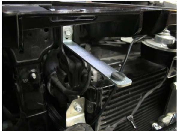
Fig. 10-b: 3/4" width radiator shroud bracket with rubber mount
