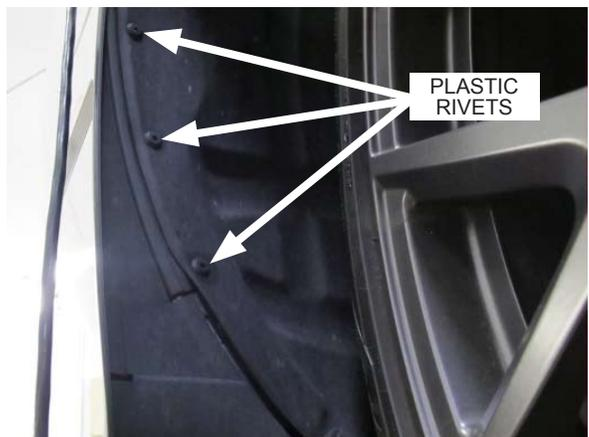
Fig. 11-c: Resecure using provided plastic rivets
