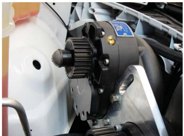
Fig. 8-c: Install supercharger to supercharger mounting bracket assembly
