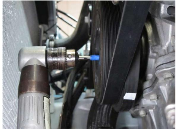
Fig. 3-d: Drill crankshaft / damper assembly
