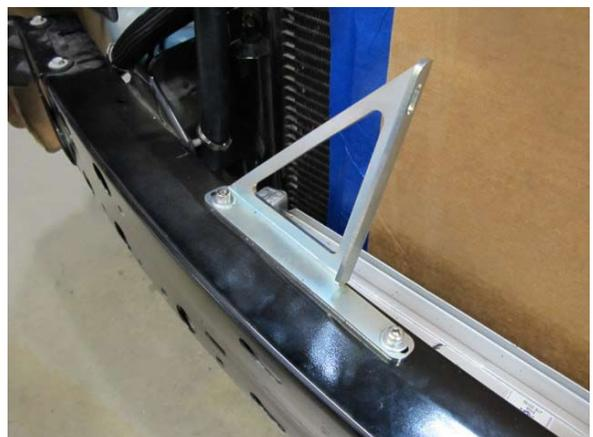
Fig. 7-o: Loosely install passenger side air/water cooler support bracket
