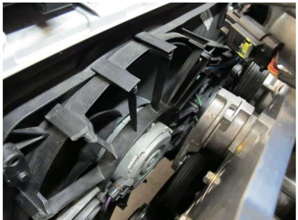
Fig. 4-c: Reinstall radiator fan assembly
