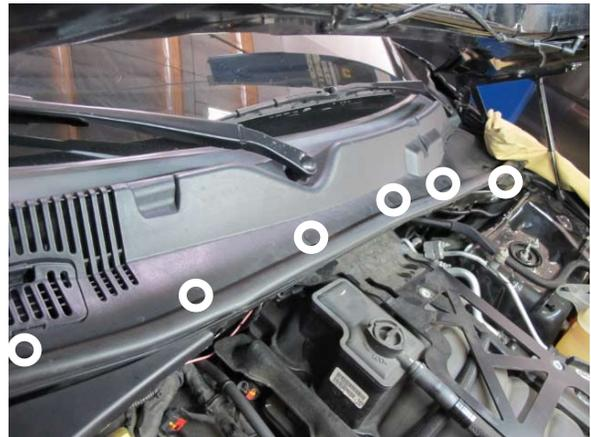
Fig. 1-b: Remove plastic fasteners
