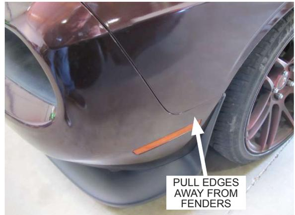
Fig. 2-j: Remove front bumper cover
