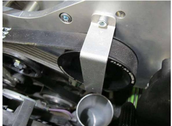
Fig. 6-j: Reinstall pulley guard
