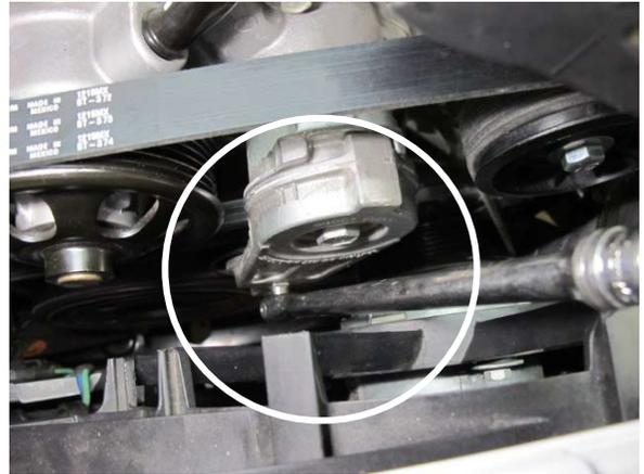
Fig. 2-y: Remove accessory drive belt
