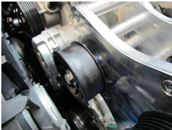
Fig. 6-h: Reinstall serpentine belt idler pulley
