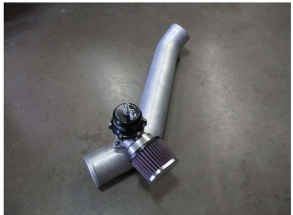
Fig. 7-aa: Install bypass valve to discharge tube 'B'
