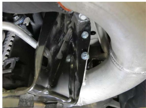
Fig. 7-x: Secure discharge tube 'D' to lower radiator support
