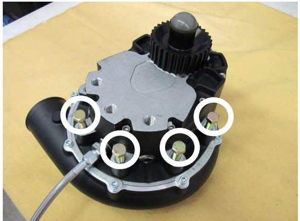
Fig. 8-b: Lubricate supercharger mounting boss threads
