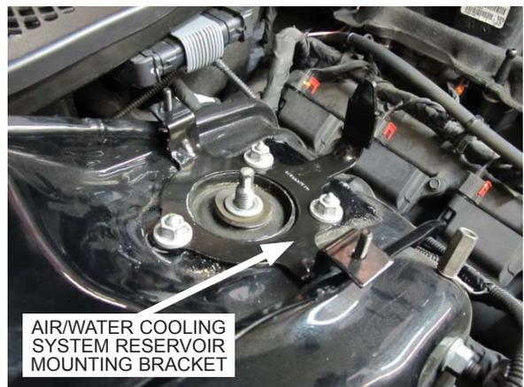
Fig. 9-l: Install air/water cooler system reservoir mount
