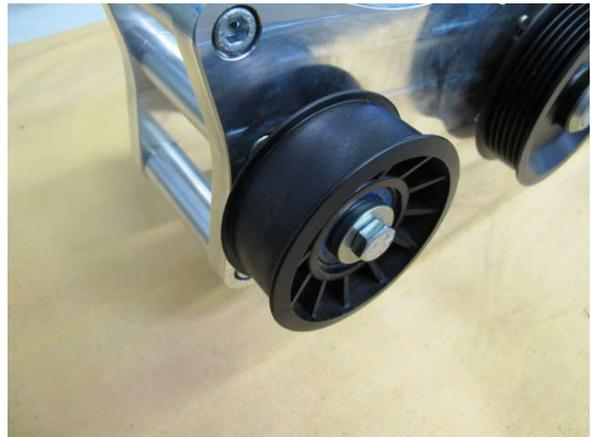
Fig. 6-b: Remove serpentine belt idler pulley
