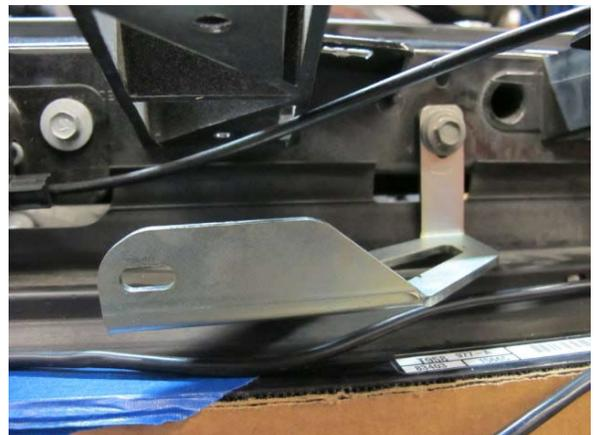
Fig. 7-l: Install upper air/water cooler support bracket
