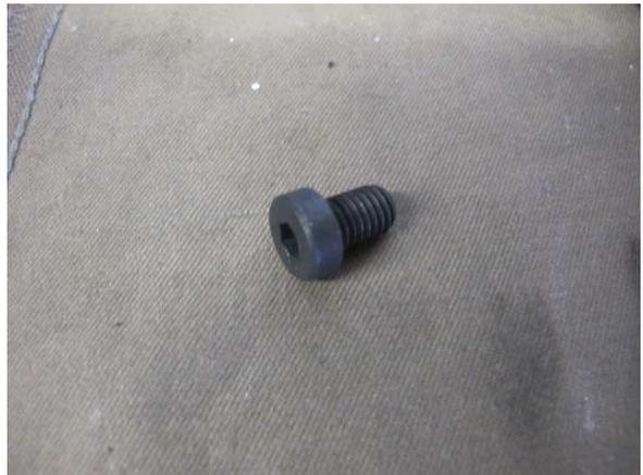
Fig. 9-h: Shorter front bumper support screw
