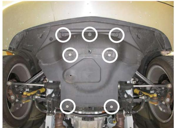
Fig. 2-e: Remove splash guard
