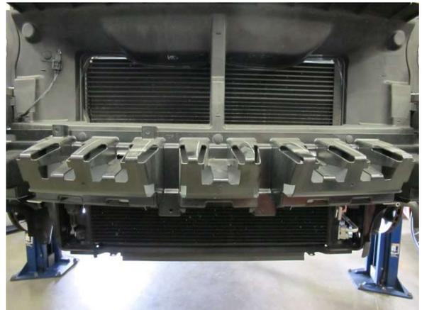
Fig. 2-k: Remove plastic bumper guard
