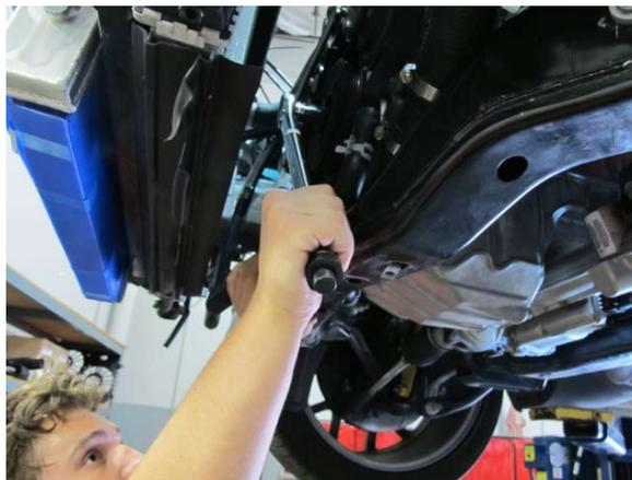
Fig. 3-h: Torque crank bolt
