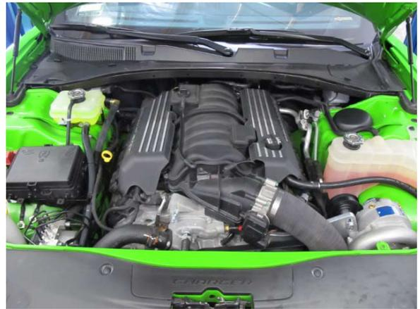
Fig. 11-e: Reinstall both engine covers
