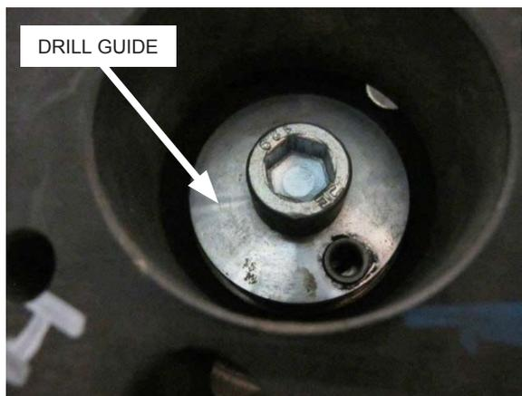
Fig. 3-b: Install drill guide
