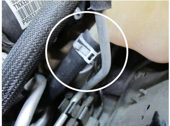
Fig. 5-g: Attach coolant hose to coolant reservoir
