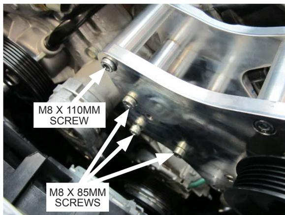
Fig. 6-g: Secure S/C mounting bracket hardware
