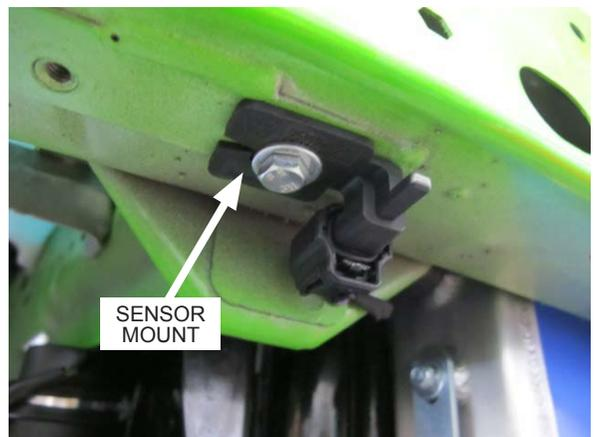
Fig. 7-ad: Reinstall ambient air temperature sensor as shown
