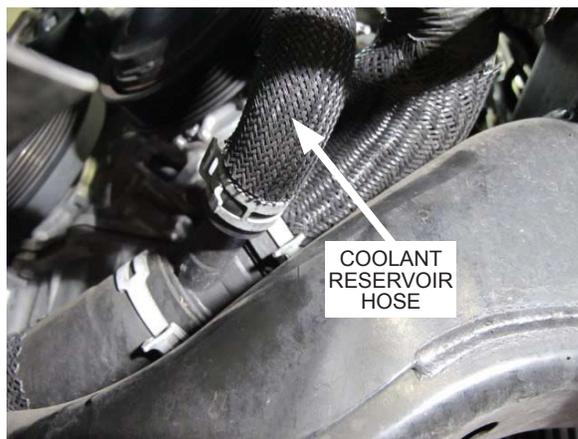
Fig. 5-b: Detach coolant reservoir hose from plastic tee
