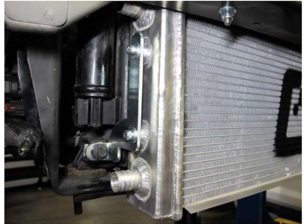
Fig. 7-g: Install passenger side of heat exchanger assembly
