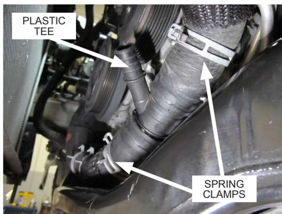
Fig. 5-c: Temporarily move two spring clamps
