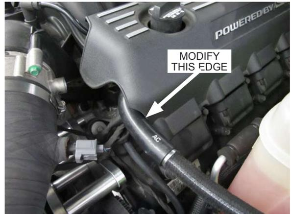
Fig. 11-d: Modify driver side engine cover
