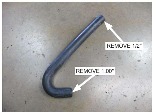
Fig. 9-i: Modify 150° molded hose as shown
