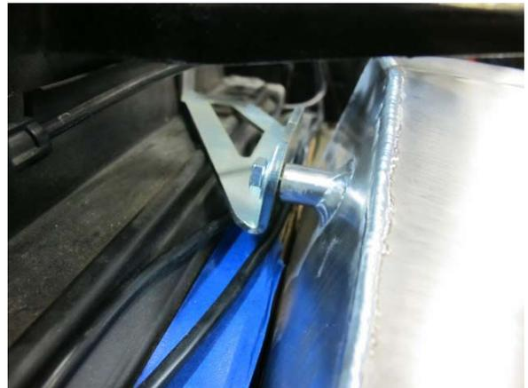
Fig. 7-q: Temporarily secure top side of air/water cooler
