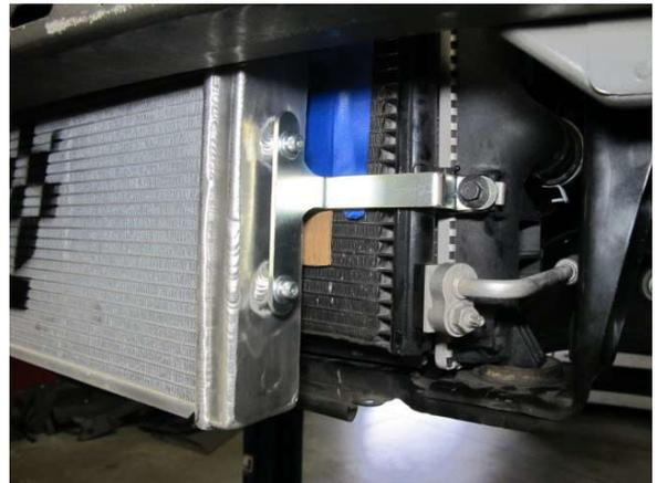
Fig. 7-h: Install driver side of heat exchanger assembly
