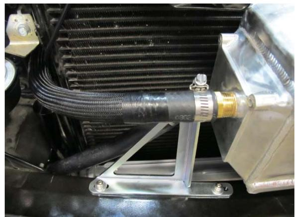
Fig. 9-u: Attach 3/4" coolant hose to air/water cooler
