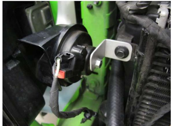
Fig. 7-k: Relocate driver side horn to upper radiator
