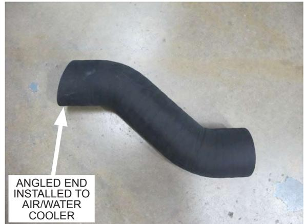
Fig. 7-t: Discharge sleeve 'C'
