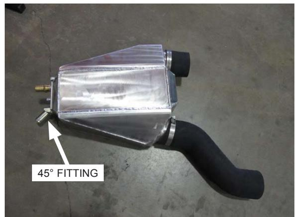
Fig. 7-u: Install silicone sleeves to air/water cooler as shown
