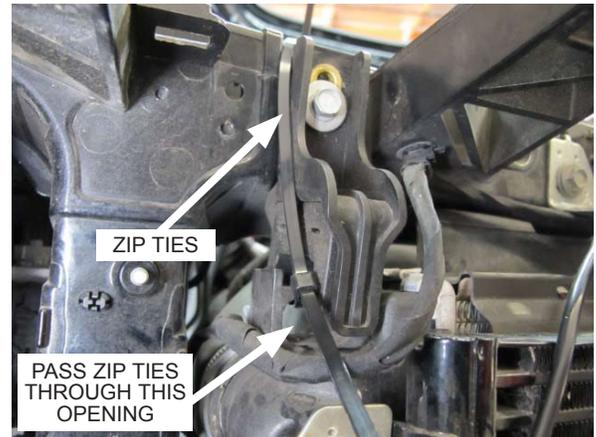
Fig. 2-v: Zip tie radiator to core support
