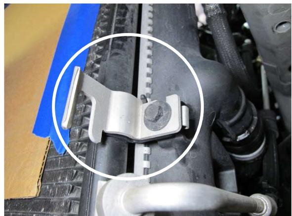
Fig. 7-c: Remove aluminum bracket and screw
