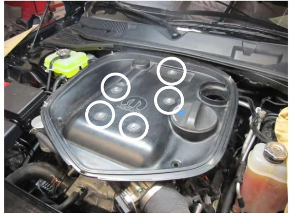
Fig. 2-p: Remove shaker base
