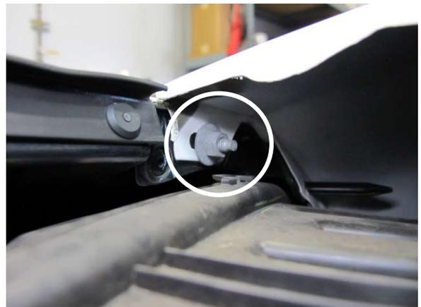
Fig. 2-f: Remove two nuts
