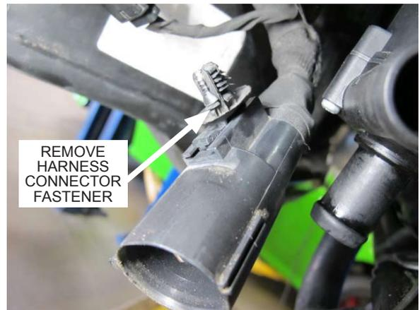
Fig. 9-e: Remove plastic harness connector fastener
