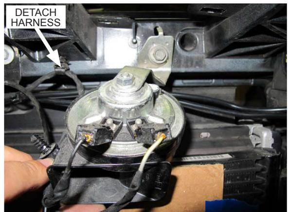
Fig. 7-i: Remove driver side horn
