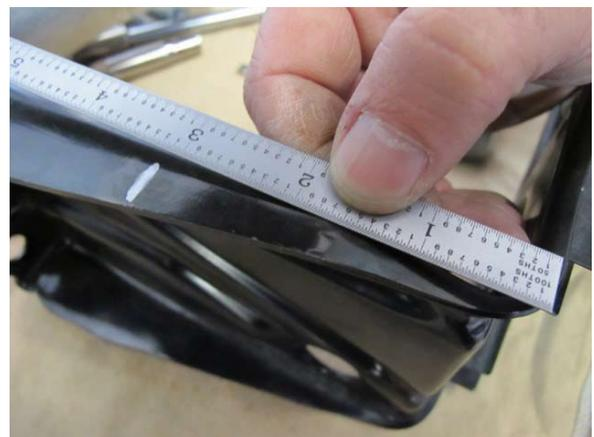
Fig. 4-f: Measure 3.25" from bottom edge
