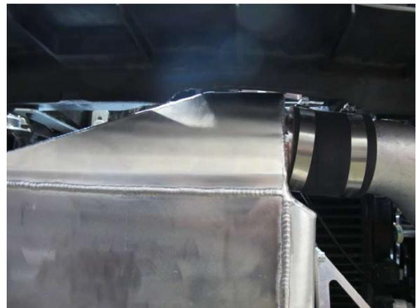
Fig. 10-e: Modified radiator shroud to air/water cooler clearance
