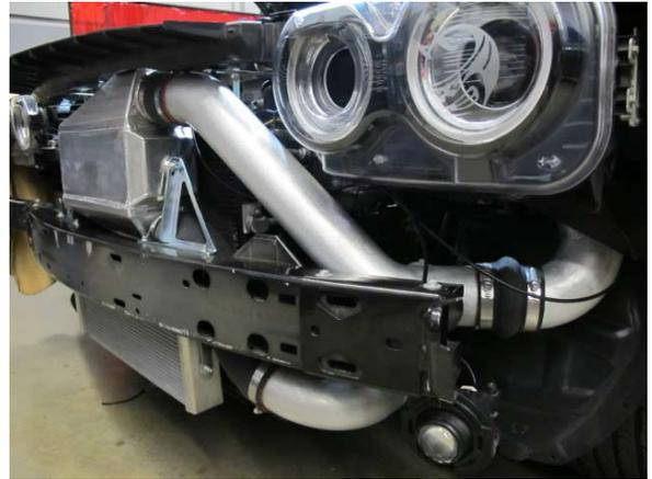
Fig. 7-ab: Install discharge tube 'B'
