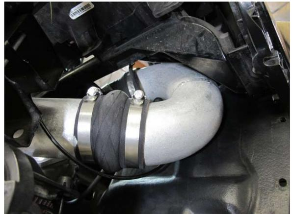
Fig. 7-ac: Loosely install discharge tube 'A' to discharge tube 'B'
