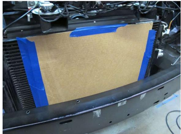
Fig. 7-b: Cover A/C condenser with cardboard
