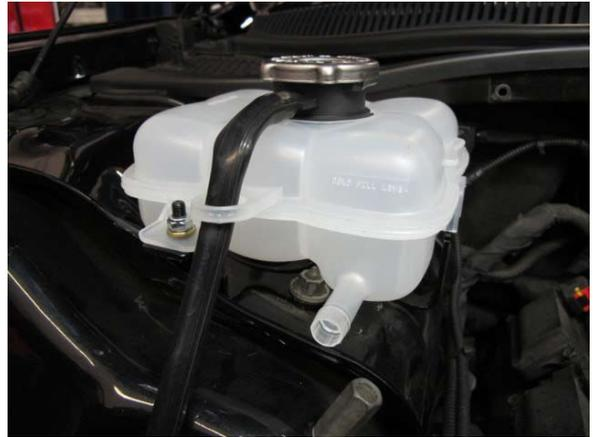
Fig. 9-m: Install air/water cooler system reservoir to mount
