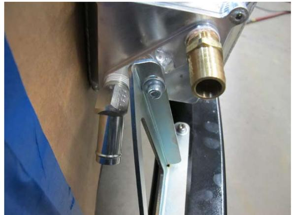
Fig. 7-p: Temporarily secure passenger side of air/water cooler
