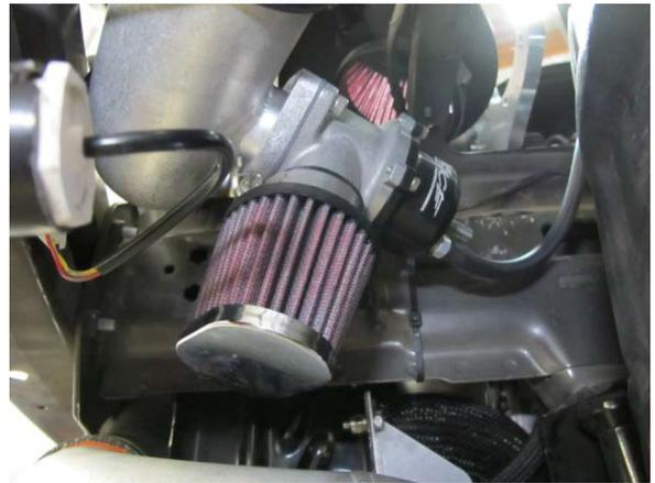
Fig. 8-k: Attach vacuum hose to bypass valve
