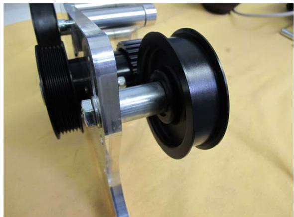
Fig. 6-c: Remove cog belt idler pulley
