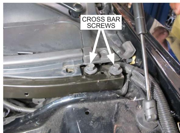
Fig. 1-c: Remove cross bar screws
