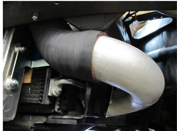
Fig. 7-w: Loosely install discharge tube 'D'
