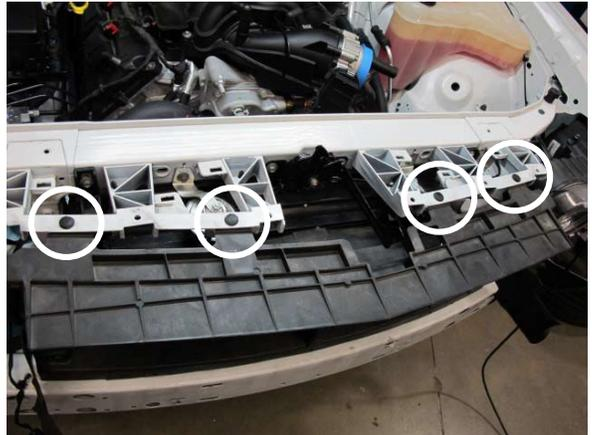
Fig. 2-m: Remove radiator shroud and fasteners
