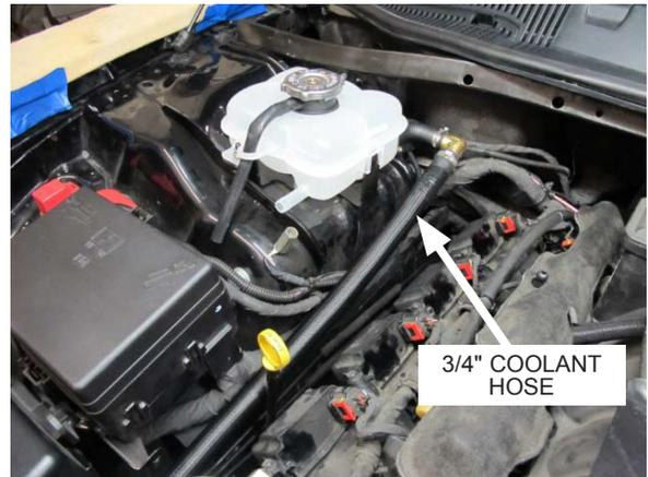
Fig. 9-s: Route 3/4" coolant hose towards air/water cooler
