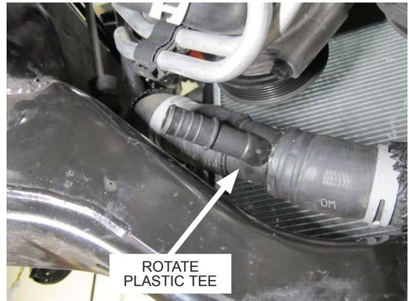
Fig. 5-d: Rotate plastic tee 180° clockwise
