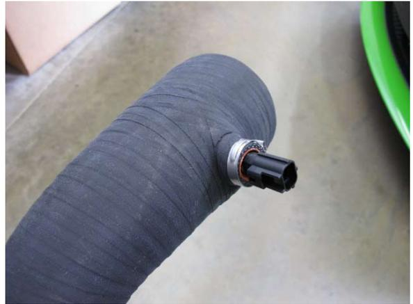
Fig. 7-y: Install IAT sensor to molded boss on discharge sleeve 'E'
