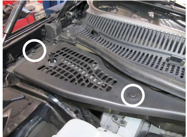
Fig. 1-d: Remove two plastic fasteners
