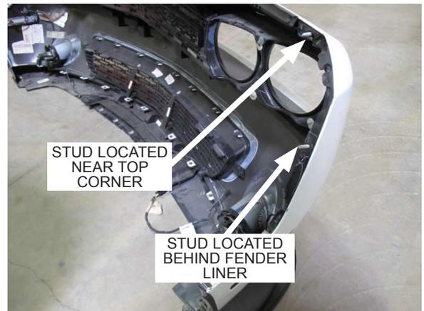
Fig. 2-h: Remove two nuts
