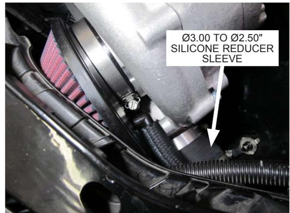
Fig. 8-h: Secure air filter and discharge tube A to supercharger
