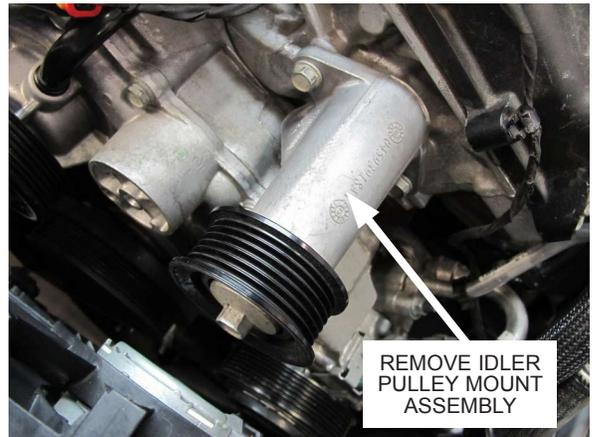
Fig. 2-z: Remove idler pulley mount assembly
