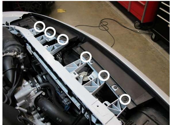
Fig. 2-b: Remove six plastic fasteners
