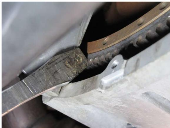
Fig. 3-g: Lock engine in position
