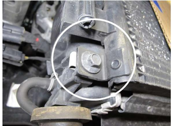
Fig. 7-d: Remove screw
