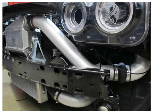
Fig. 8-i: Secure discharge tubes and discharge sleeves
