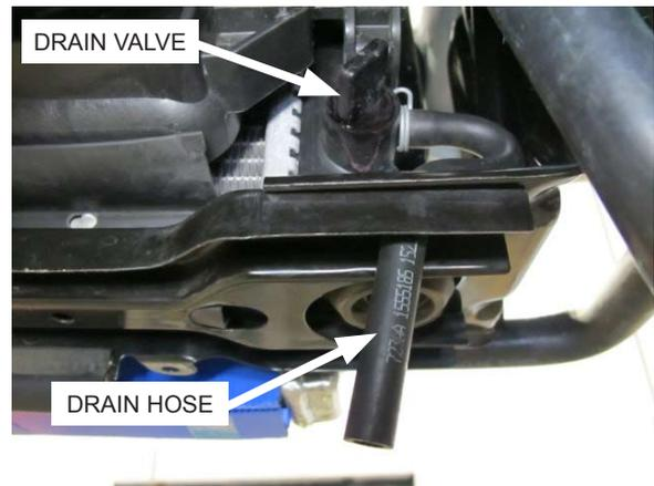
Fig. 2-s: Drain coolant
