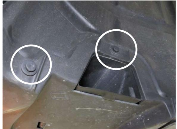
Fig. 2-d: Remove two plastic fasteners
