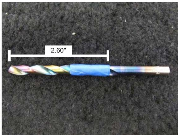
Fig. 3-c: Measure drill bit to 2.60"
