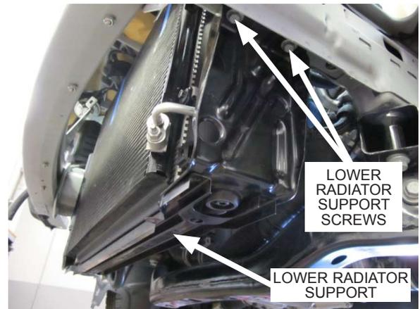
Fig. 2-w: Remove lower radiator support hardware
