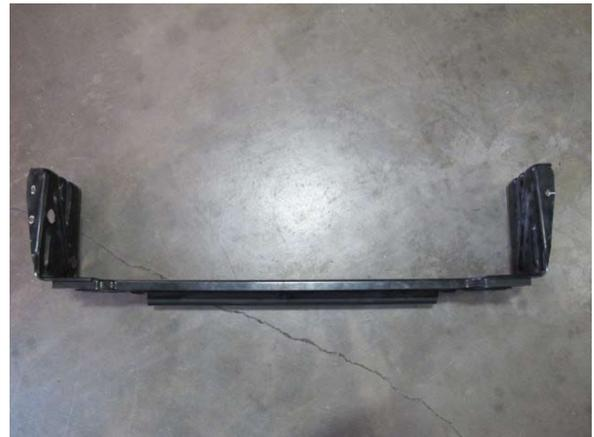
Fig. 4-e: Lower radiator support
