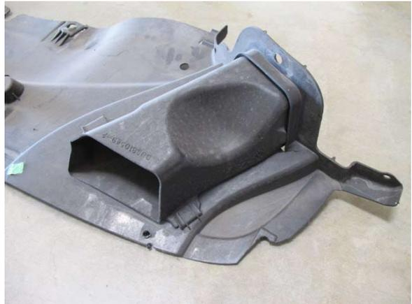
Fig. 11-a: Front brake cooling ducts
