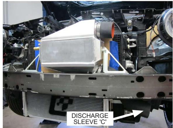
Fig. 7-v: Install air/water cooler
