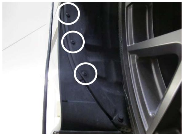
Fig. 2-c: Drill through and remove plastic rivets
