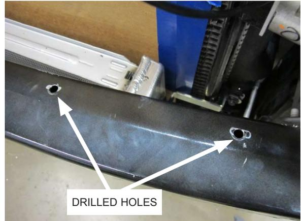
Fig. 7-s: Drill 2x holes using 6" length drill bit
