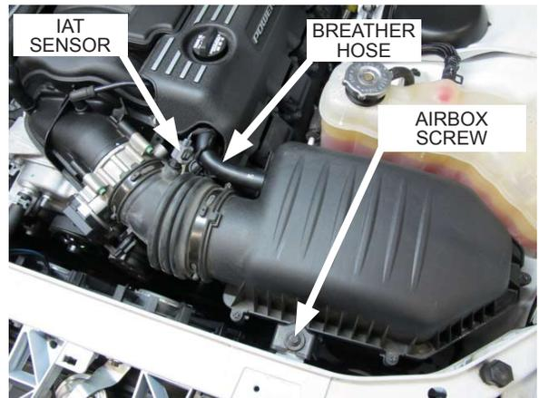
Fig. 2-q: Remove airbox and air inlet duct
