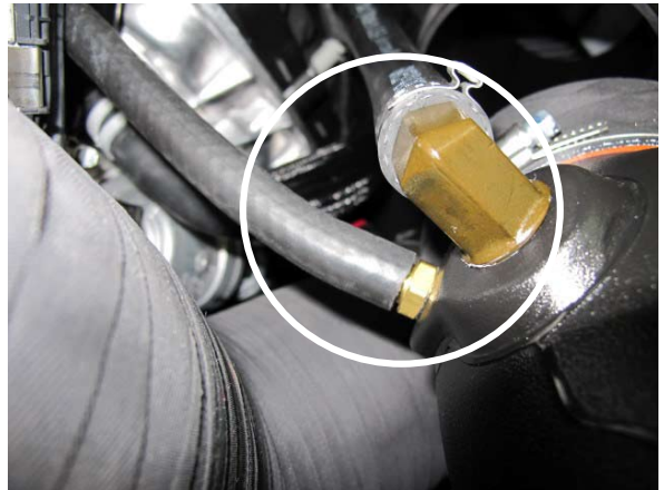
Fig. 7-m: Install 3/8" Hose, Then Secure Air Inlet Tube
