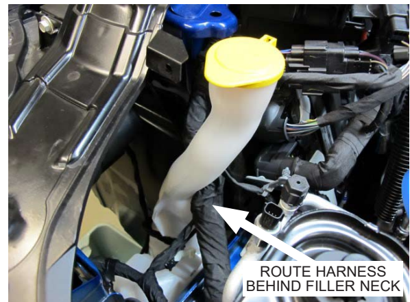
Fig. 4-k: Reinstall Windshield Washer Fluid Reservoir
