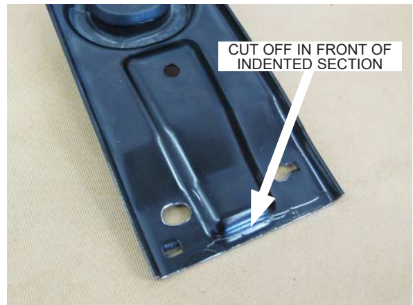
Fig. 3-e: Cut The Upper Radiator Bracket As Shown
