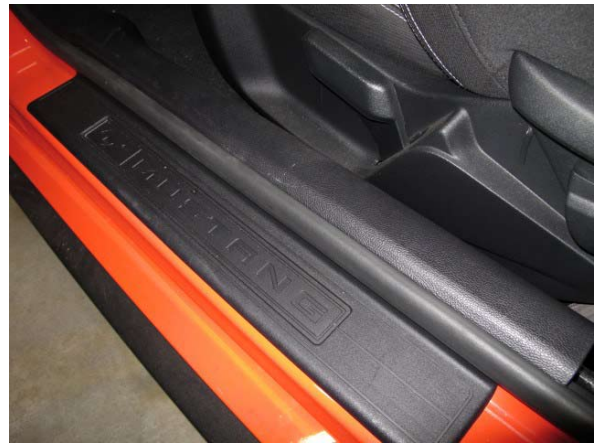
Fig. 6-q: Reinstall Interior Panel Above Driver Side Door Sill
