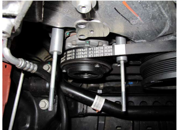
Fig. 2-g: Install 1x 2.058" & 1x 2.146" Spacers
