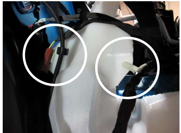
Fig. 4-e: Detach Electrical Harnesses & Windshield Washer Fluid Line
