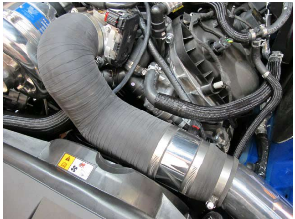
Fig. 4-aq: Secure All Hose Clamps
