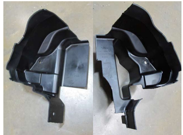
Fig. 4-w: Modify Radiator Shrouds
