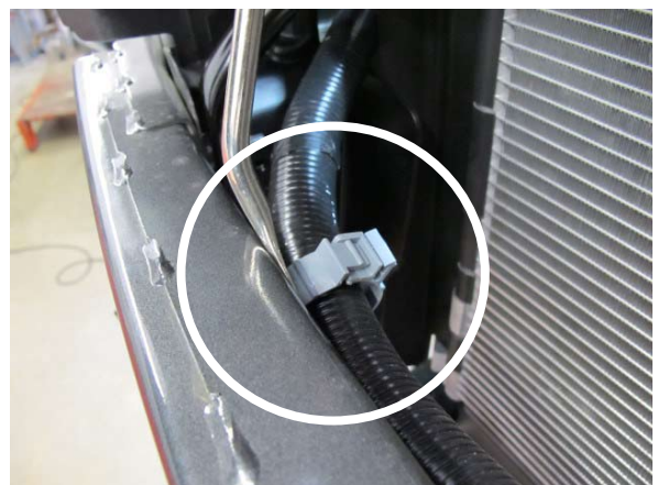
Fig. 4-o: Detach Wire Harness
