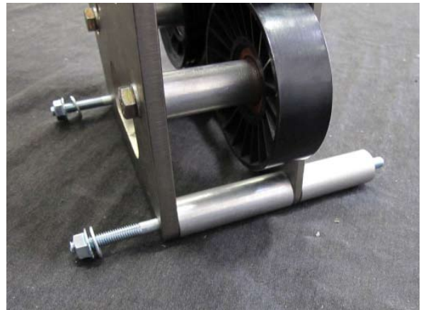
Fig. 2-h: Keep 2x 2.730" Spacers In Place
