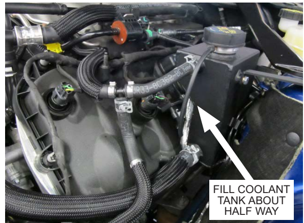
Fig. 3-y: Refill Cooling System
