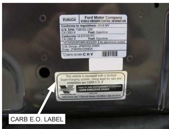
Fig. 8-b: Affix Emissions Label As Shown
