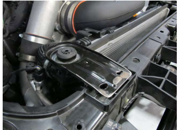
Fig. 3-g: Reinstall Modified Upper Radiator Brackets
