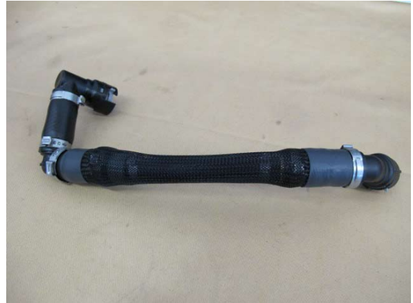
Fig. 7-d: Loosely Assemble OEM Quick-Release Fittings As Shown
