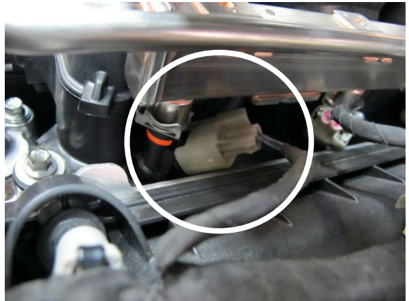
Fig. 5-d: Disconnect Fuel Injectors
