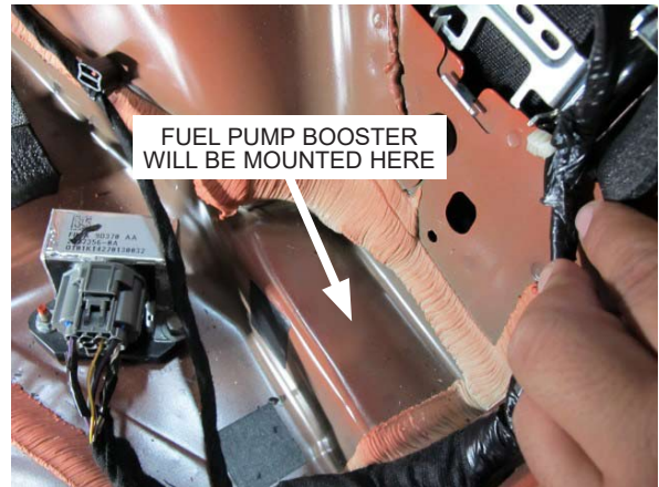
Fig. 6-j: Fuel Pump Booster Mounting Location
