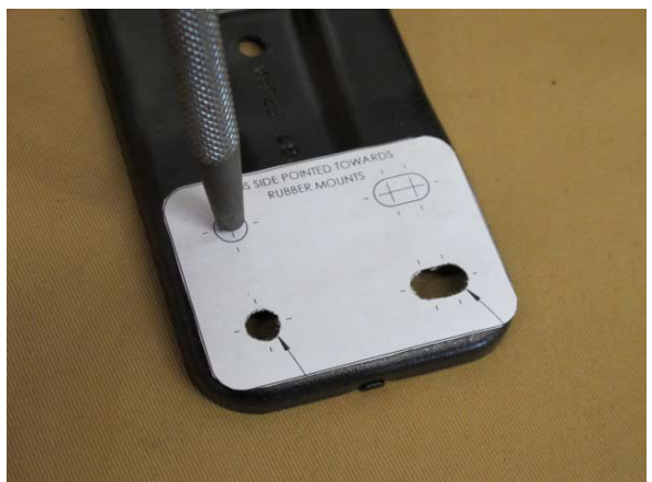
Fig. 3-c: Center Punch The Holes To Be Drilled
