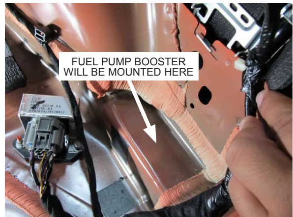
Fig. 6-j: Fuel Pump Booster Mounting Location
