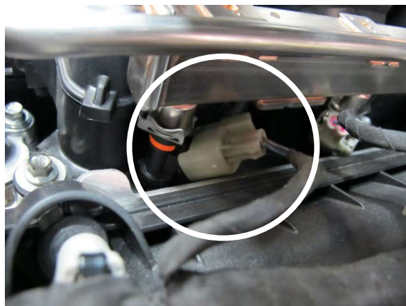
Fig. 5-d: Disconnect Fuel Injectors
