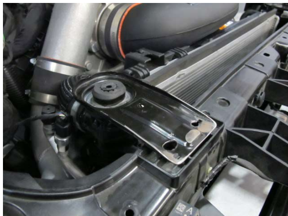
Fig. 3-g: Reinstall Modified Upper Radiator Brackets
