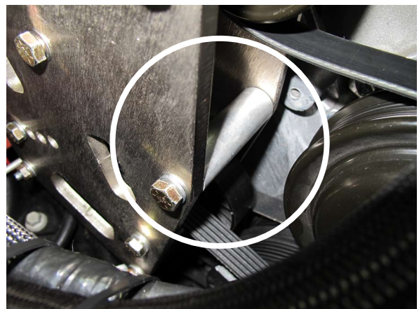
Fig. 2-r: Reinstall Previously Removed 1x 2.730" Spacer
