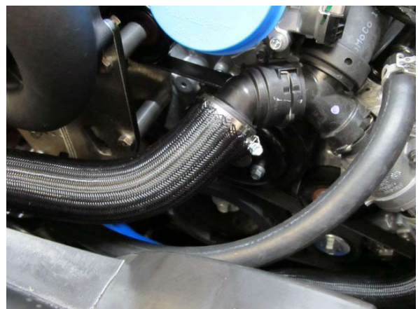
Fig. 3-l: Secure Quick-Release To Hose Using #24 Hose Clamp
