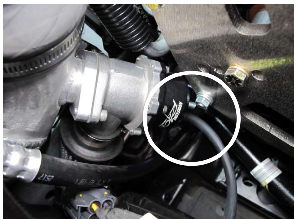
Fig. 4-as: Attach Vacuum Hose To Bypass Valve (M/T Bypass Valve Picture, Same For A/T)
