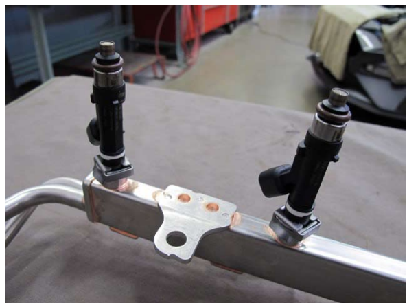
Fig. 5-i: Make Note Of Fuel Injector Orientation
