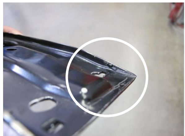
Fig. 3-f: Grind Down Raised Edges To A Taper
