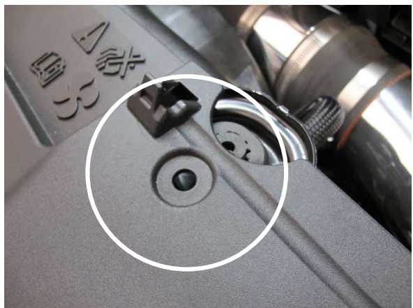
Fig. 7-o: Check Upper Radiator Support Cover
