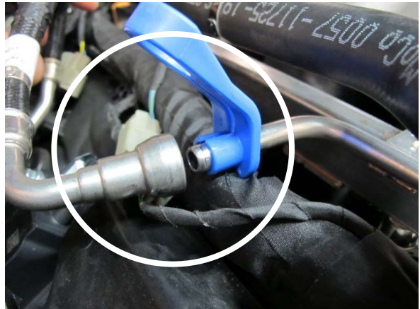
Fig. 5-g: Disconnect Direct Injection Fuel Line
