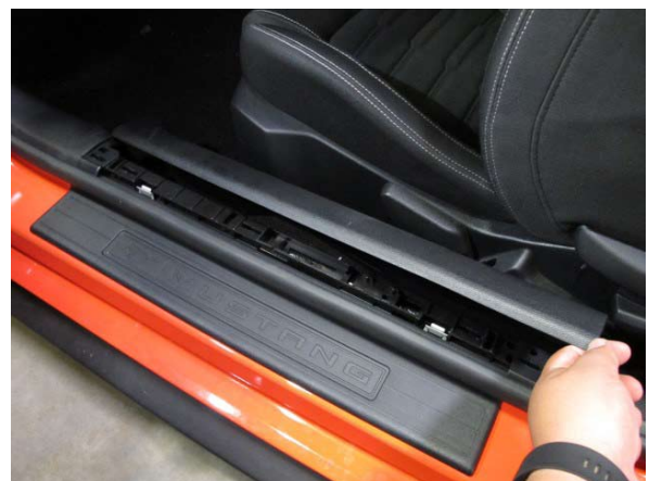
Fig. 6-f: Remove Interior Panel Above Driver Side Door Sill
