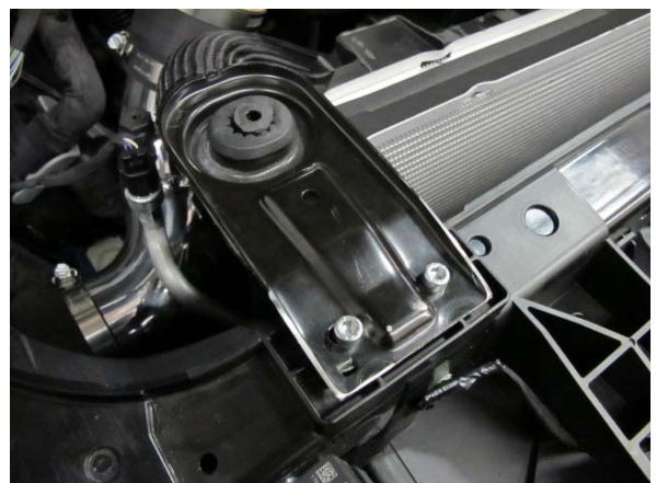
Fig. 4-av: Reinstall Modified Upper Radiator Brackets
