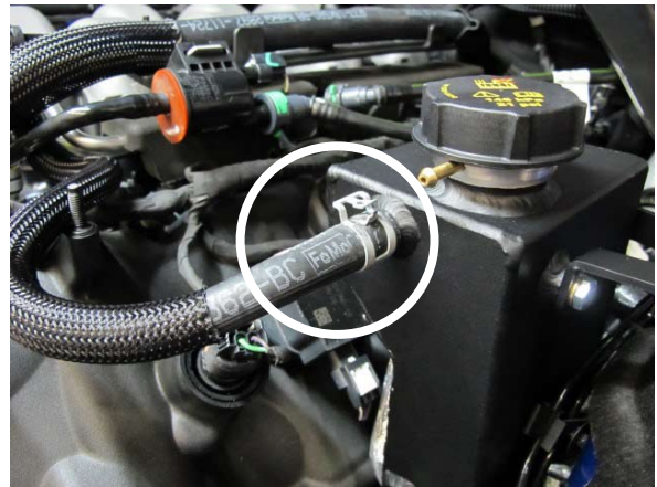
Fig. 3-t: Attach Upper OEM Molded Coolant Hose
