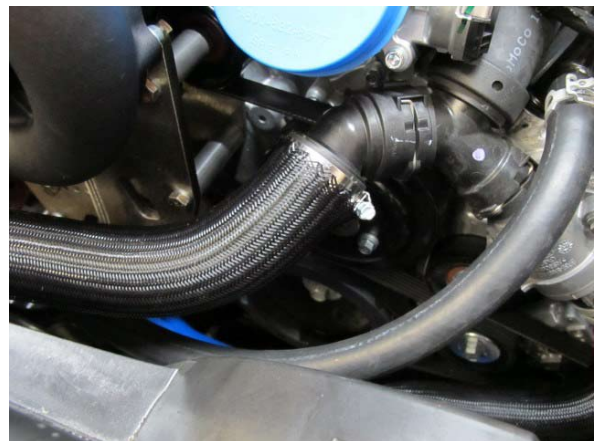
Fig. 3-l: Secure Quick-Release To Hose Using #24 Hose Clamp
