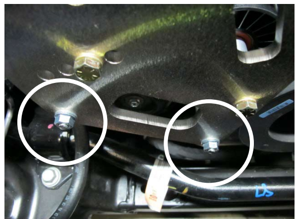
Fig. 2-l: Install 2x M8 Nuts & 2x 5/16" Washers
