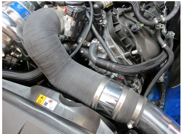
Fig. 4-aq: Secure All Hose Clamps
