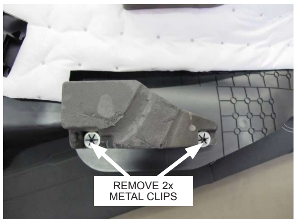
Fig. 6-i: Remove Foam Insulation Block
