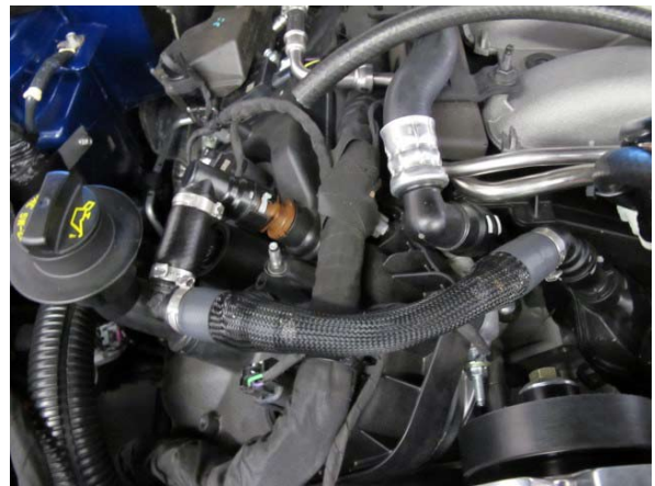
Fig. 7-e: Install PCV Assembly
