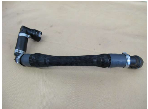
Fig. 7-d: Loosely Assemble OEM Quick-Release Fittings As Shown
