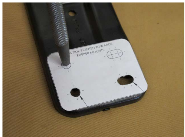
Fig. 3-c: Center Punch The Holes To Be Drilled
