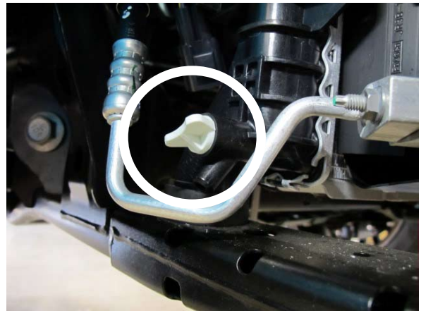
Fig. 1-w: Drain Engine Coolant
