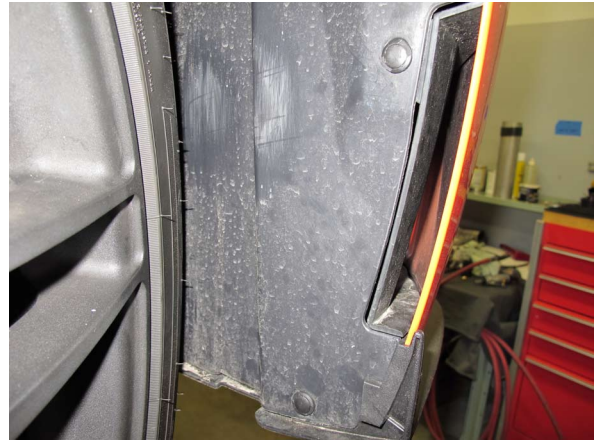
Fig. 1-d: Remove Fender Liner Fasteners0
