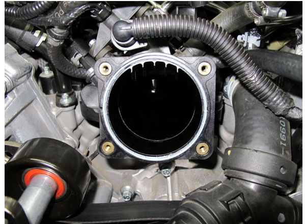
Fig. 3-v: Clean T-Body Flange & Verify O-Ring Placement
