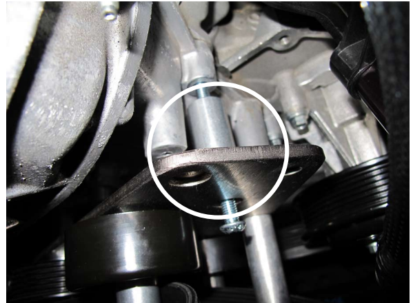
Fig. 3-j: Secure Top Of Rear Mounting Plate
