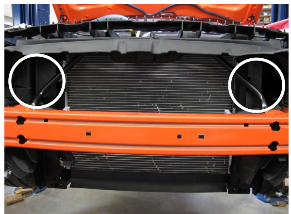
Fig. 1-l: Remove Radiator Shrouds
