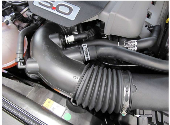
Fig. 1-m: Remove Intake Tube
