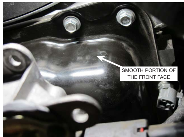
Fig. 12-b: Mark Oil Pan
