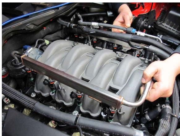
Fig. 6-c: Remove Fuel injector Rail Assembly
