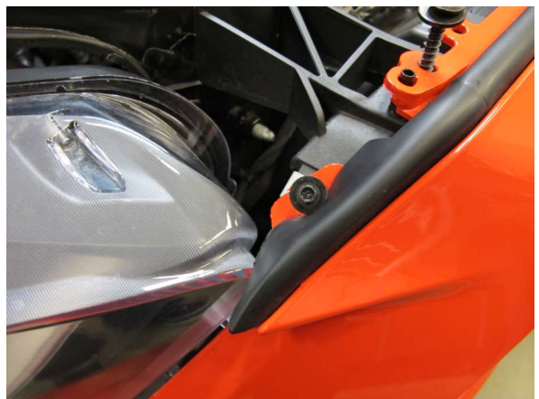
Fig. 1-c: Remove 5.5mm-Headed Fastener
