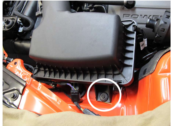
Fig. 5-d: Remove Air Box
