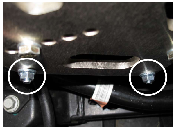
Fig. 3-l: Secure Lower Mounting Bracket Fasteners
