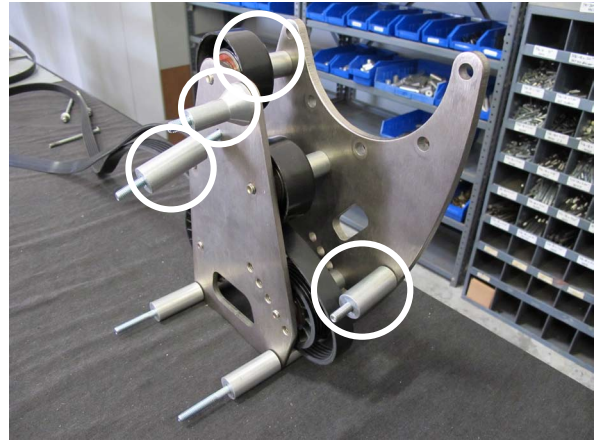
Fig. 3-d: Remove Spacers & Hardware (Circled)
