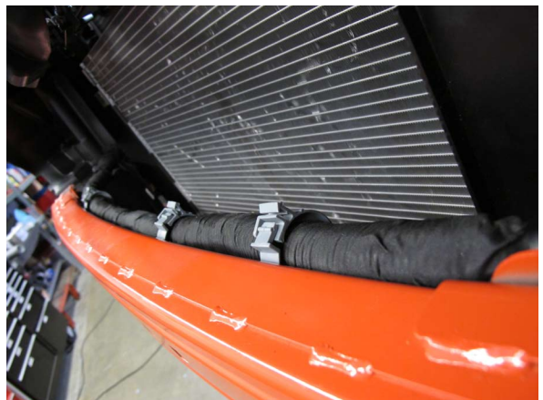
Fig. 1-i: Detach Wire Harness
