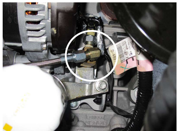
Fig. 11-f: Oil Feed Assembly Orientation
