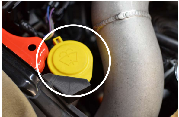
Fig. 5-g: Windshield Reservoir Clearance
