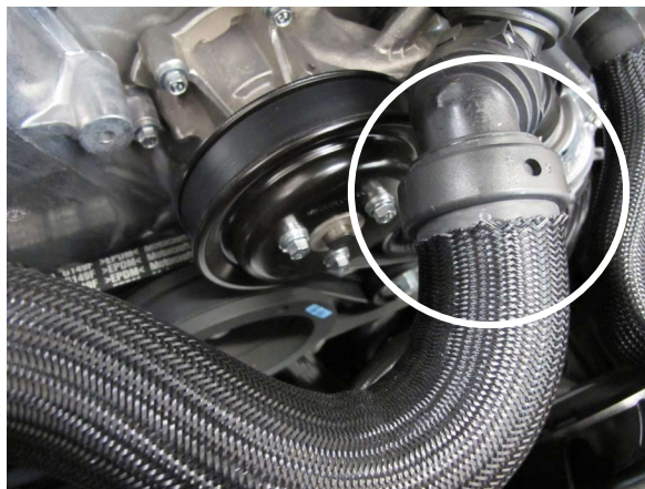
Fig. 7-b: Cut Plastic Hose Clamp
