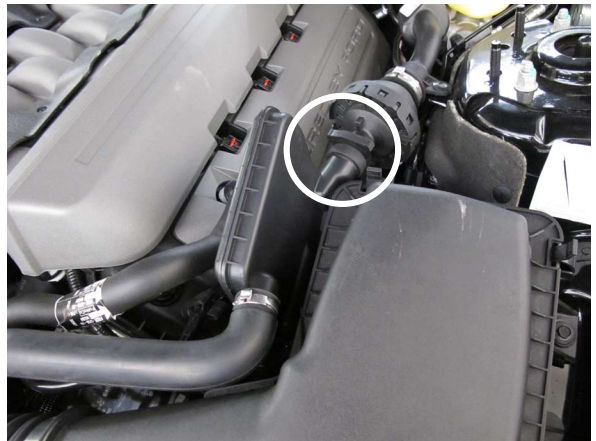
Fig. 1-n: Remove Interior Sound Tube
