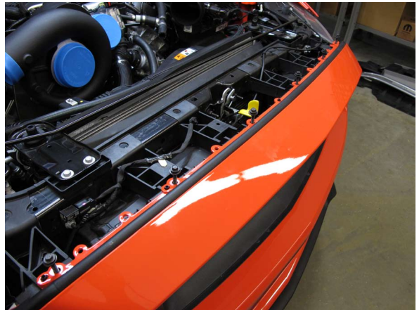
Fig. 1-b: Remove Bumper Cover Fasteners
