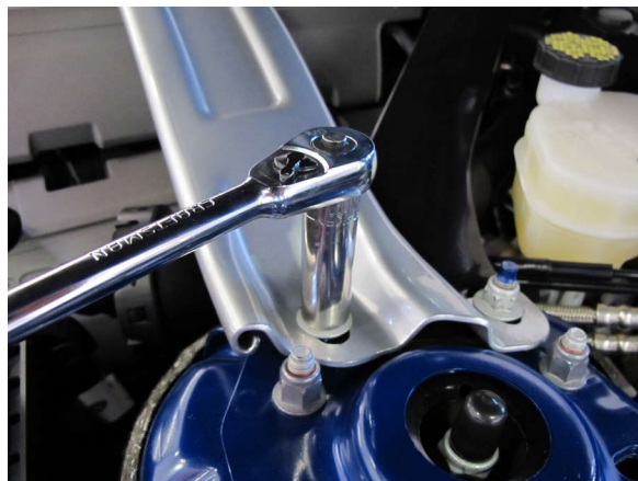
Fig. 2-d: Remove Strut Tower Brace
