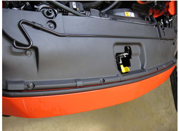
Fig. 1-a: Remove Plastic Cover
