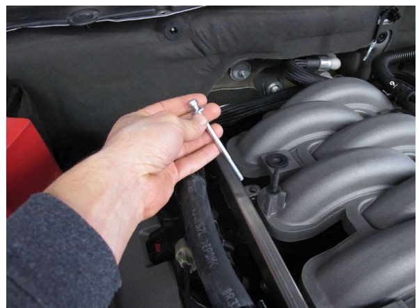
Fig. 6-f: Re-securing Fuel Rails
