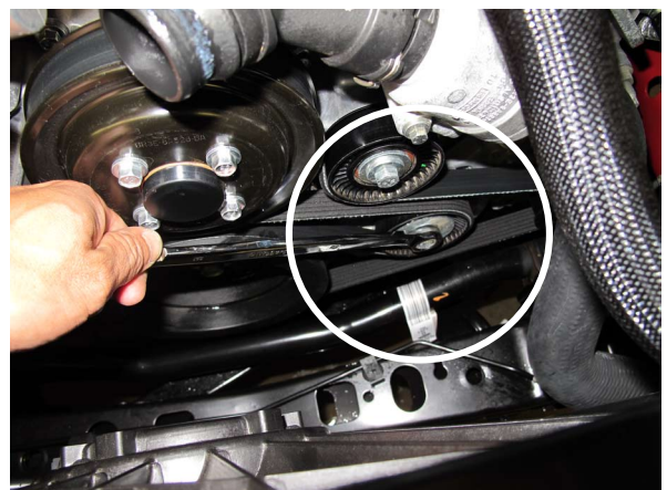
Fig. 1-r: Remove Accessory Drive Belt
