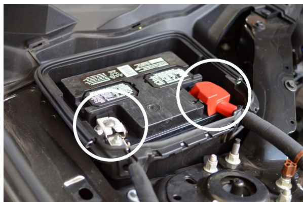
Fig. 2-e: Unplug Battery Leads
