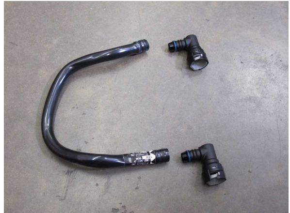
Fig. 4-a: OEM Passenger Side PCV Hose (Fittings Removed)
