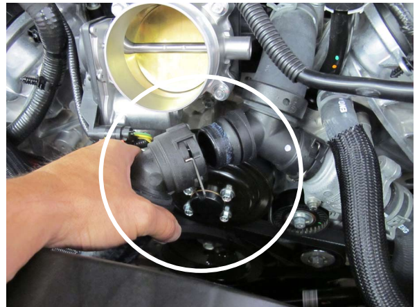
Fig. 1-q: Remove Upper Radiator Hose
