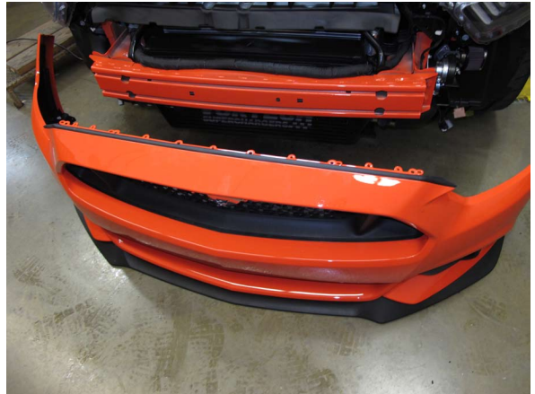
Fig. 1-h: Remove Front Bumper Cover
