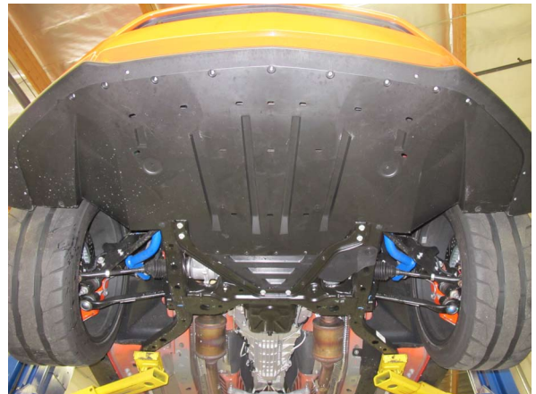
Fig. 1-e: Remove Front Undertray
