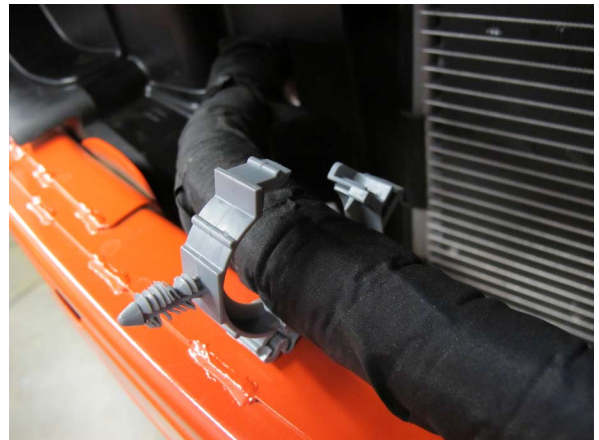
Fig. 1-j: Remove Gray Wire Harness Clips
