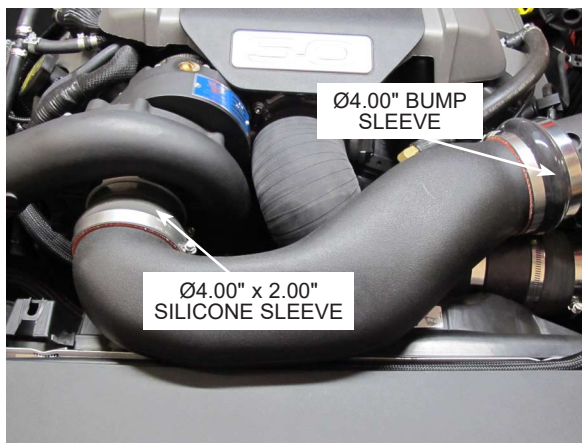
Fig. 8-b: Attach Air Inlet Duct To Air Box
