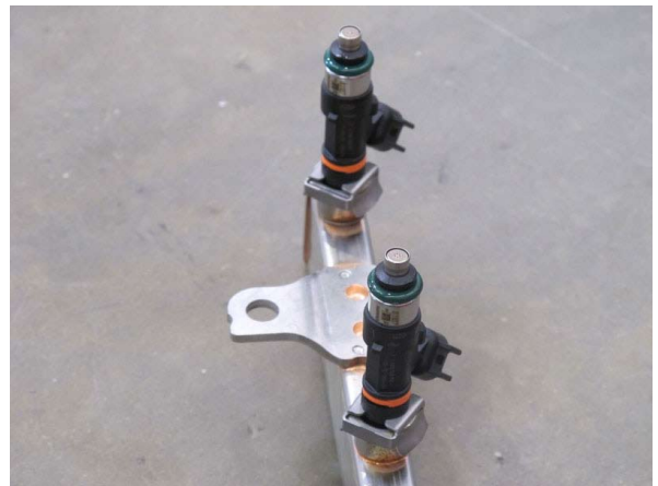
Fig. 6-e: Fuel Rail / Injector Assembly Detail
