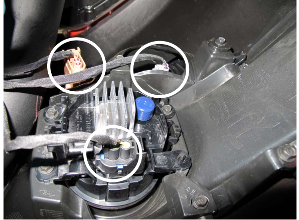
Fig. 1-g: Unplug Fog Light Connectors
