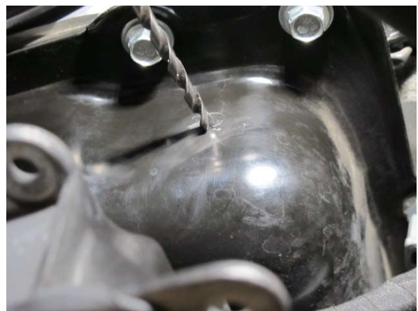
Fig. 12-c: Drill Pilot Hole
