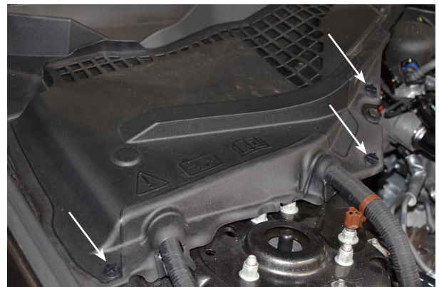
Fig. 2-c: Remove Battery Cover
