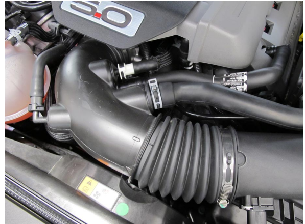
Fig. 1-m: Remove Intake Tube
