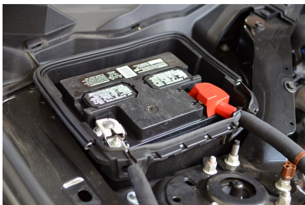
Fig. 2-d: Unplug Battery Leads
