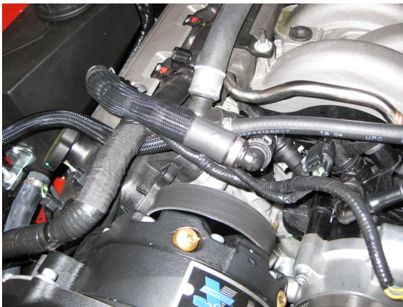
Fig. 4-d: Modified Passenger Side PCV Hose, Installed
