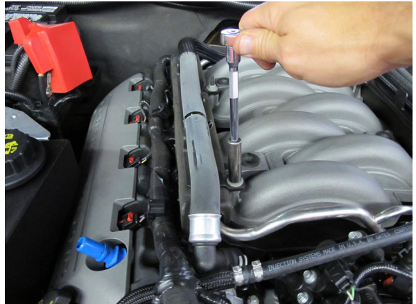
Fig. 6-b: Hose Guide Removal
