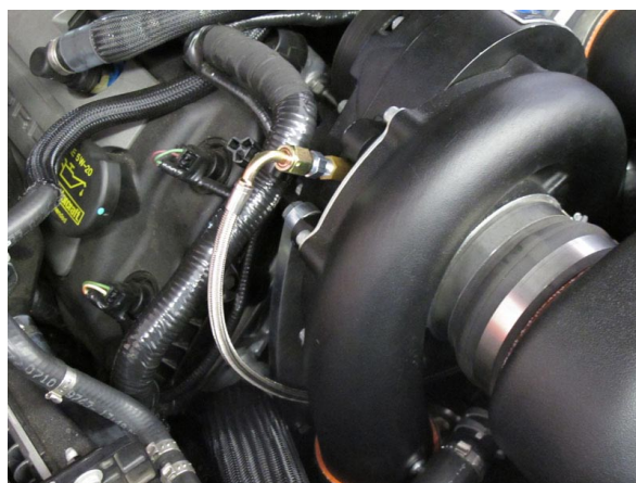
Fig. 11-c: 90° Oil Feed Hose Installed
