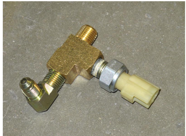
Fig. 11-h: Oil Feed Assembly (shown removed for clarity)
