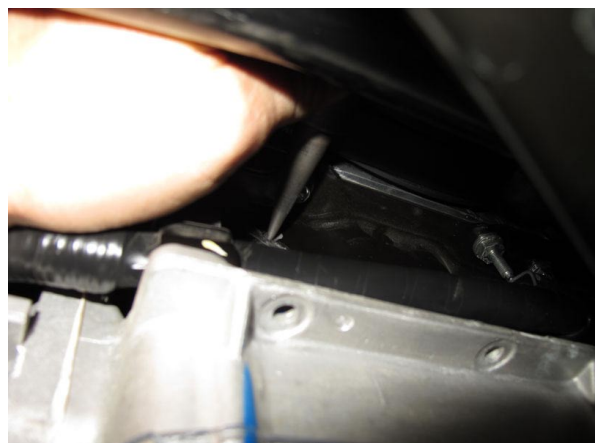
Fig. 12-d: Punching Hole in Oil Pan
