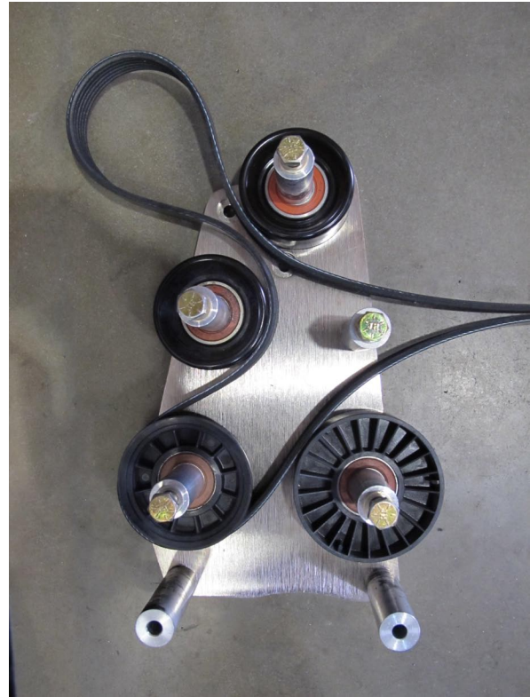
Fig. 3-c: Belt Routing (front plate removed for clarity)
