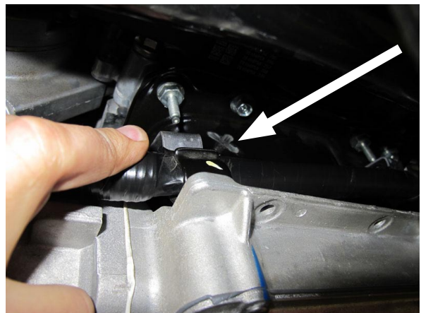
Fig. 12-b: Oil Drain Fitting Installation Location
