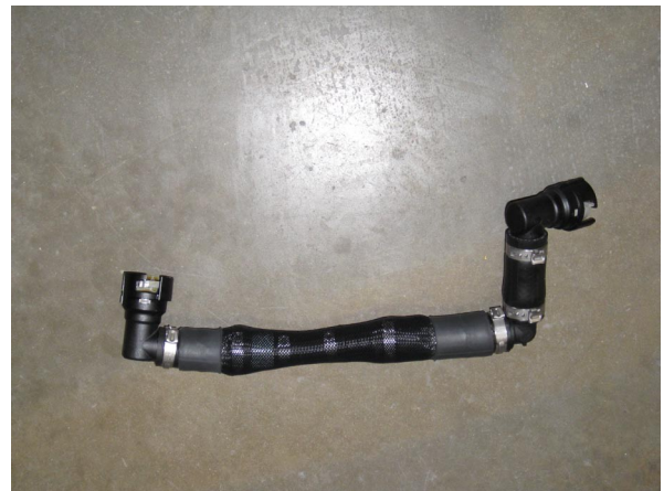
Fig. 4-c: Modified Passenger Side PCV Hose
