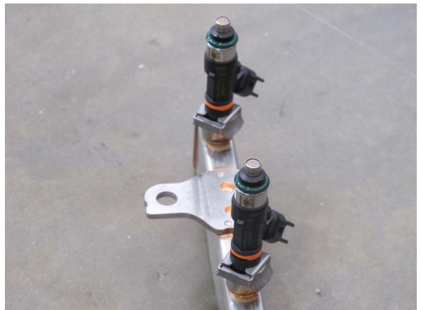
Fig. 6-k: Fuel Rail / Injector Assembly Detail
