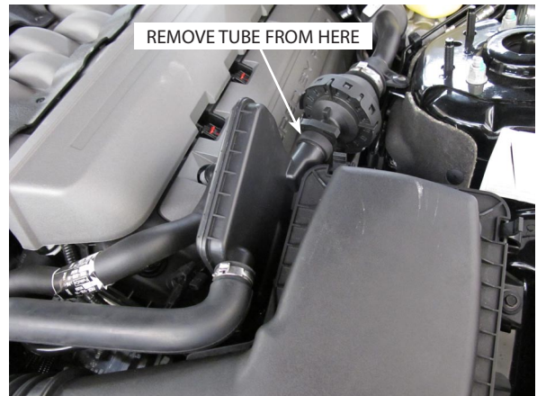
Fig. 1-n: Remove Interior Sound Tube
