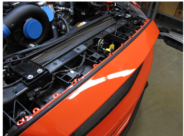
Fig. 1-b: Remove Bumper Cover Fasteners
