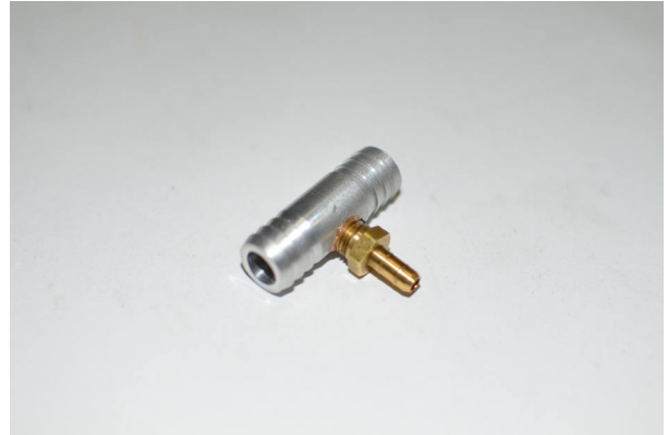
Fig. 9-a: Vacuum Tee Installation
