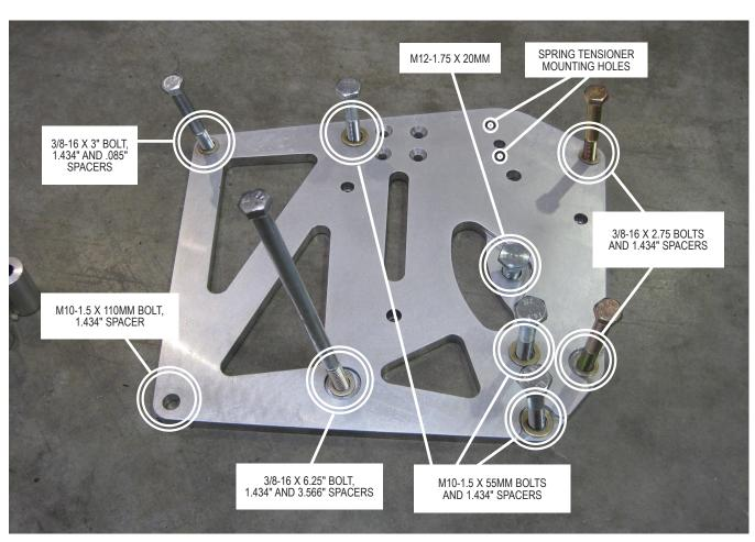
Q. Tighten all fasteners with the exception of the M10-1.5 x
