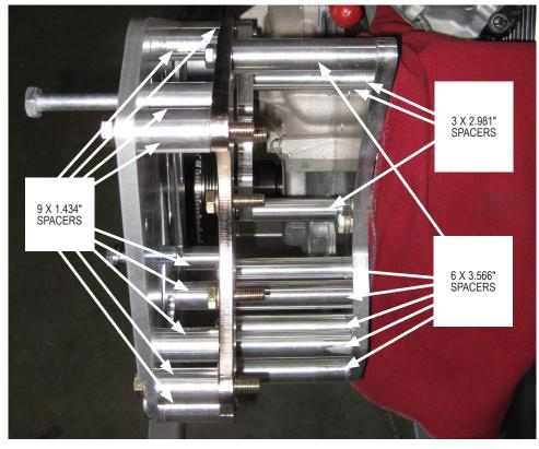
P. Remove the one (1) 3/8-16 x 3" and one (1) 3/8-16 x 6.25" screw previously loosely installed. Take care not to lose the .085" spacer sandwiched between the steel plate and the aluminum P/S bracket in the location of the 3" screw. Install the front tensioner support plate using all of the hardware and spacers in the previous step. Reinstall the one (1) 3/8-16 x 3" and one (1) 3/8-16 x 6.25" screw, again taking care not to lose the .085" spacer.
