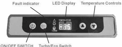
ON/OFF SWITCH Turbo/Eco Switch
