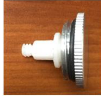
NG Position: Plastic Ring is next to the Cap
