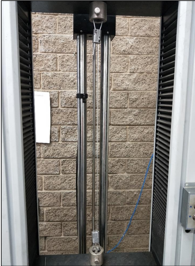
Figure 5: Without lock 1 mounted in the UTM before test
