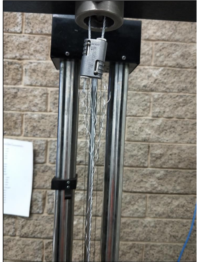
Figure 6: Without lock 1 failure location
