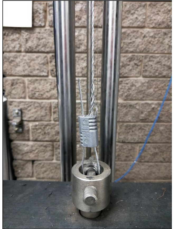
Figure 2: With lock 1 failure location
