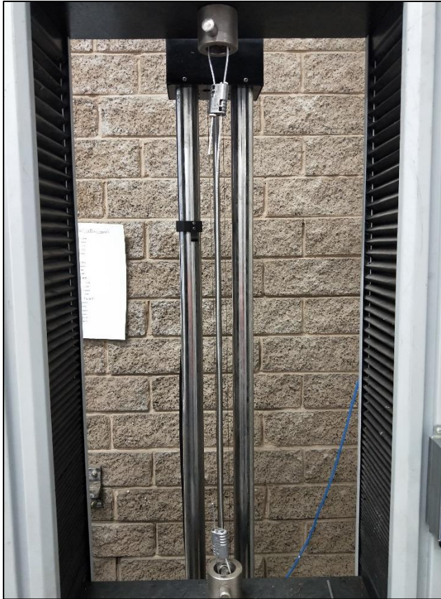
Figure 1: With lock 1 mounted in the UTM before test
