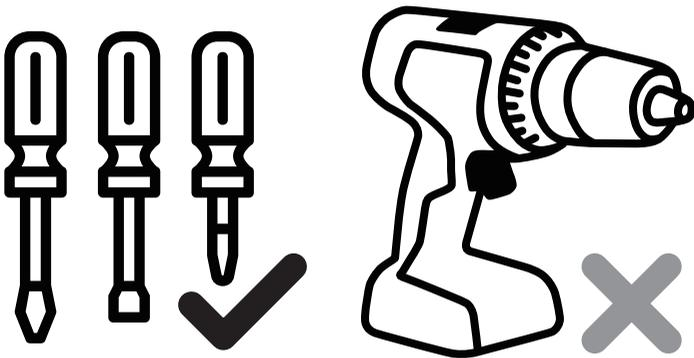
Using an electric drill can cause irreversible **damage to the MDF boards**, leading to compromised structural integrity and potential voiding of your warranty.
