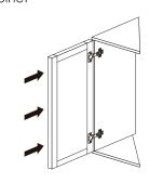
Rotate the "front and rear screws" to the right
