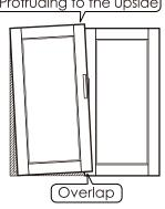
Turn "internal & external screw" to the left can make the bottom of the door tilted outward.
