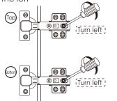
After adjusting the "front and rear screw", the door still does not change, please turn the "internal & external screw" to the right Slightly.
