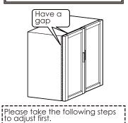
Rotate the "front and rear screws" to the left
