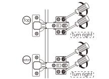
$\divideontimes$  If the door is lower on bottom, please lift up the left door slightly on step 2
