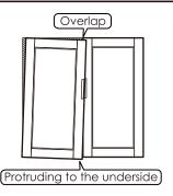
Turn "internal & external screw" to the left can make the top of the door tilted outward.
