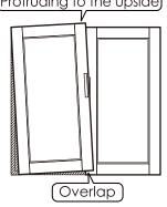
Turn "internal & external screw" to the left can make the bottom of the door tilted outward.
