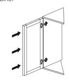
Rotate the "front and rear screws" to the right Turn right!
