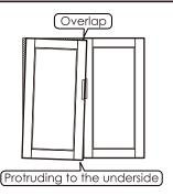
Turn "internal & external screw" to the left can make the top of the door tilted outward.
