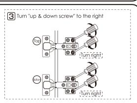
$\divideontimes$  If the door is lower on bottom, please lift up the left door slightly on step 2
