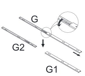
Flip the switch to separate G into G1G2
