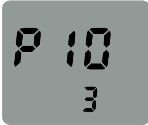
Start power strength setting interface
