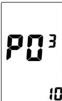
Automatic shutdown time setting interface
