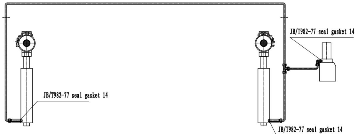
Diagram of hydraulic line of floor-plate 2-post lift
