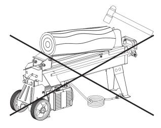
Do not try to knock the jammed log off. Knocking about will damage the machine or may launch the log and cause accident.
