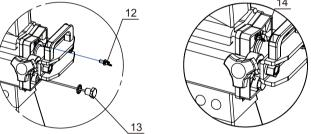
Before operating the log splitter, the Bleed Screw should be loosened by some rotations until air can go in and out of the oil tank smoothly.
