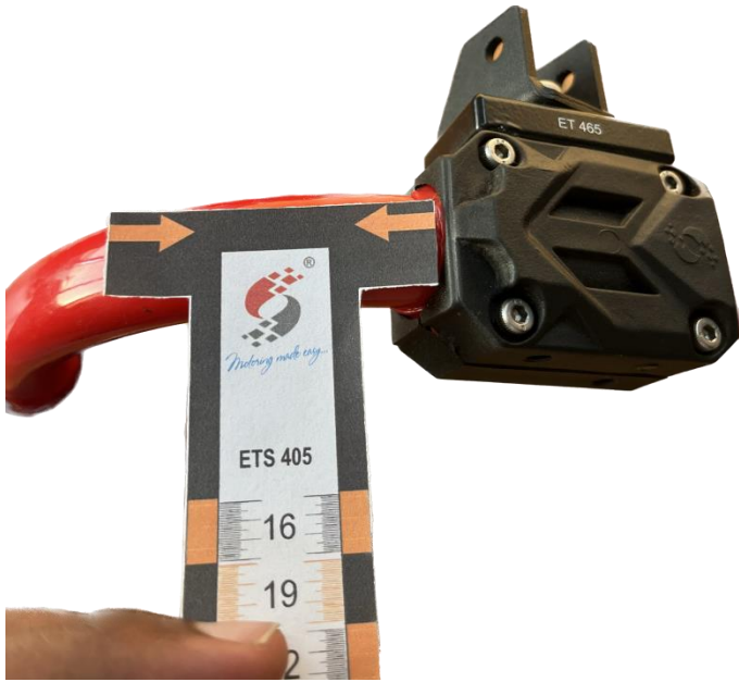
Measuring Tape used on bent pipe surface
