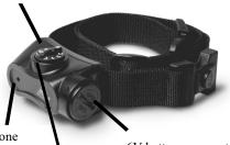
Turning the unit ON To turn on the unit, turn the dial from the off position to one of the levels (shown on the dial from 1-8 as well as a "T" for TONE ON-LY) You will hear a series of quick beeps. The LED indicator light will flash to indicate power is on.
