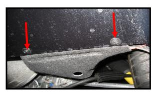
You can remove this panel if you need more access to feed the wires up to the side markers. Remove 2 #15 torx screws.
