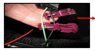
Using the supplied connectors place 1 wire in each metal clip and fold the connector closed until it clicks shut. You may need to use pliers. Wire colors are: drivers side: purple is positive. Black is negative Passenger side: brown is positive, black in negative.
