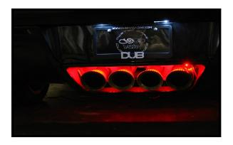
Turn on the lights and be sure leds are working. Use black electrical tape to re-tape the harness. Tie up the led wires to keep away from the exhaust. Reverse procedures to reinstall any panels removed.
