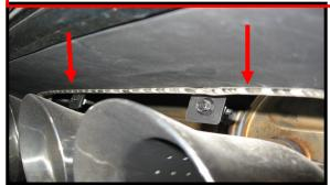
This shows where to mount the led strip. You may want to do the wiring before mounting the strip. Clean this area with the alcohol pad and led dry. Apply adhesion promoter, let dry. Center the led strip, remove backing and apply strip. Press in place for a minute.
