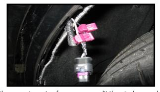
Pull the connector out as far as you can, split the wire loom and separate the wire to install the connectors. Route the led wires up to the connectors. This is where a straightened coat comes in handy. Tape the wire to the coat hangar and pull through.
