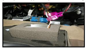
Now plug in the led wires to the connectors. Red to orange and black to white as shown. The led wires just plug into the back of the connectors. Use force to make sure they are tight
