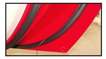
The weather strip is held by small push in pins. You can release them with a forked tool. Route the wires behind the weather strip down towards the bottom of the door where the leds will be mounted.
