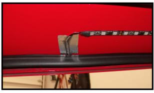
This shows how to mount and hide the wires. Use strong tape to secure the wire as illustrated.
