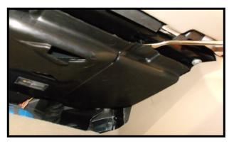
Remove the passenger side panel above the foot well. You should be able to do the drivers side without taking this panel off.
