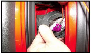
Un tape the wires. With one hand feed the wires through the boot, put the other hand in the opening of the inside upper panel you unsnapped and pull the wires through.
