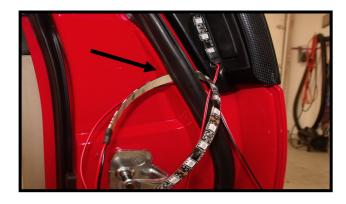
Open the door and lift the weather strip up a little so you can pass the short door handle strip under it. (arrow).
