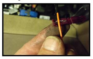
You can now tap into the orange and white wires coming from the footwell lights. Place each wire in the metal V of the supplied connectors and snap shut using a pair of pliers.
