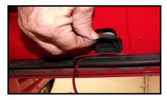
Remove the rubber plug at the front bottom of the door. Now move to inside the car.
