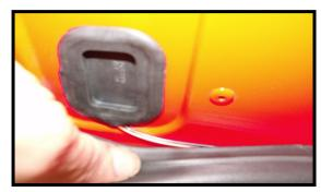
Now replace all boots. You can dab a little silicone on this boot to assure its sealed. Test the lights by turning on the key or opening the doors.
