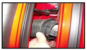
At the front of the door you will find this rubber boot. Pull it out of the front of the door so you can pass the led wires through it after you feed the wires through the door.
