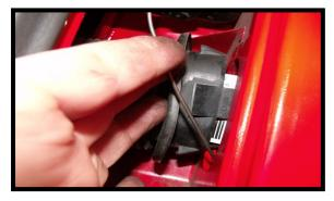
This shows the feed wire coming out of the boot. Pull the wires through the door.
