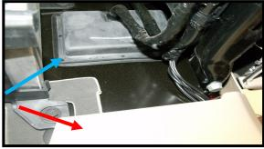
Blue arrow points to the panel you need to remove. Its located above the side kick panels on each side of the foot wells. (red arrow) Just grab the wire harness and pull, it pops out easily. Now move to the front of the door.
