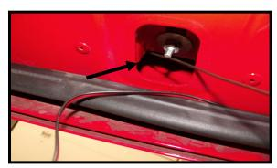
Now straighten a coat hangar or equivalent and tape the end of the led wires to the end tightly. Feed the hangar behind the brace (arrow) towards the boot you just removed at the front of the door.
