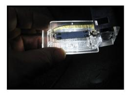
Un-hook the 2 wire loops from the end on the factory bulbs. (careful, they may still be hot). Remove the bulbs. Install the new led bulbs and test. Led bulbs are polarity sensitive so if they don't light, swap ends and re-test. Be sure to face the leds toward the clear lens and not toward the metal shield. Make sure interior lights havent timed out which they may do after about 15 minutes.
