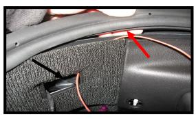
Pull up on the weather strip (red arrow) and pass the led wires through the opening ( black arrow).
