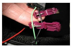
This illustrates how to use the connectors. Your wire colors will be different. (see next text box). Place the wires in the metal V and close with pliers until they latch.
