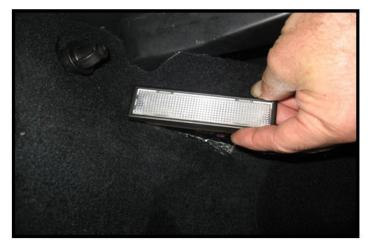
Pull the hatch/trunk light housing from the carpet to gain access to the back of the housing.
