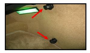
You can tap into the wires on either side. Decide which side you want to tap into and remove these 2 plastic cargo net nuts, remove the light housing to gain access to the wires.
