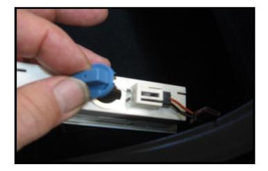
Turn the bulb socket 1/4 turn counterclockwise to remove it. Pull the factory bulb out and insert the led. Replace the socket and lock it in place. If the led doesn't light remove the socket and turn it 180 degrees and re-insert it. It should now light. The lights will time out after about 15 minutes so keep that in mind if it doesn't light. Push the housing back into the carpet and repeat procedure on the other side.
