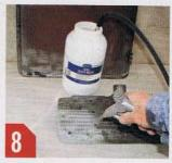
8) Soda blast media is ideal for more delicate work, such as removing paint without using chemicals and without damaging metal-especially very old metal, such as this Navarro head.
