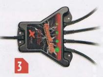
The QuadLink is one of the better ideas to come along for the home shop where multiple batteries (up to four) need to be maintained. Compatible with all chargers that use the standard twopin power output connector.
