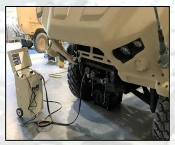
• When this happens on a JLTV we recommend lowering the battery tray for access to test and charge the batteries. Continued next page.
