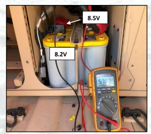
NOTE: Alternate chargers for JLTV Pri or AUX batteries would be the Pallet, Pro-PC-6, Pro-PC-12, or SC-2. These are small clamp 12V chargers where individual batteries would need to be charged with no need to remove batteries (except dropping the tray for the primary) or disconnect cables.
