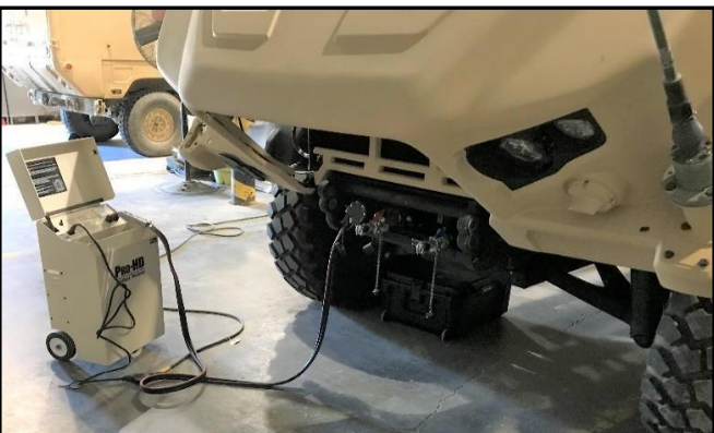
Example: Pro-HD Charger servicing the primary batteries on a JLTV.
