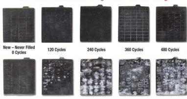
12-Volt Lead-Acid Batteries Charged with Typical Charger
