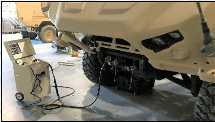
Pro-HD being used to charge the primary batteries on a JLTV.
