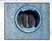
Low electrolyte level, top of battery plates are dry.
