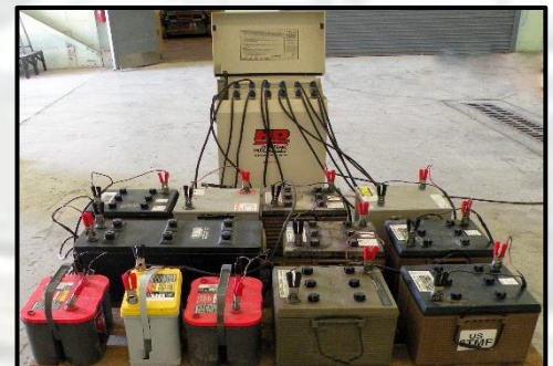
Example: Pallet Charger engaging 12 batteries of various types simultaneously.
