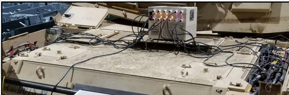
Example: BenchTop 12 station charger engaging 12 batteries simultaneously, while still mounted on M1 Tank.
