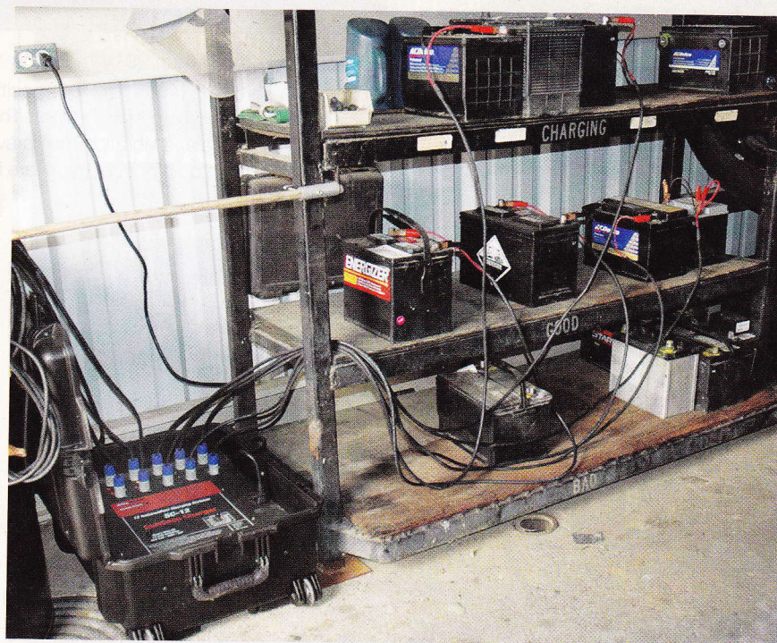
North Richland Hills, Texas, Fleet Services recharges up to 12 batteries at a time using PulseTech Products' SC-12 multiple battery charger (bottom left). Photo: Steve Noyes
